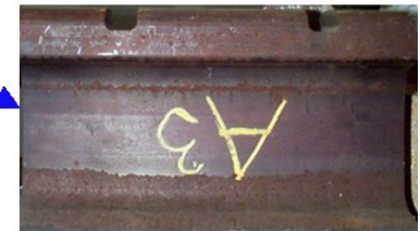
Parent pearlitic rail head before repair
