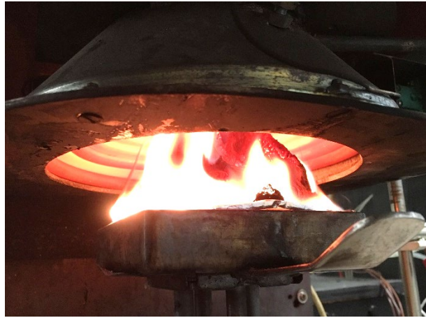
Figure 6-7. Preliminary test of Sample 1 without the retainer frame or the wire grid
