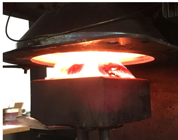
Figure 6-6. Preliminary test Sample 1 with the retainer frame and without the wire grid
