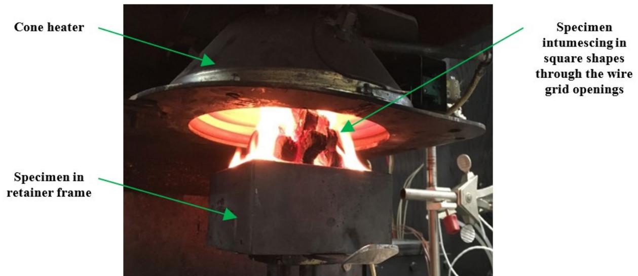
Figure 6-5. Preliminary test of Sample 1 with the retainer frame and the wire grid
