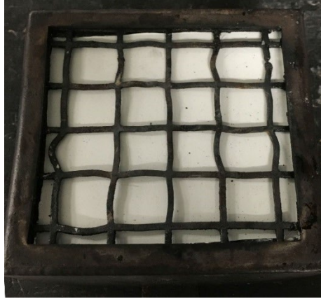
Figure 6-4. Specimen prepared with retainer frame and wire grid
