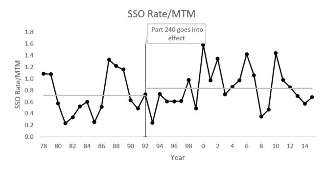
Figure 16. Comparison of SSO Rate Before and After Stop Signal Regulation Went Into Effect
