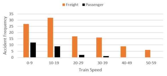
Figure 10. SSO Accident Distribution by Train Speed for Freight and Passenger Operations
