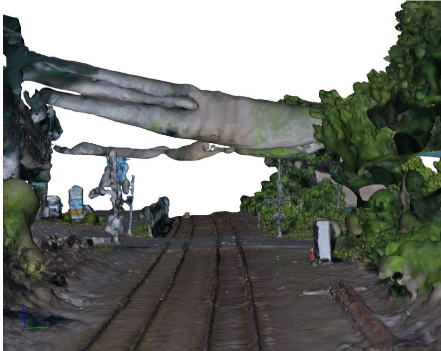
Figure 4 – Frame capture of a 3-dimensional rendering showing anomalies caused by overhead wires
