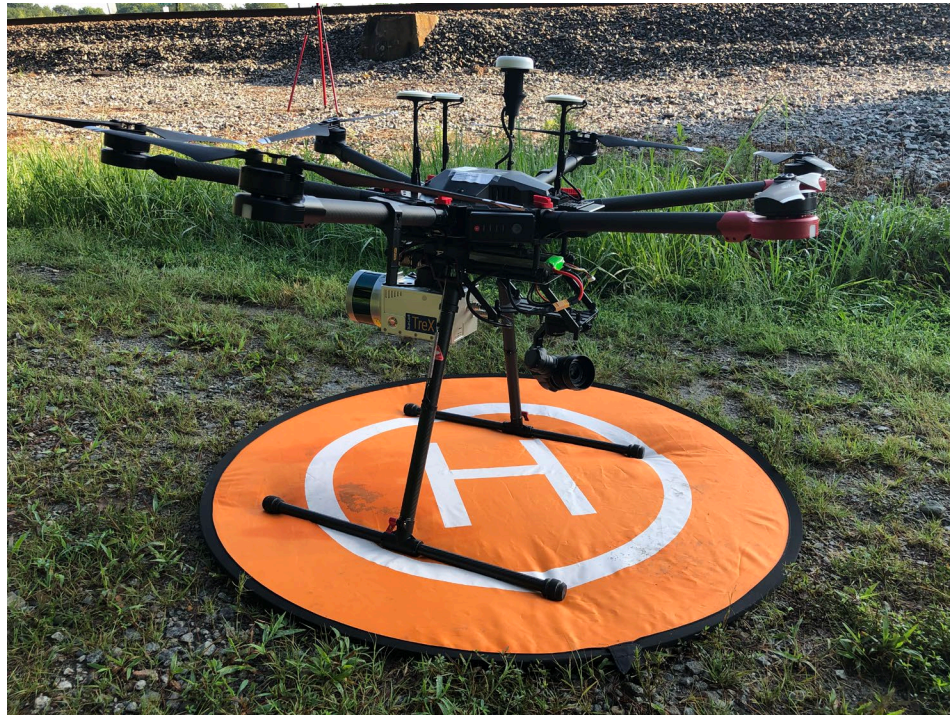
Figure 5 – DroneUp’s DJI Matrice 600 with Velodyne LiDAR system
