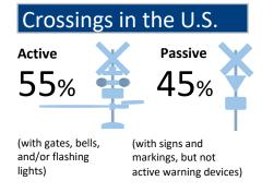
About half of the public at-grade crossings are passive and have no train-activated warning devices. Drivers must scan for oncoming trains and judge the speed and distance to determine if it is safe to cross.
