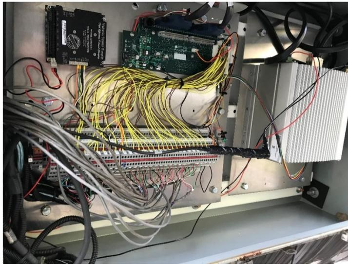
**Figure 15. Junction Box with Data Collection System Hardware**
