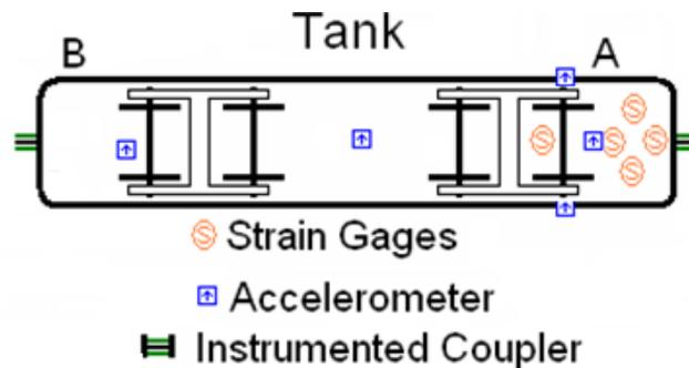
Figure 5. Schematic Diagram of Tank Car's Instrumentation
