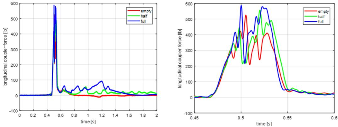
**Figure 39. Comparison of Coupling Force During Impact Empty, Half-Full and Full Tank Cars**
