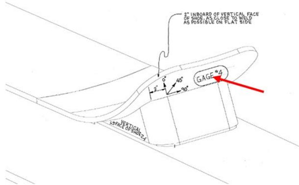
**Figure 8. Shoulder Pad Strain Gage Installed Above the Head Shoe at the A-End of the Instrumented Tank Car**
