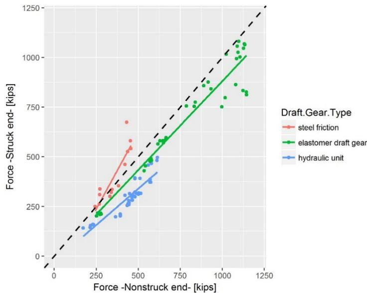
**Figure 32. Comparison of Struck and Non-Struck End Impact Force for Different Struck End Draft Gear Types and Steel Friction Gear on Non-Struck End**
