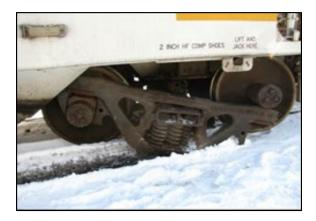
Figure 1. Broken side frame in low temperature service
