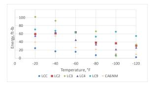
Figure 4. Charpy impact energies of the six steels
