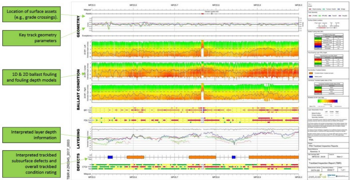
Figure E 10. One-half mile per page plots subdivided into Defects, Layering, Ballast Condition, and Geometry
