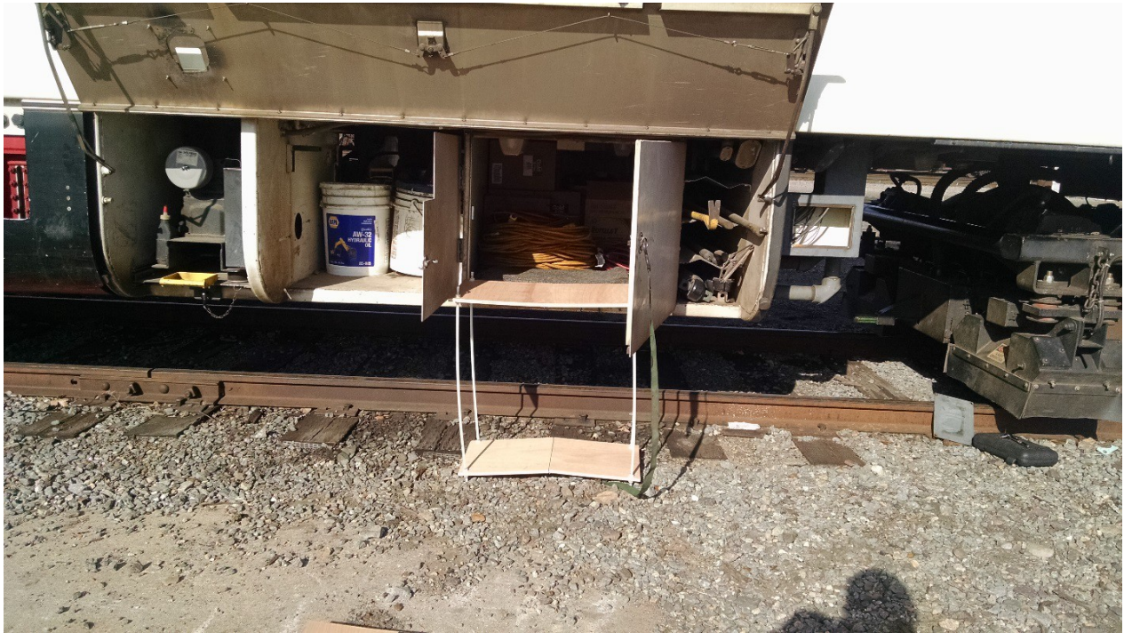
Figure A 1. DOTX220 storage compartment with plywood mockup of 2 GHz antenna
