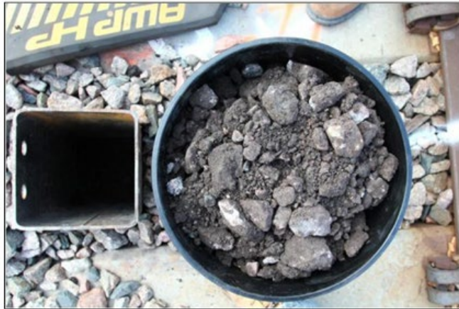
Figure E 4. Bulk ballast samples hand excavated from the sampling tubes and transferred to sealed buckets
