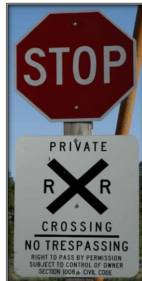
Figure 10: Stop Sign with CPUC Private Grade Crossing Sign
