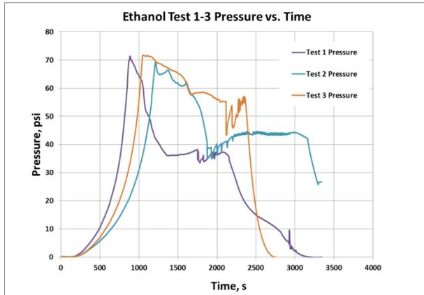
**Figure 4. Measured pressure vs. time PRD release, Tests 1-3**
