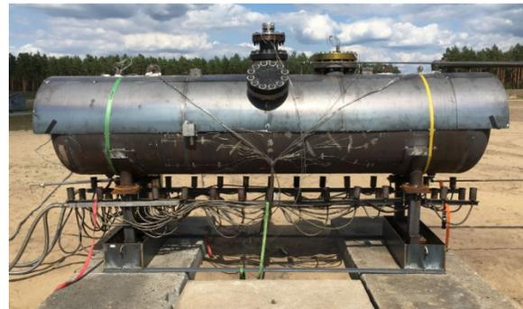
**Figure 2. Pre-test photo with steel shield and insulation for ethanol testing**
