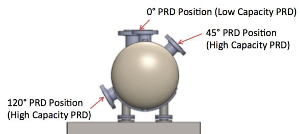
**Figure 3. End view of the tank showing PRD orientations**
