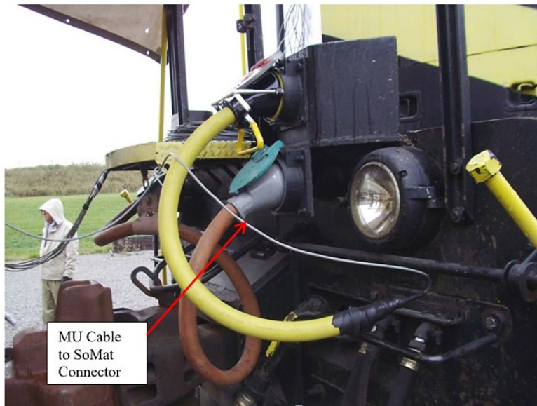
Figure 2-4. Modified MU cable (yellow) for collecting throttle position
