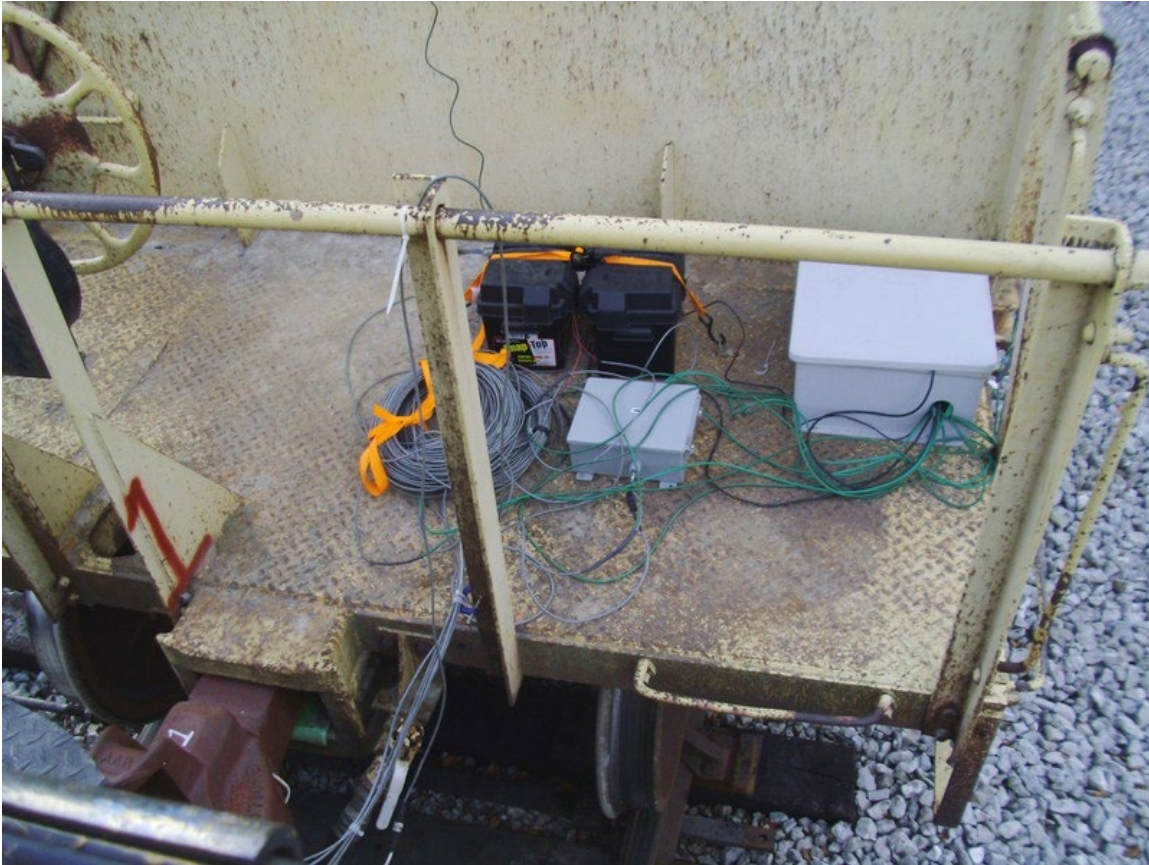
Figure 3-6. Data acquisition equipment on a typical test car
