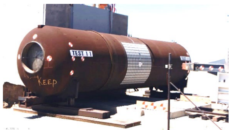
Figure 1. Pre-test Photo of DOT-113 Surrogate
