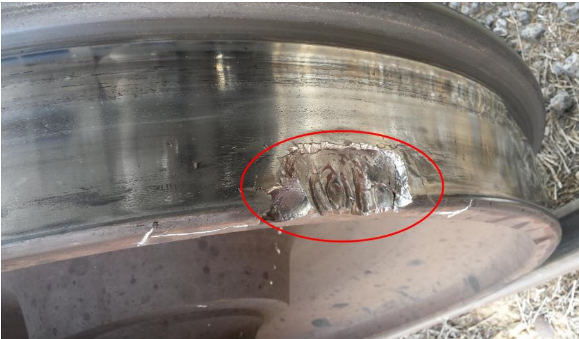
Figure 20. FAST wheel with shattered rim verified in field
