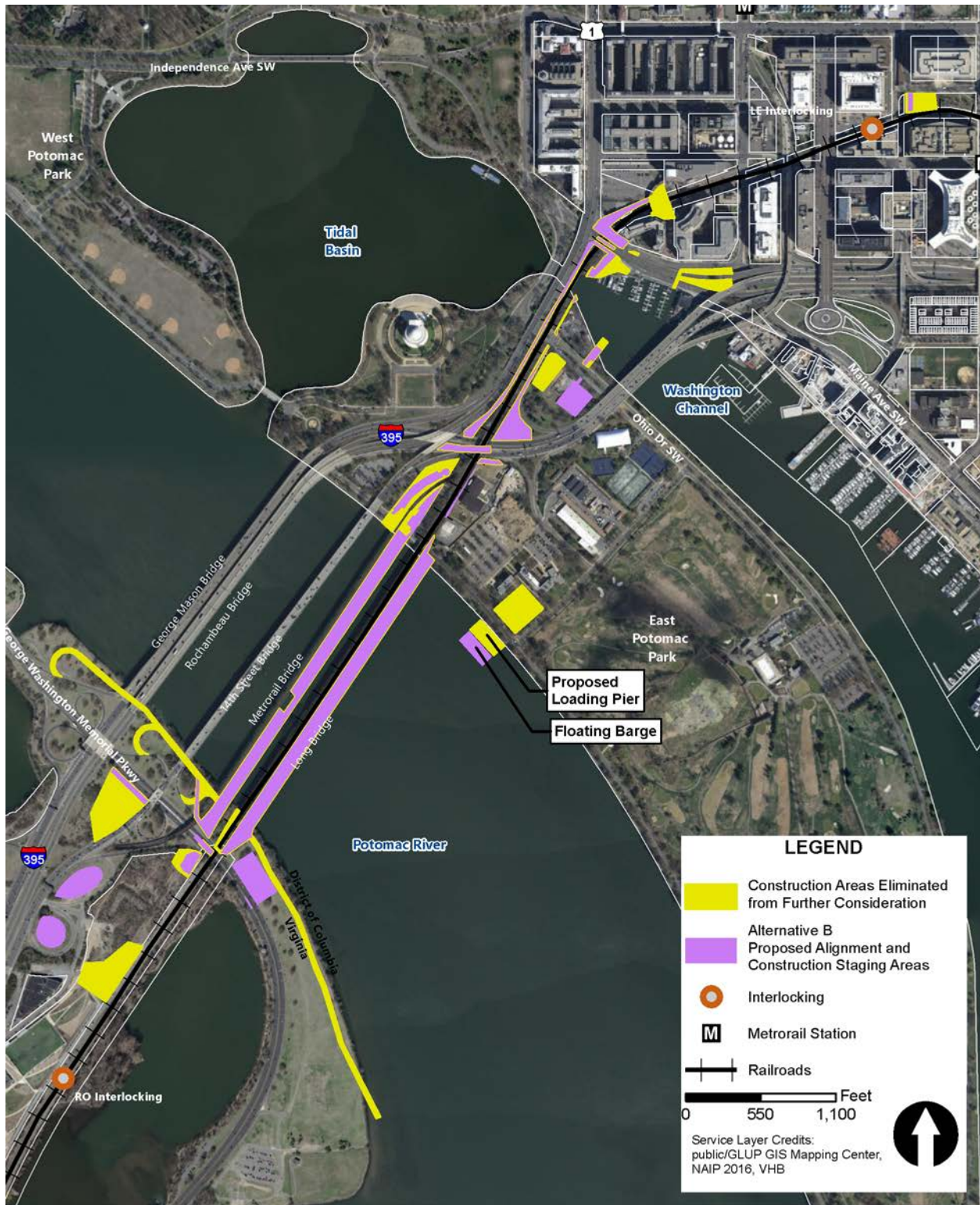
899 Figure 5-2 | Action Alternative B Minimization of Construction Impacts
