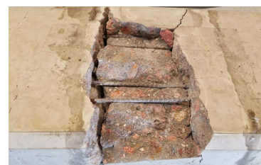
Figure 10. Crosstie with exposed wires after test
