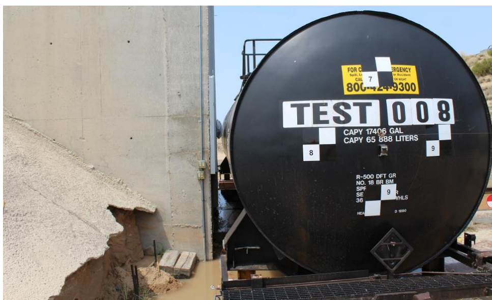
Figure 16. Tank Car—Post Impact (wall side)
