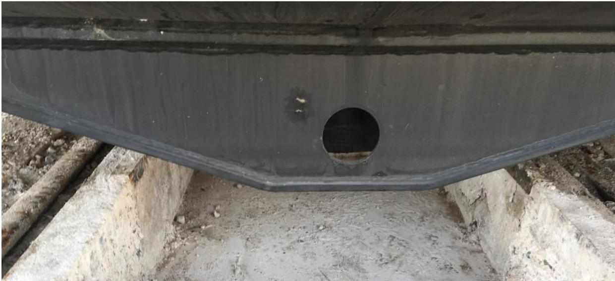
**Figure 7. Tank Car's Bottom Valve Protection Structure**
