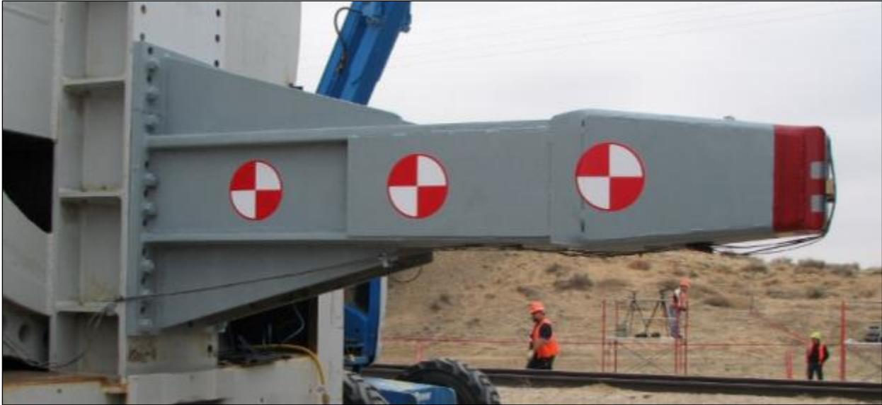
**Figure 9. Ram Arm with 12-inch by 12-inch Indenter**
