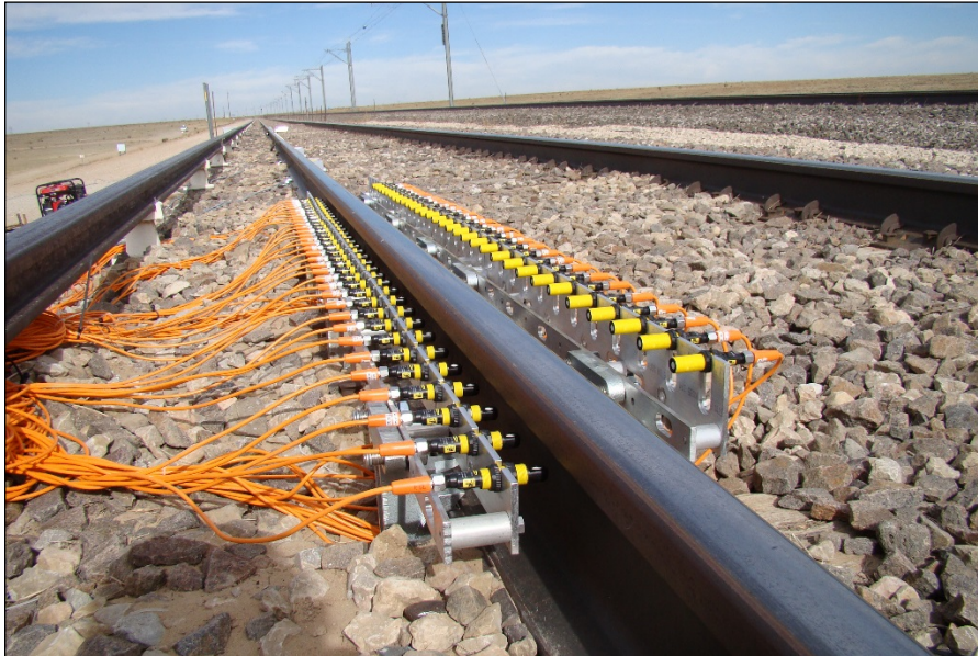
Figure 1. Broken Rim Detector Proof of Concept Prototype with Ultrasonic Sensors
