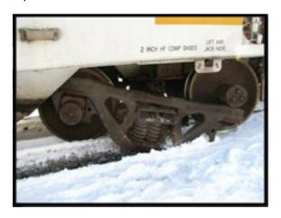
Figure 2. Broken side frame that led to derailment in winter
