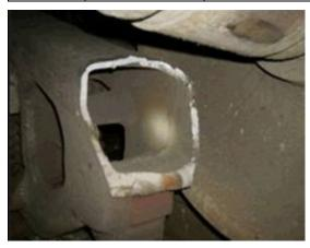
Figure 3. Fractured side frame
