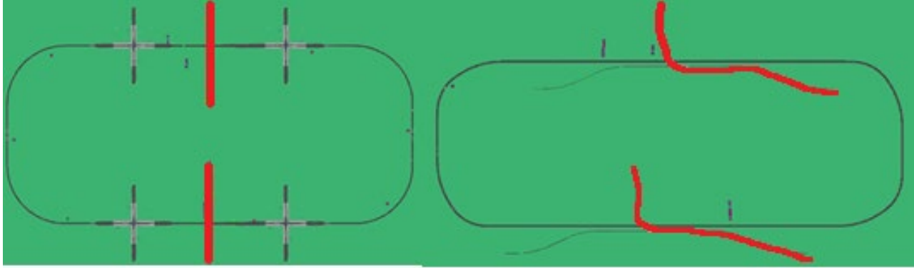
Figure 17. Track Designs for Scenario A (Left) and C (Right). Red Lines Indicate Railroads that Intersect with Highways (Gray)
