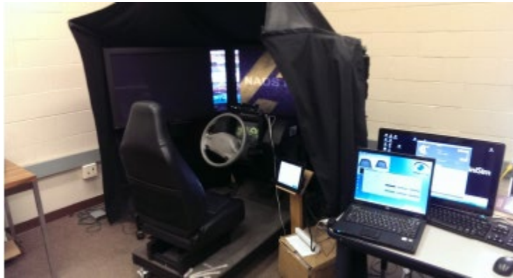
Figure 31. NADS MiniSim Driving Simulator
