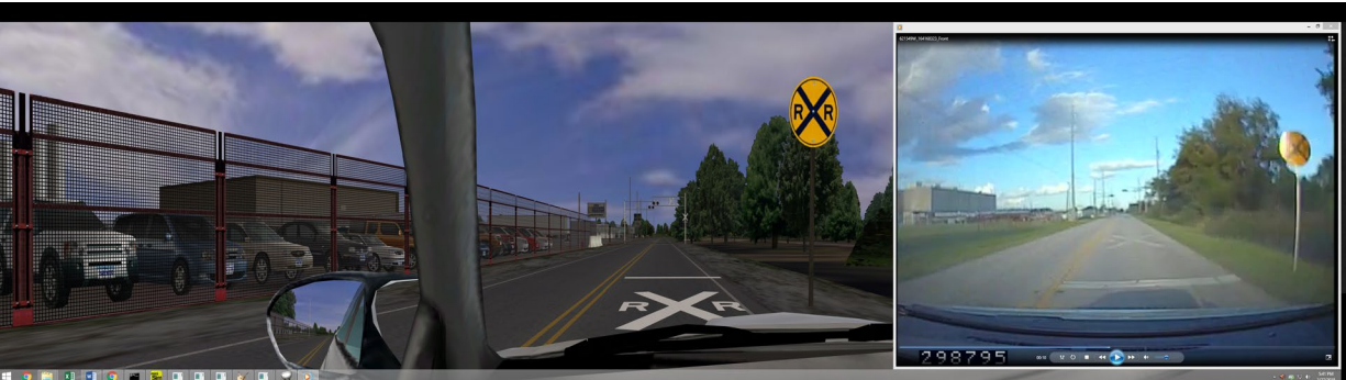
Figure 19. Simulated Advance Warning in Scenario C (Left) Compared to Reference NDS Video (Right)
