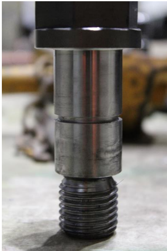
Figure 43. Intact Shear Bolt After Test
