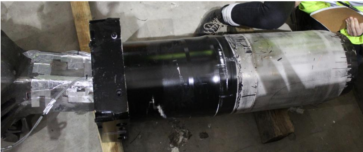
Figure 41. Activated Push-Back Coupler
