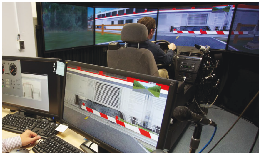
Figure 9. View of RTI Driving Simulator from Experimental Workstation
