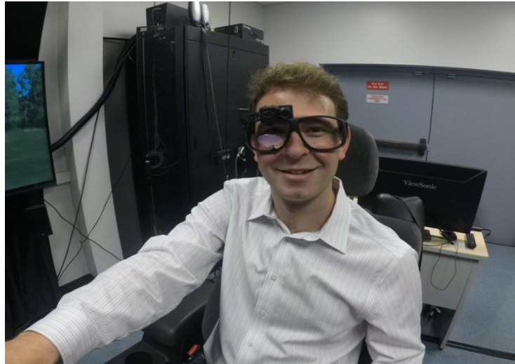
Figure 10. Head-Mounted Applied Science Laboratories Mobile Eye-XG Eye Tracker
