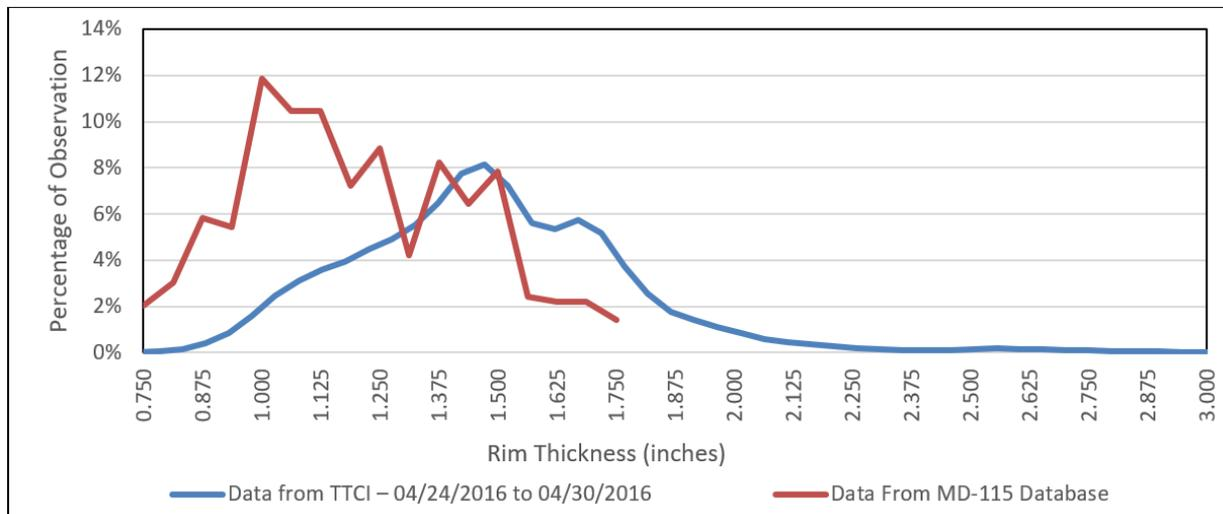
**Figure 15. Rim Thickness Values for VSR/VSF Failed Wheels (Red) Compared to the General North American Freight Population (Blue)**
