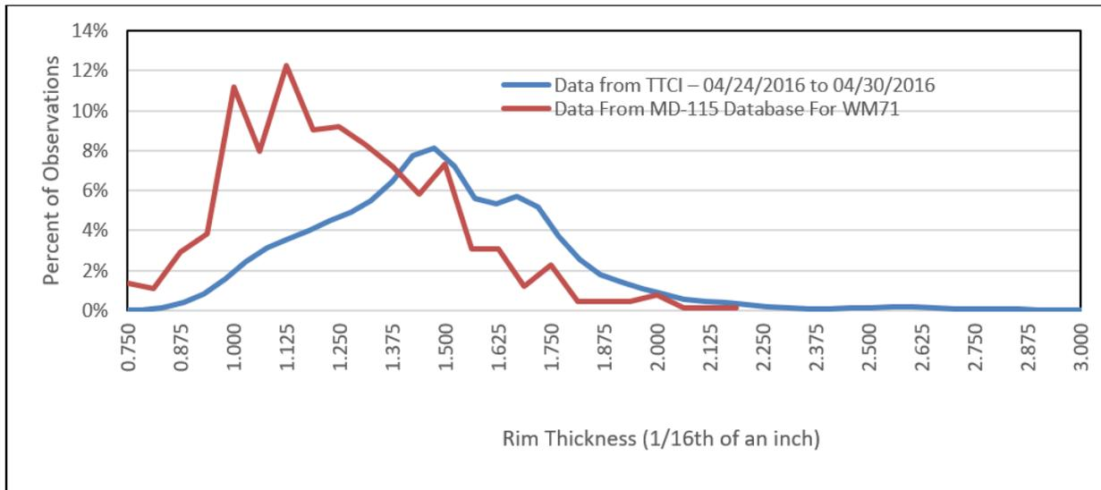
**Figure 37. Rim Thickness for Shattered Rim Wheels Compared to the General North American Freight Population**
