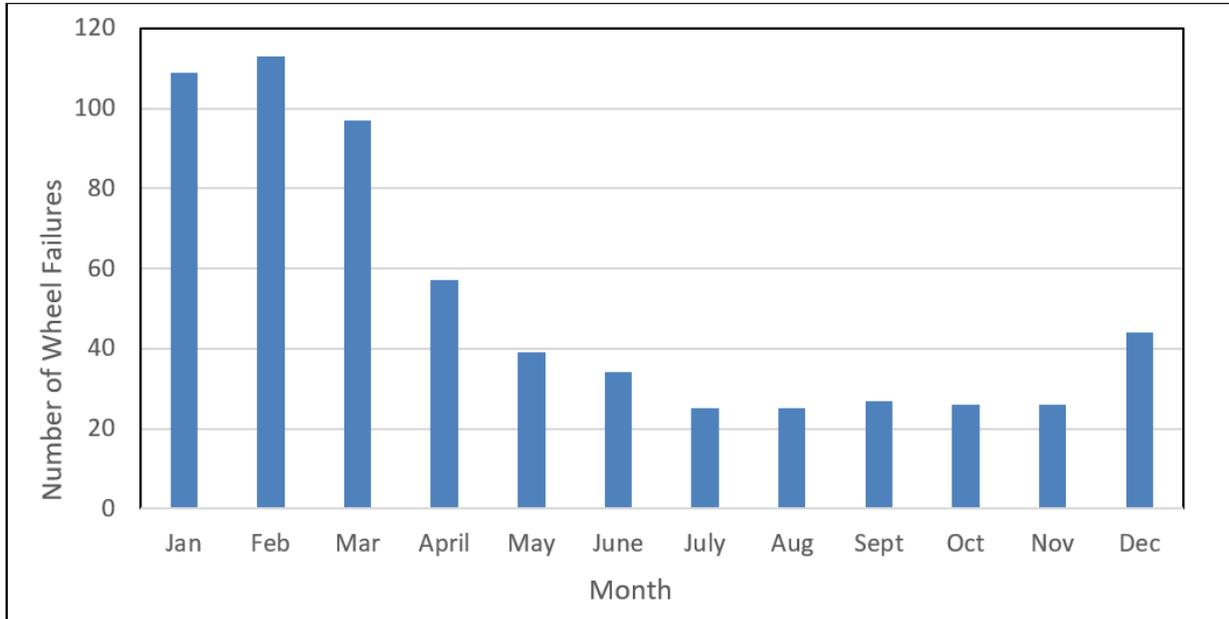
**Figure 11. VSR/VSF Failures per Month of Year**
