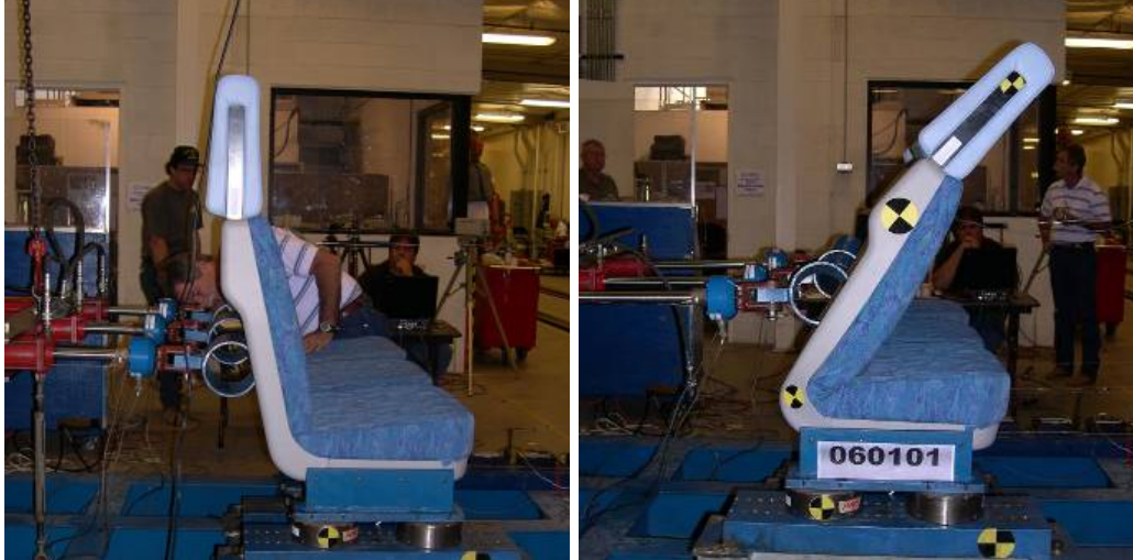
Figure 60. Pre- and post-test photographs of the FF knee load test
