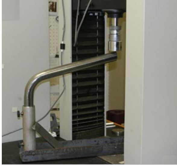
Figure 14. A pre-test photograph of A572-50 tube bending specimen inserted into the fixture and mounted on the Instron testing machine
