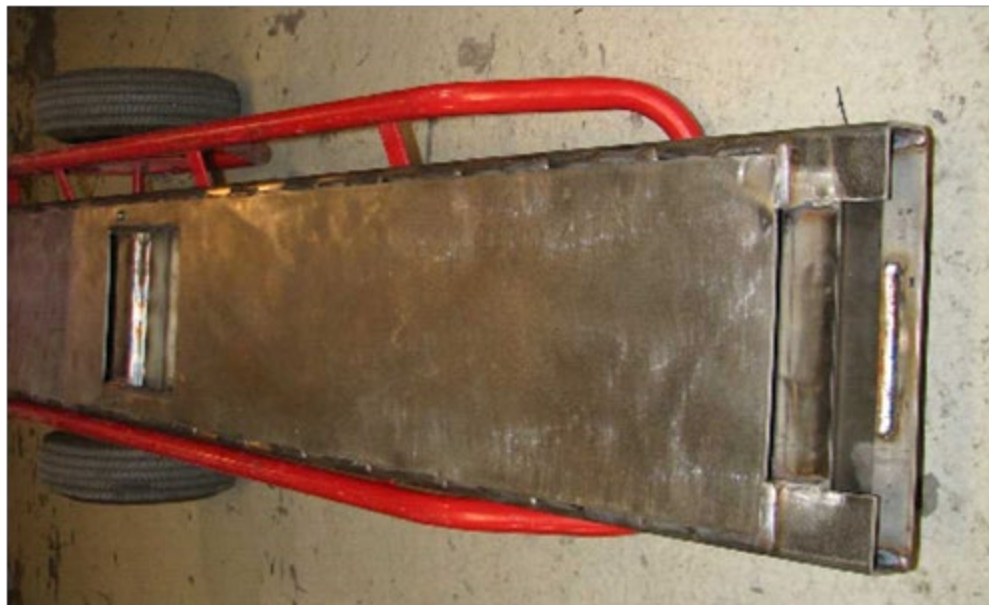
Figure 53. Seat channel with welded bottom cover plate
