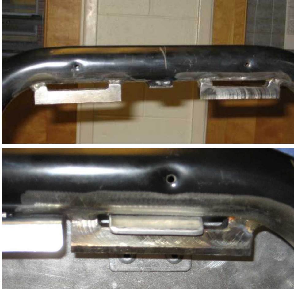
Figure 56. Two “C” brackets welded to the seat frame (top photograph). Bottom seat cushion and seat frame assembly
