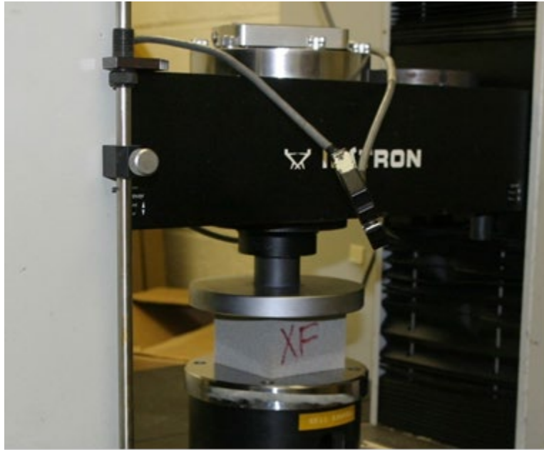
Figure 16. Test setup for headrest foam compression tests
