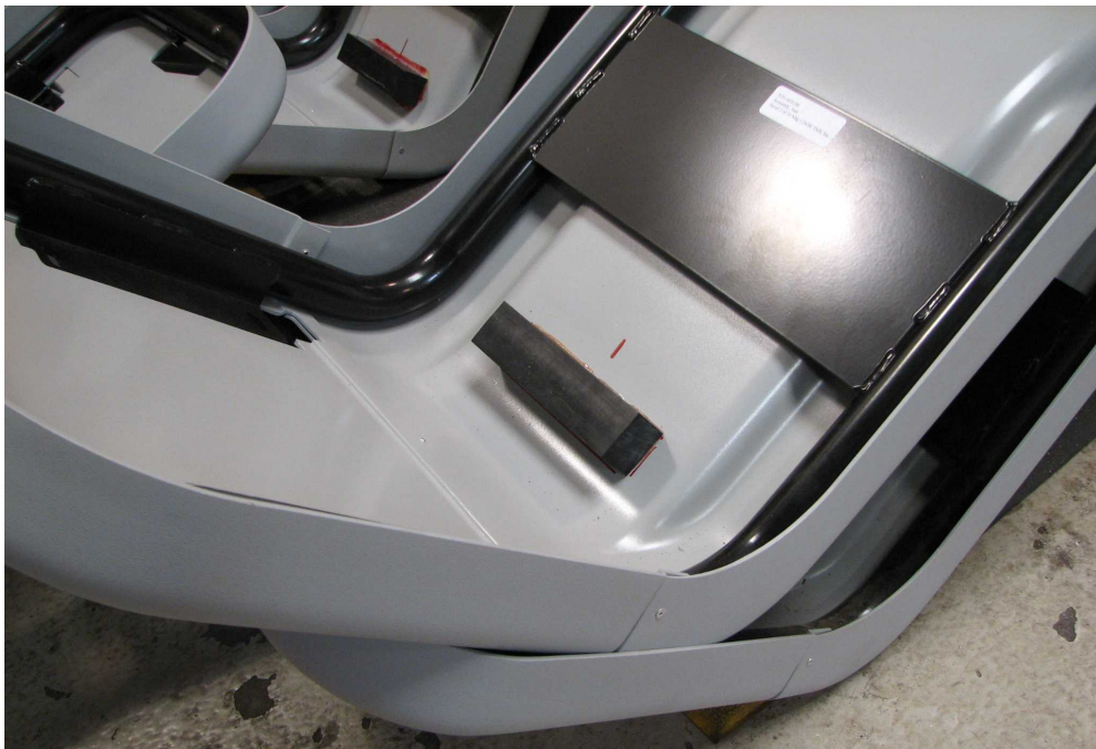
Figure 55. Rubber stop bonded to the plastic shroud
