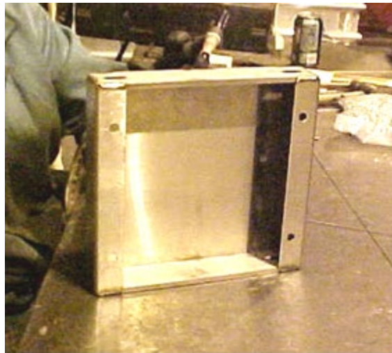
Figure 50. A photograph of the pedestal weldment
