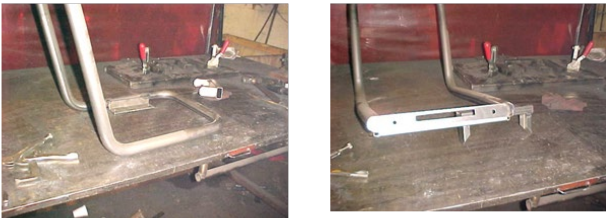
Figure 43. Seat frame welding and fixture
