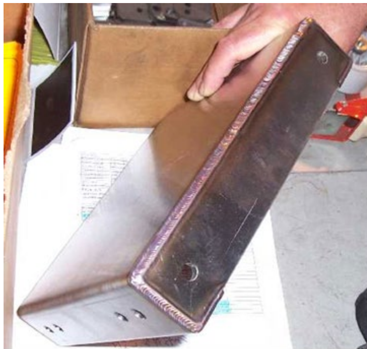
Figure 51. Revised pedestal design showing the continuous weld and the mounting holes on the side of the pedestal channel for the additional corner brackets
