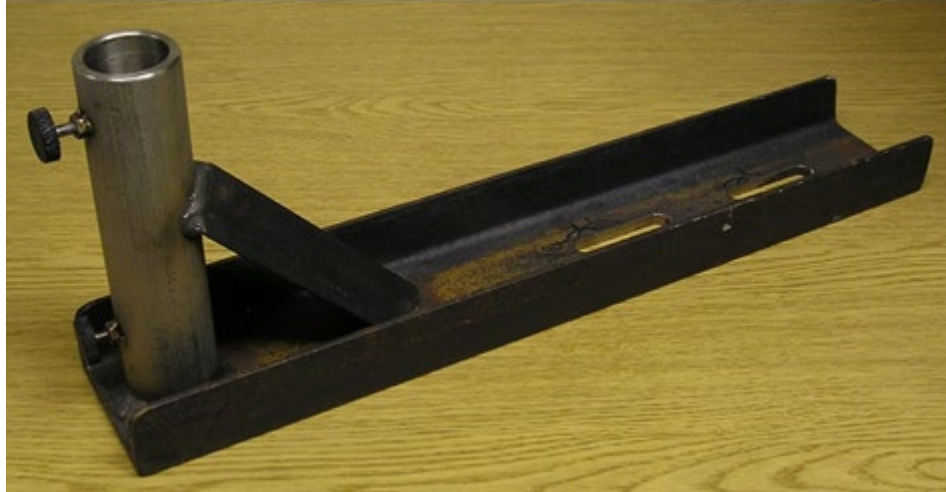
Figure 13. Fixture used to hold the tube bending test specimen
