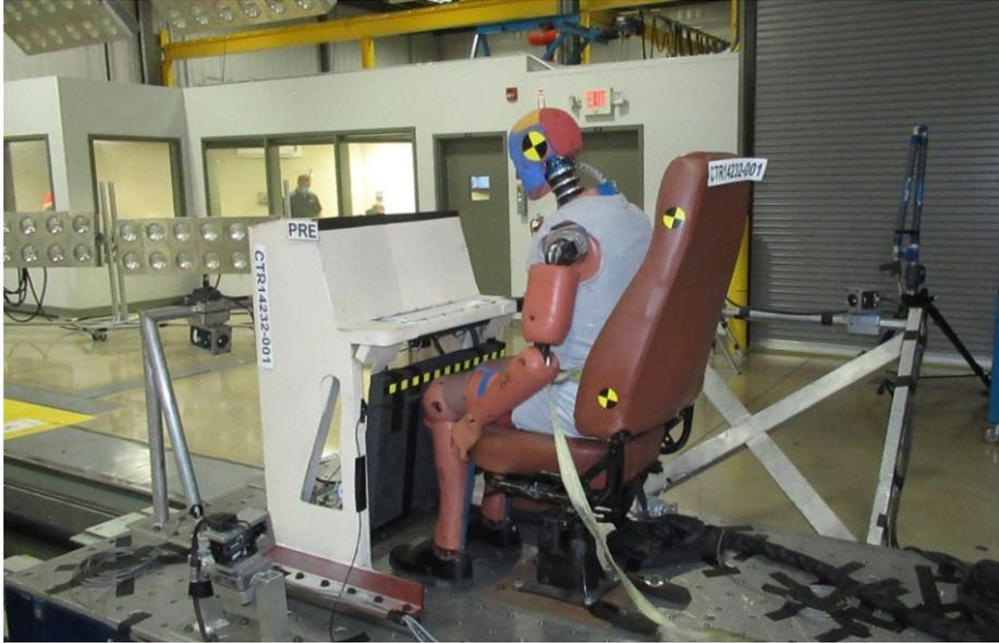
Figure 4-6. Dynamic Sled Test Setup with 95<sup>th</sup> percentile Male ATD
