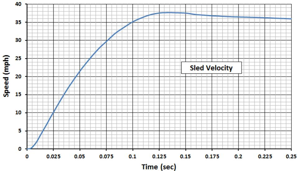
**Figure 4-13. Sled Speed Resulting from the 23g Trapezoidal Crash Pulse during Test**
