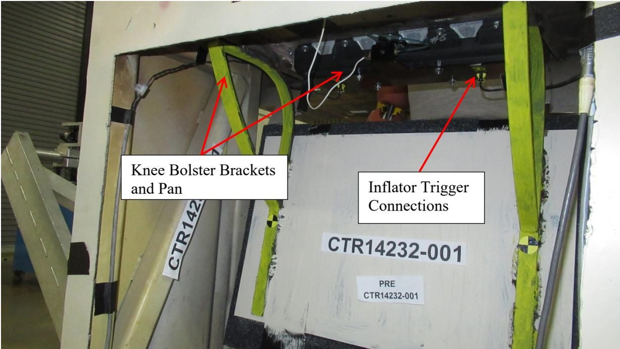
**Figure 4-10. Inflator Firing Trigger Connection**
