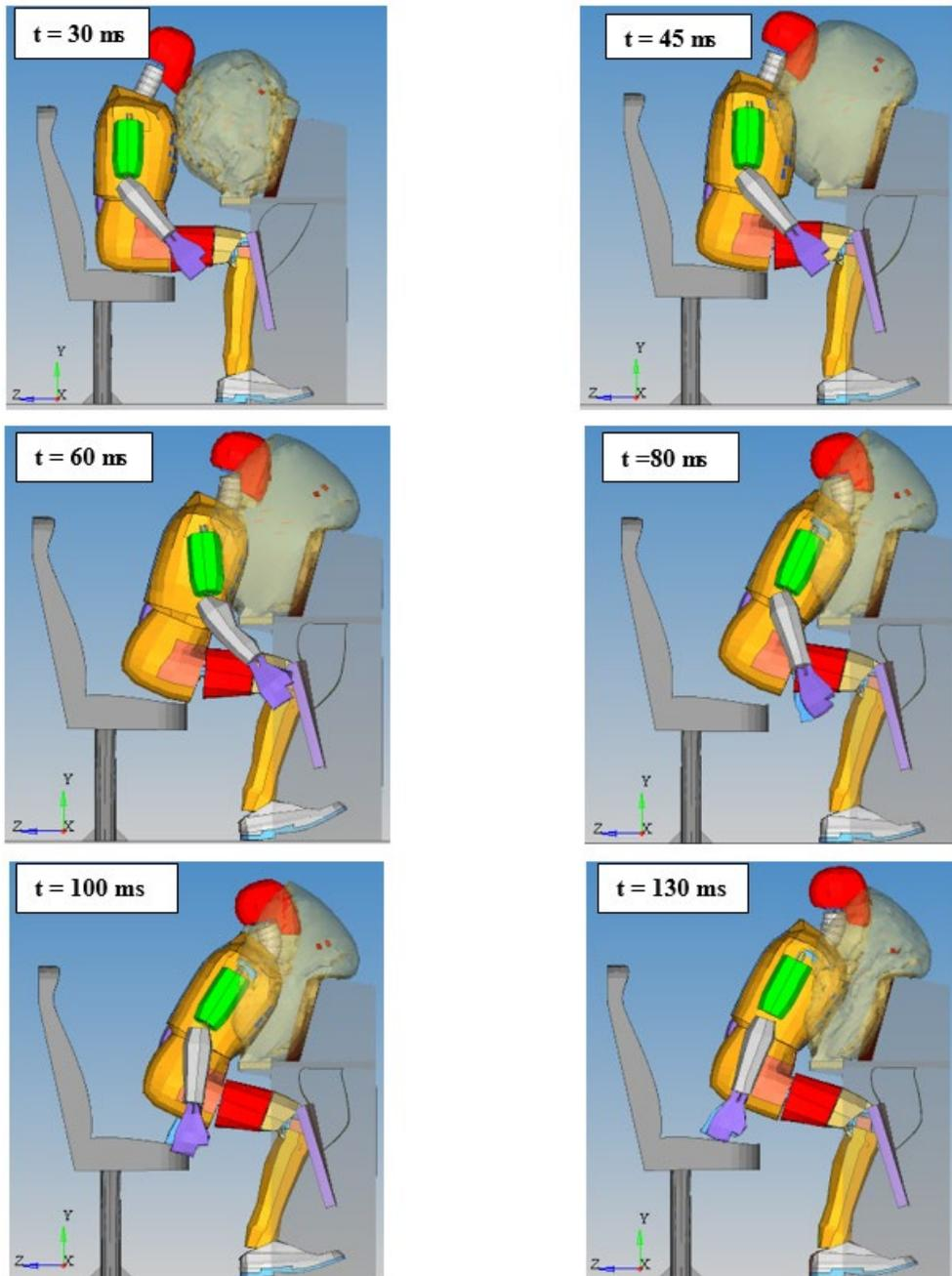
Figure 4-12. ATD Kinematics from LS-Dyna Simulation of the Sled Test
