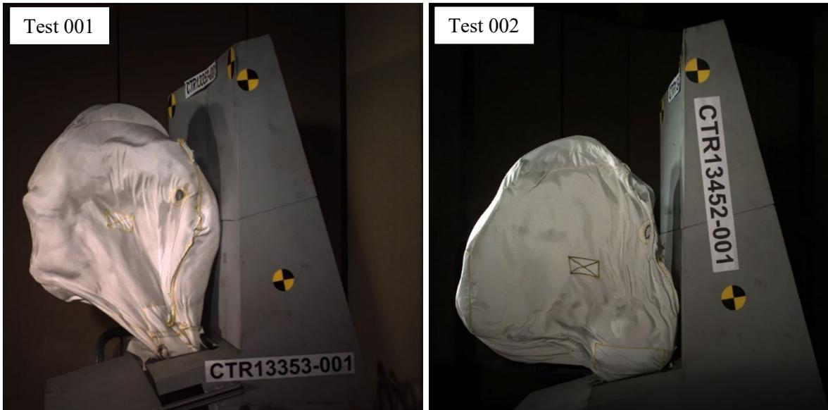
**Figure 4-3. Bag Presentation 20 ms – Test 001/Test 002**
