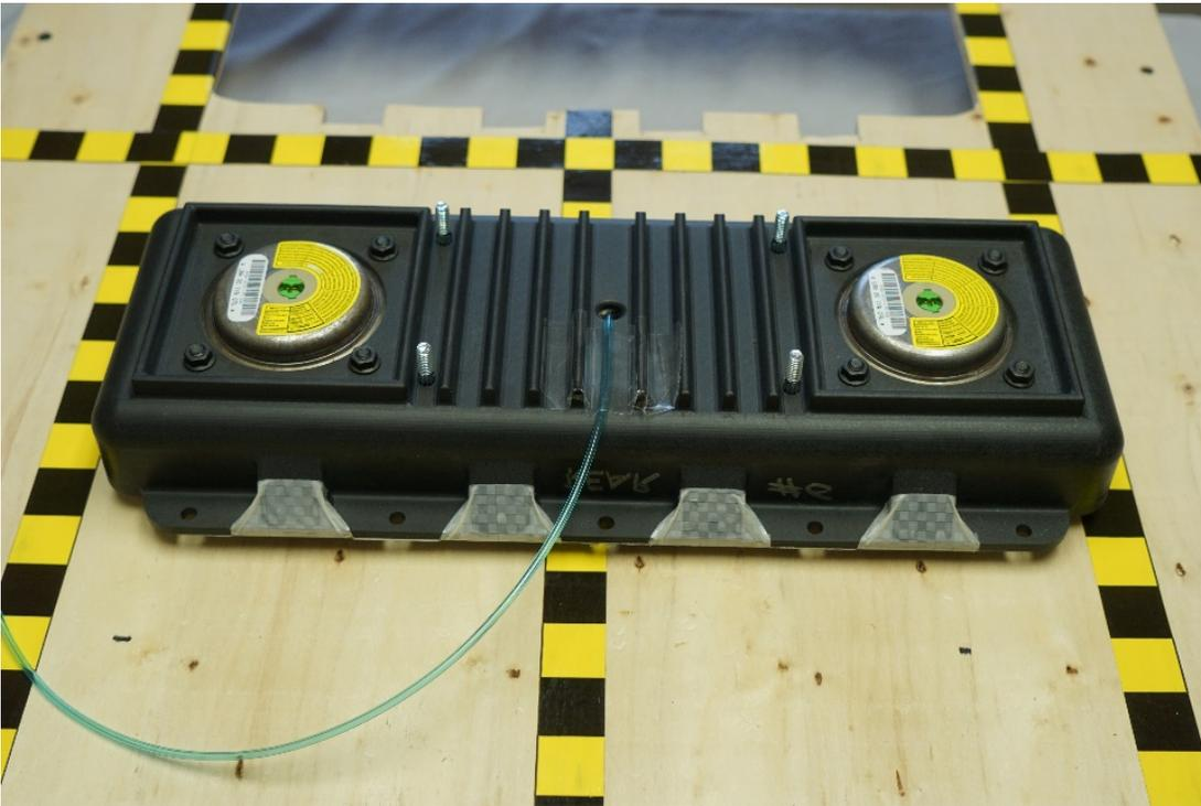
**Figure 3-1. SIPS II Airbag Module without Rear Shield**
