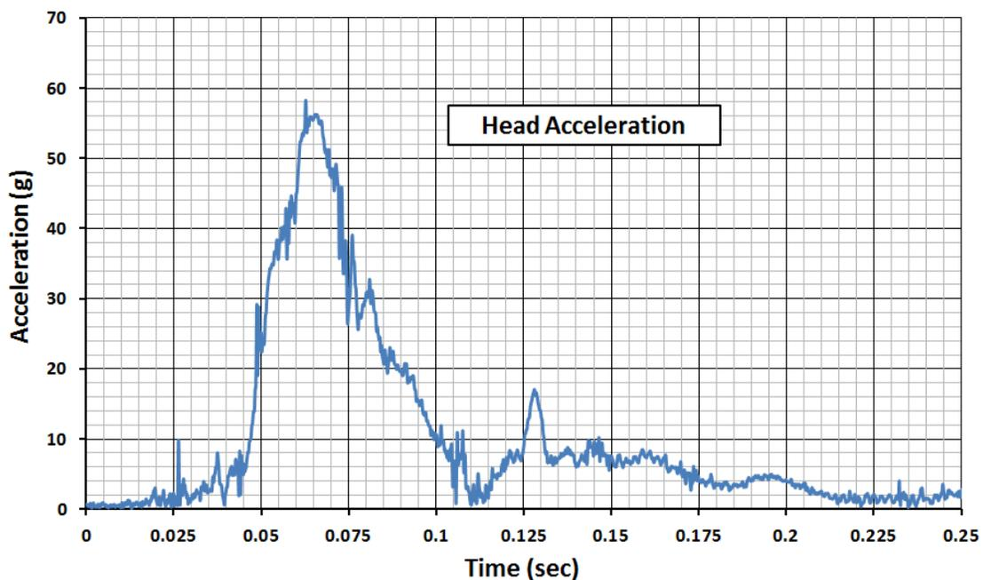
Figure 4-18. Sled Test – Head Acceleration (Resultant) Time History
