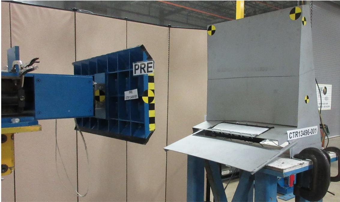
**Figure 4-4. Test Setup of Linear Impact Test**
