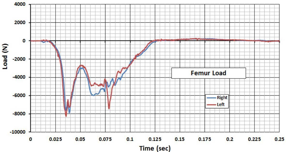
Figure 4-20. Sled Test – Right and Left Femur Load Time History
