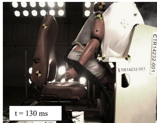
**Figure 4-14. ATD Kinematics from Sled Test**
