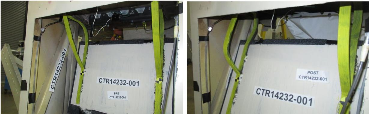
**Figure 4-16. Knee Bolster Assembly: Left – Pre-test, Right – Post-test (Permanent Deformation)**
