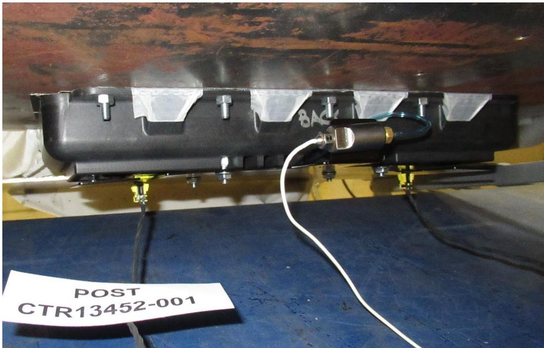
**Figure 3-2. Bottom View – Airbag Module Pan and Pressure Transducer**
