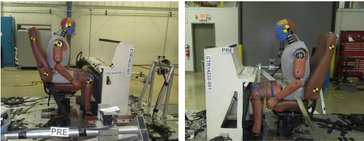
**Figure 4-11. Sled Test Setup – Right and Left Views**
