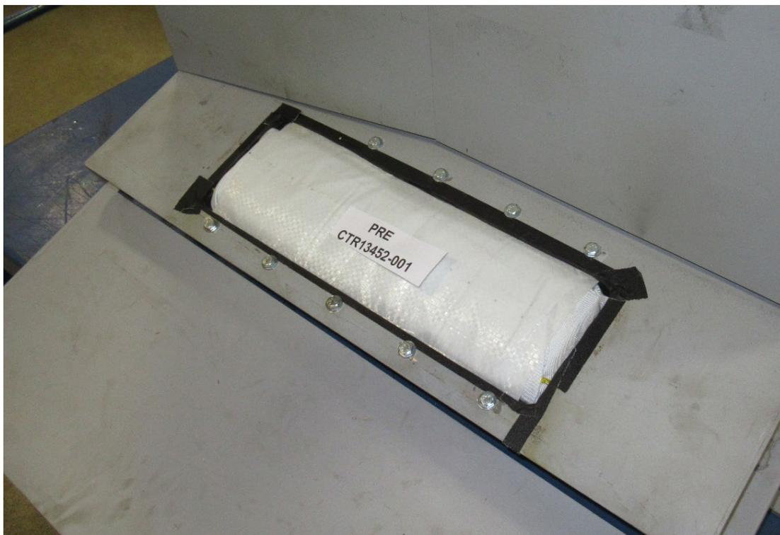
**Figure 3-3. Airbag Module Installed to Desk, Showing the Cover**
