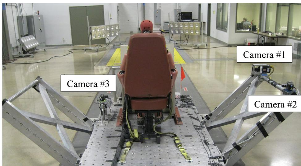
**Figure 4-9. Various Video Camera Locations as Mounted on the Sled**
