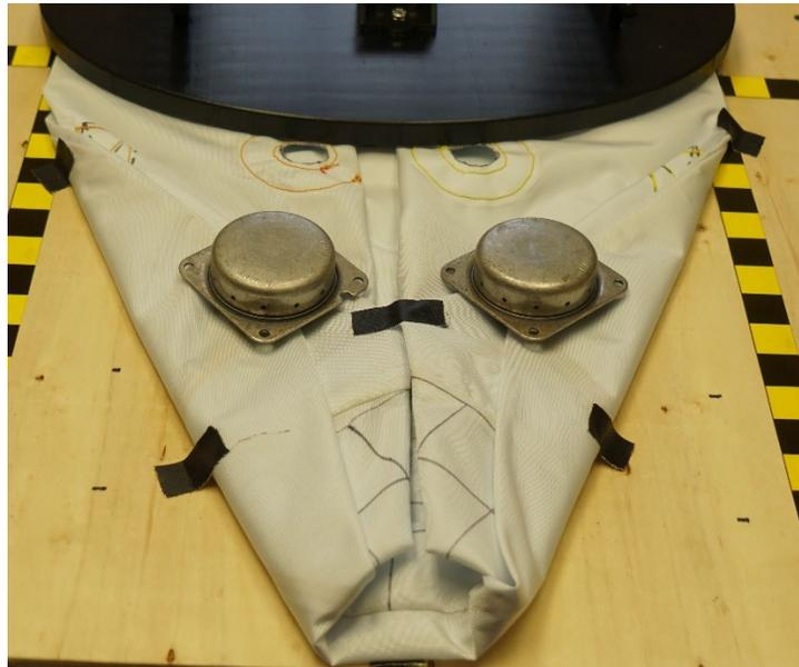
**Figure 3-8. Folding Geometry Prior to Reverse Roll Step**
