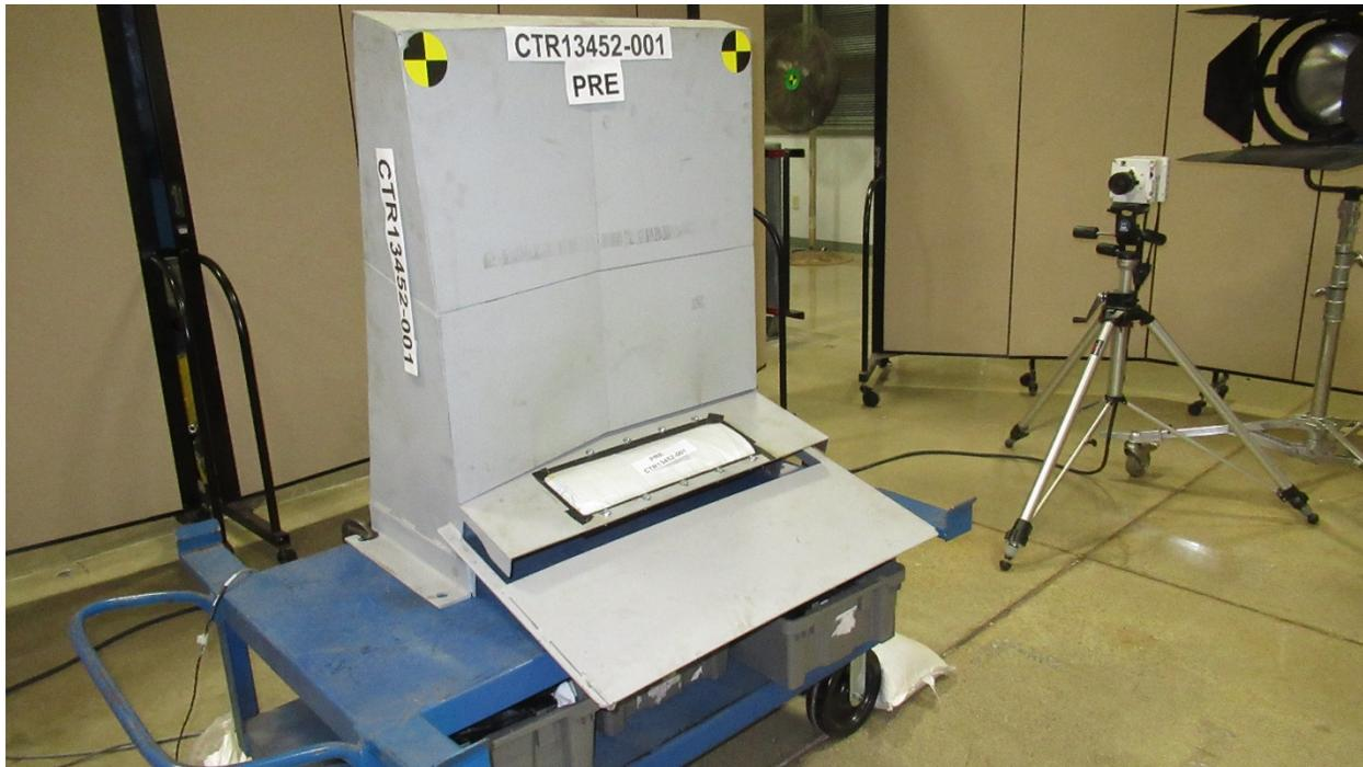
**Figure 4-2. Static Deployment Test Setup**
