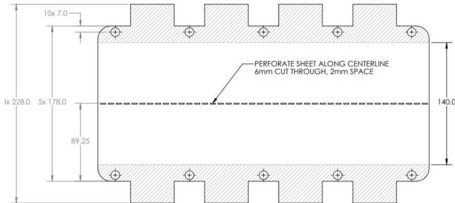
**Figure 3-11. SIPS II Airbag Module Cover Sheet**
