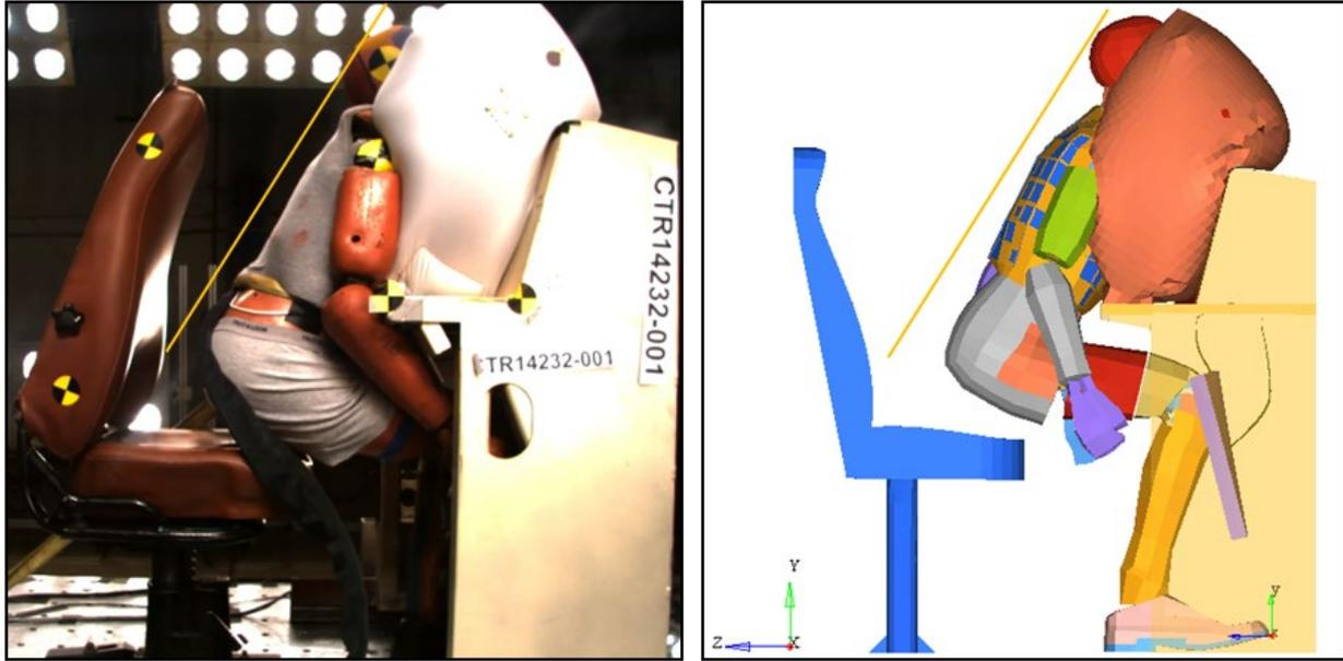
Figure 4-17. Comparison between Sled Test and LS-DYNA Simulation for 80-ms Frame
