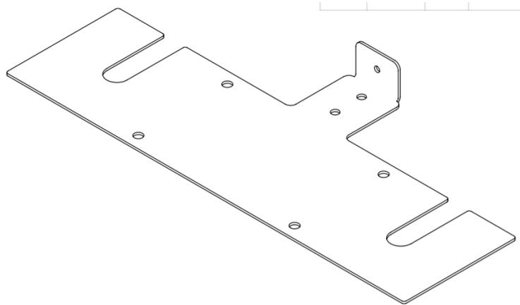
**Figure 3-12. SIPS II Airbag Module Rear Shield**
