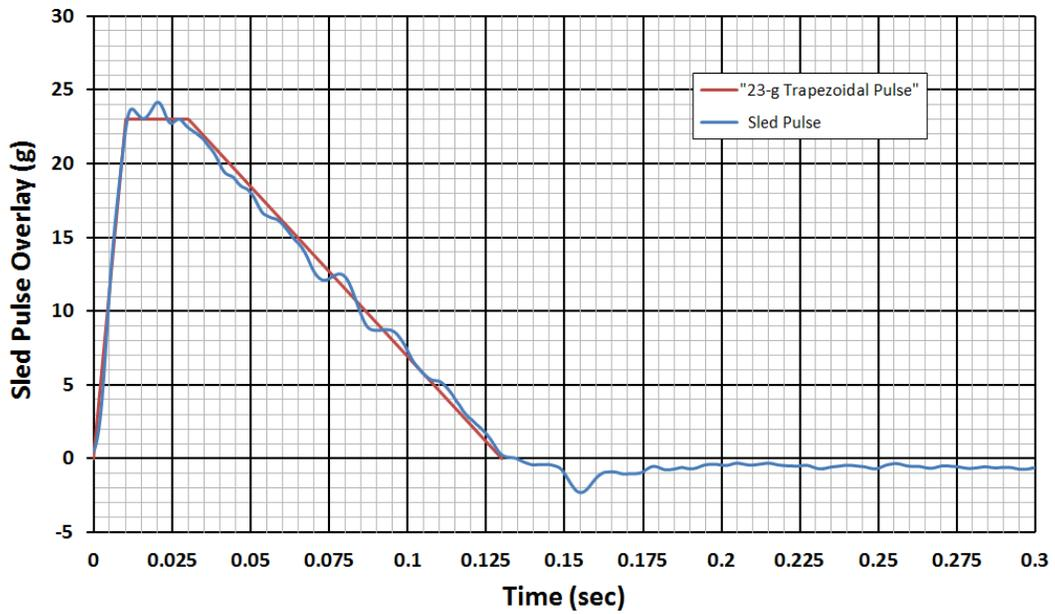
Figure 4-7. Crash Pulse and the Sled Test Acceleration Pulse
