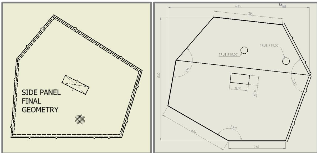
**Figure 3-5. Side Panel Geometry Comparison: SIPS left/SIPS II right**
