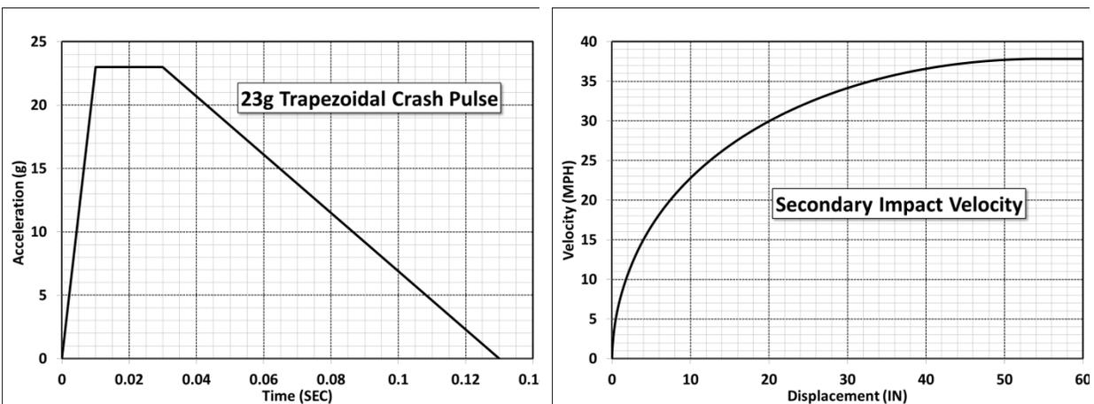
**Figure 2-1. Trapezoidal Crash Acceleration Pulse [4] and Secondary Impact Velocity**
