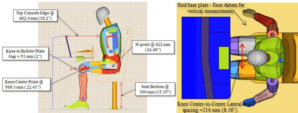
**Figure 4-8. Test Setup – ATD Relative to the Desk**
