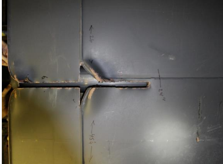
Figure 38. Tear in Test 1 Fuel Tank
