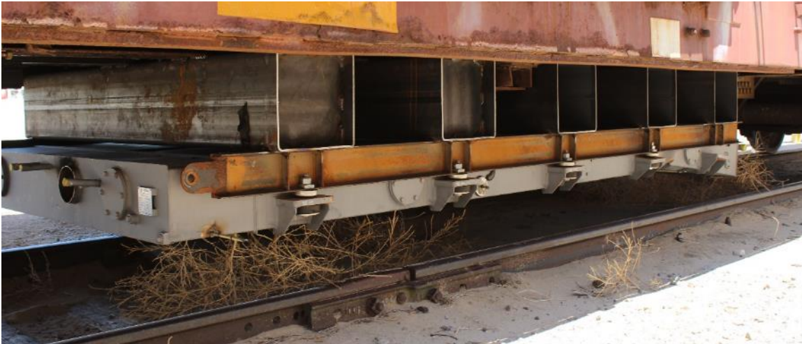
Figure 5. Fuel Tank Mounting Structure
