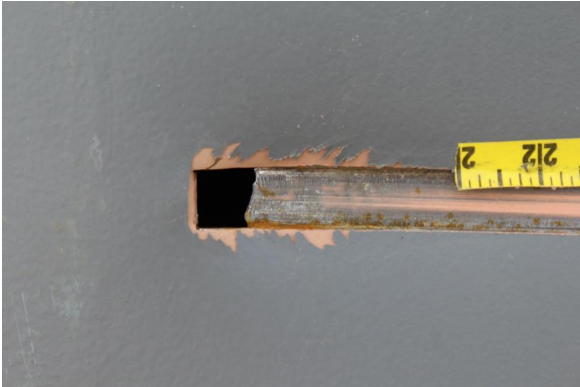
Figure 46. Second Tear in Test 2 Fuel Tank
