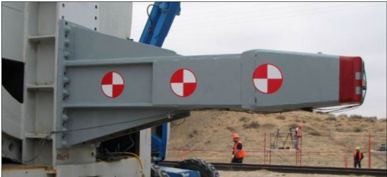
Figure 8. Ram Arm with 12-inch by 12-inch Indenter
