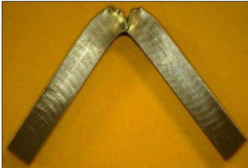
Figure B96. View of Exemplar Post-test CVN Coupon
