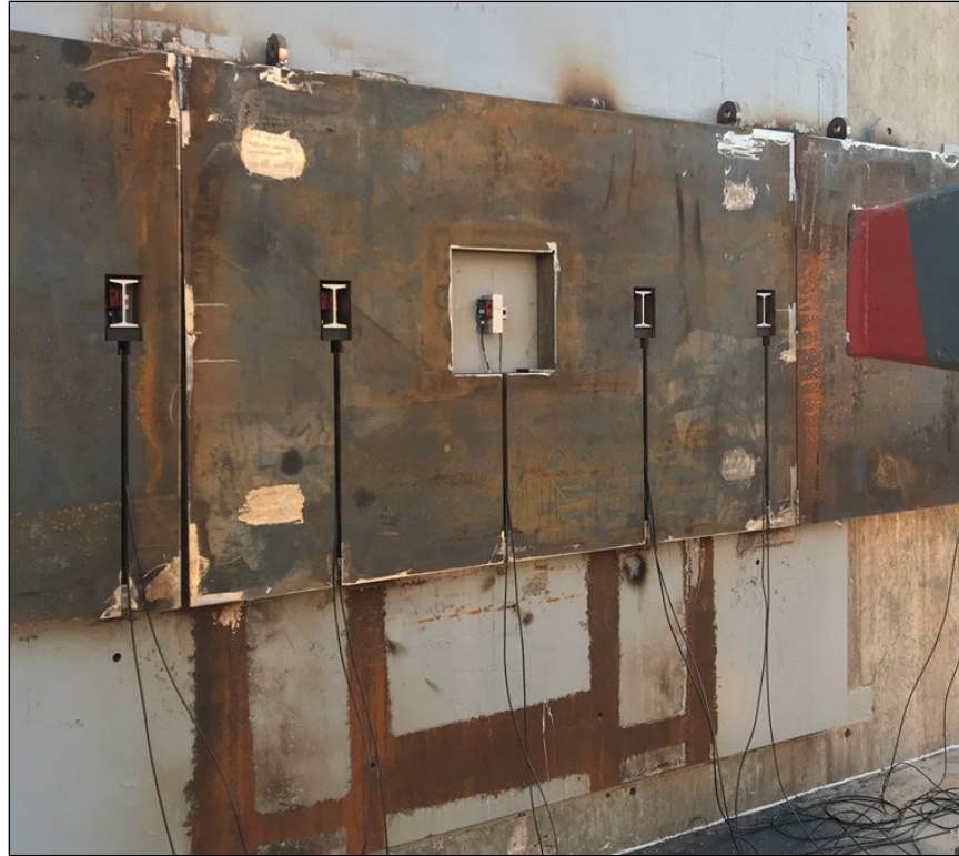
Figure 17. Lasers Displacement Transducers on Crash Wall
