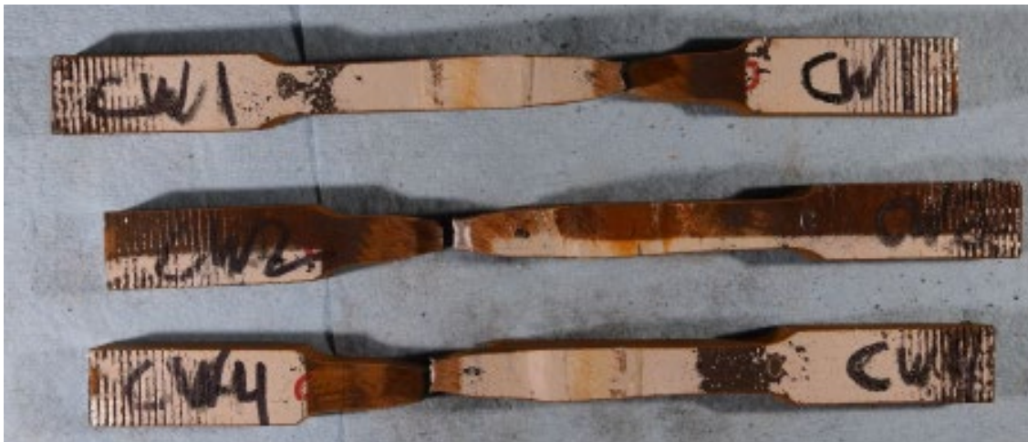
Figure B58. Post-test Closure Weld ASTM-E8 Tensile Coupons
