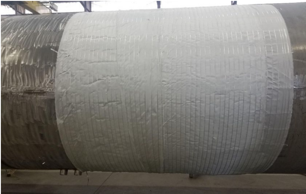
Figure 1. T304 Stainless Steel Inner Tank Wrapped in MLI
