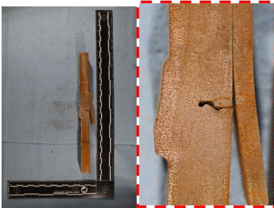
Figure B53. Closure Weld Specimen Rejected Due to Lack of Fusion Defect in Weld
