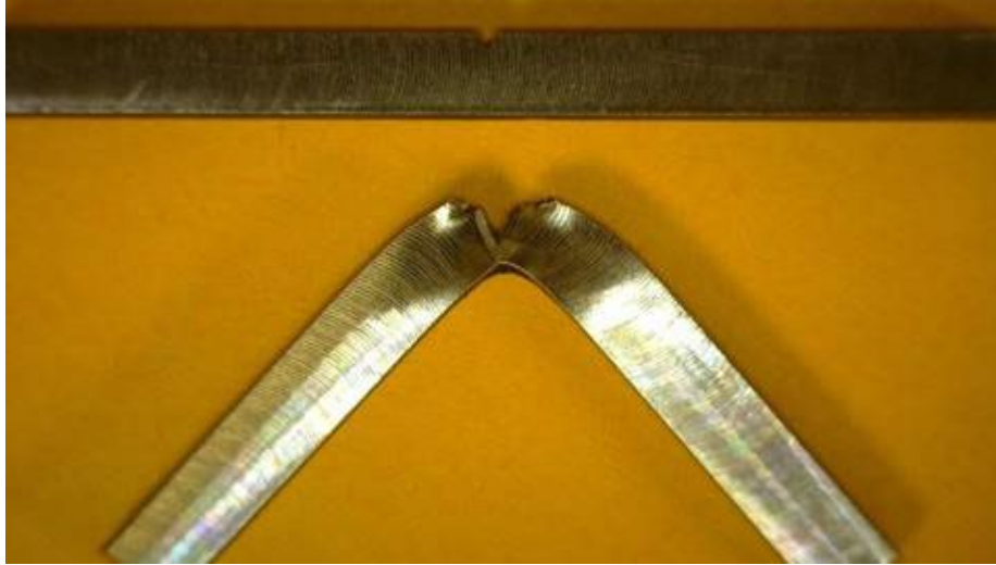
Figure 37. Pre- (top) and Post-test (bottom) CVN Specimens
