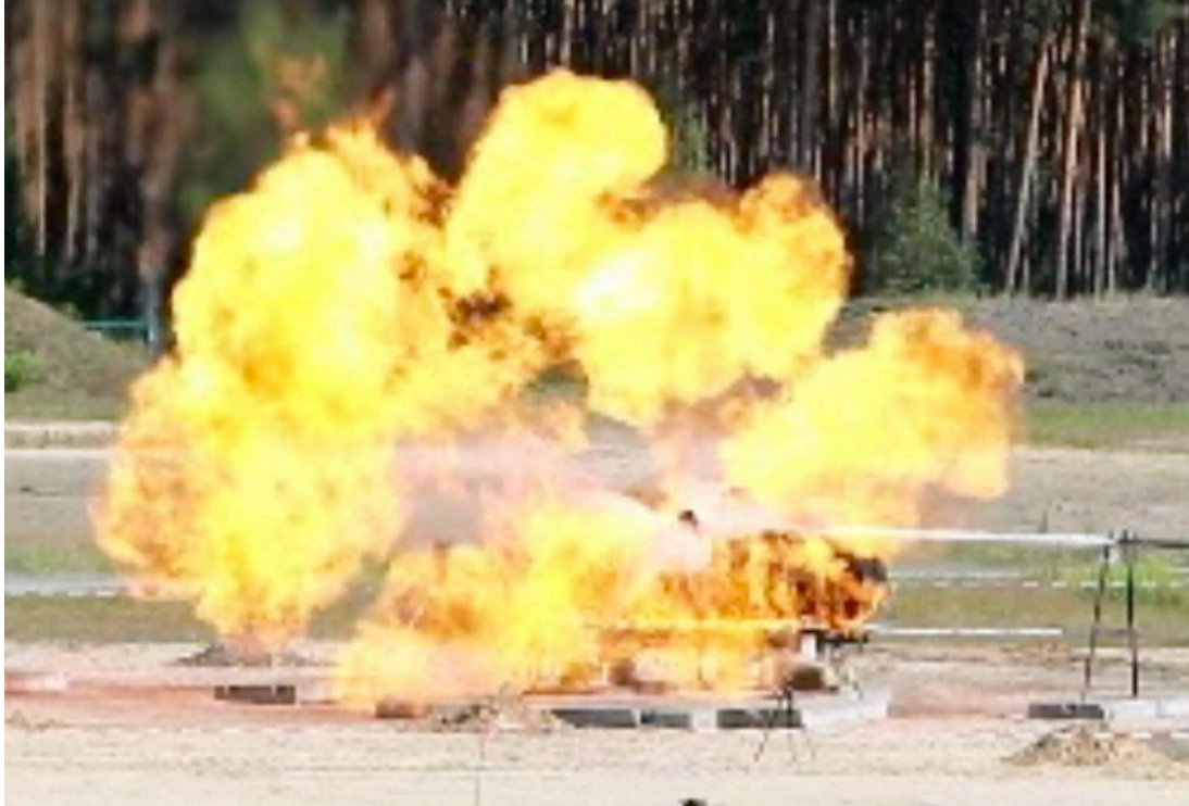
Figure 35. Liquid release followed by ignition – ethanol test #2
