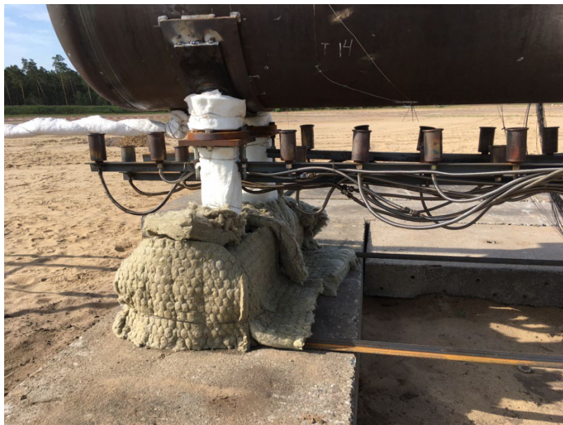
Figure 17. Support legs and water bath with insulation
