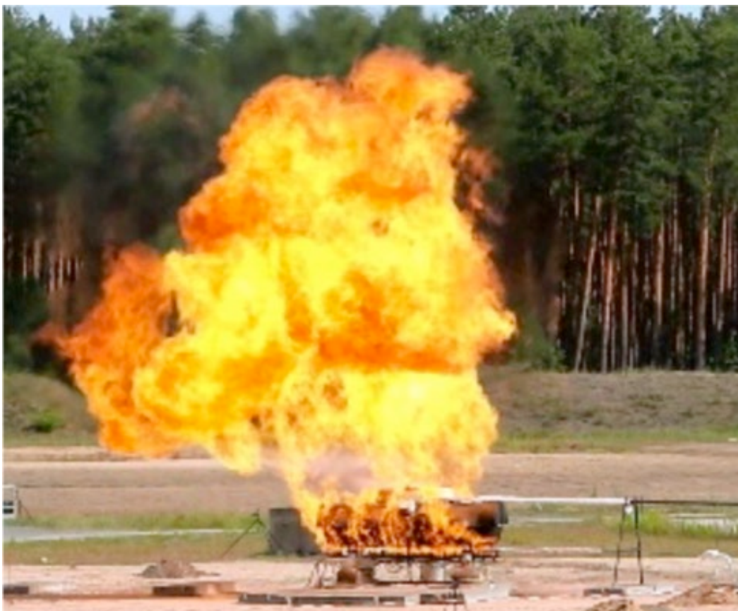
Figure 33. PRD release event – ethanol test #1
