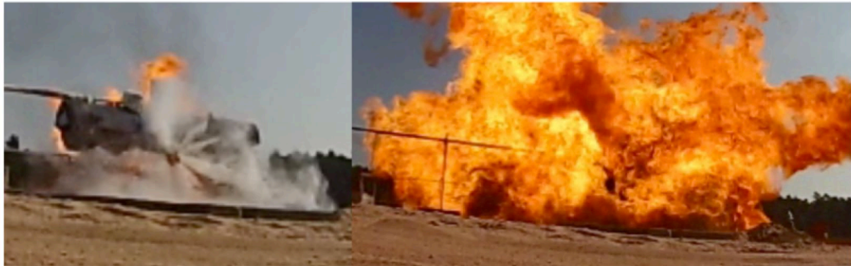
Figure 37. Liquid release followed by ignition – ethanol test #3
