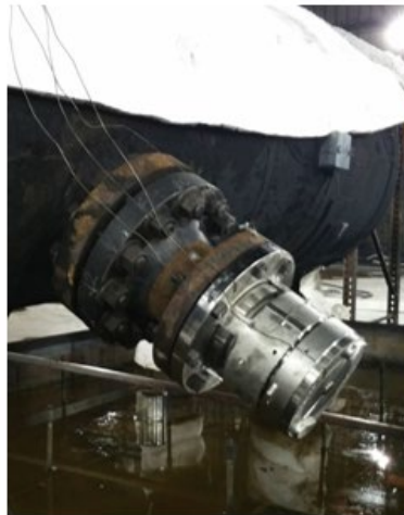
Test # 3 - High capacity PRD mounted at 120° orientation
