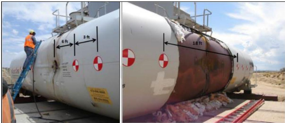
**Figure 34. Test 3 – Deformation to Jacket and Tank**
