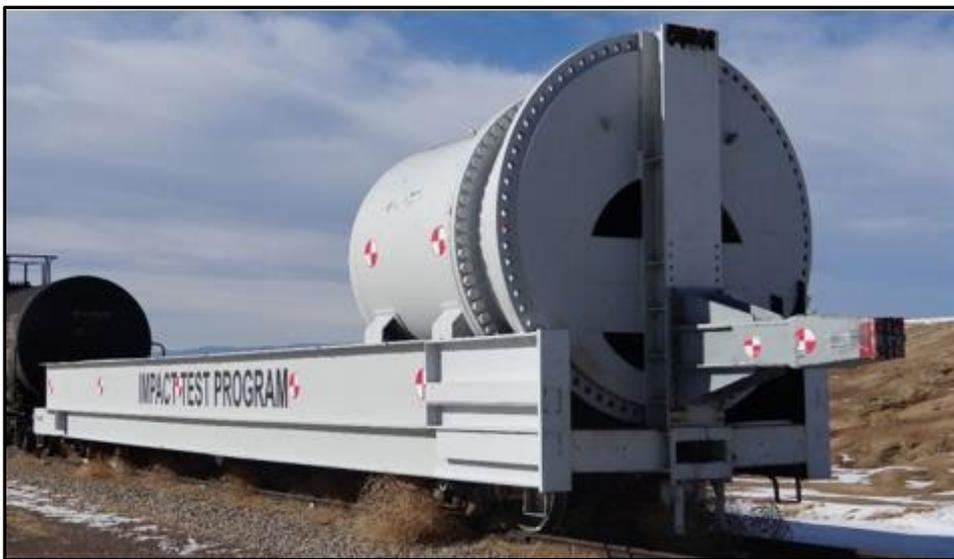
**Figure 38. Test 4 – Impactor Car Configuration Before Test**
