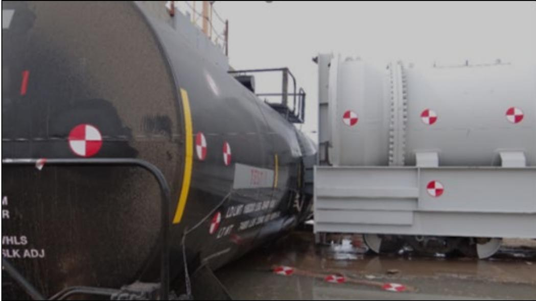
**Figure 39. Test 4 – Post-test Puncture Response of the Tank Car**
