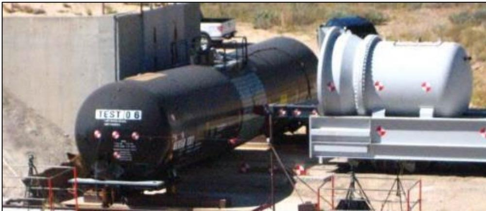
**Figure 58. Test 7 – Test Setup Showing DOT117 Tank Car and Impactor<sup>11</sup>**
