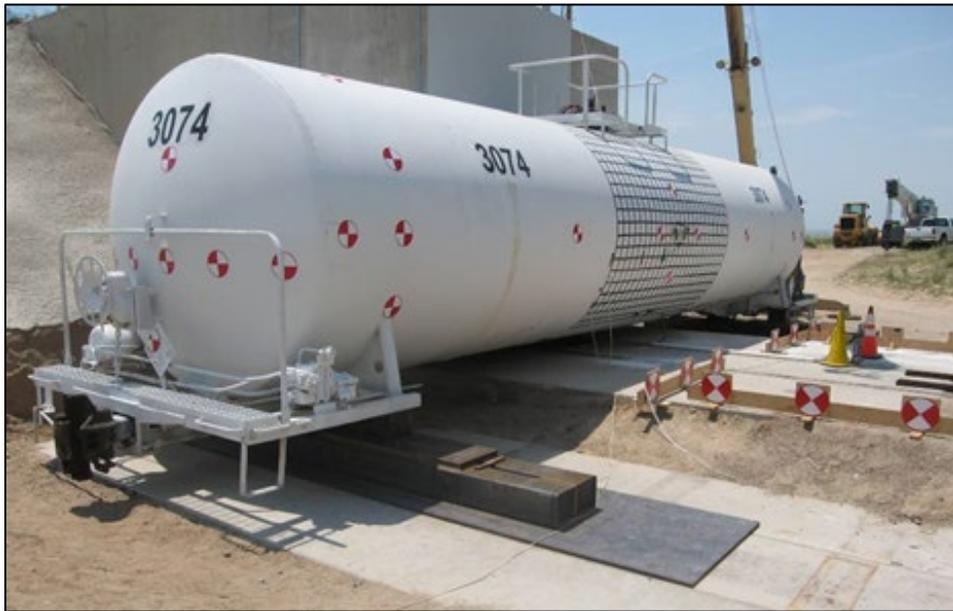
**Figure 25. Test 2 – Tank Car 3074 Mounted on Support Skids**
