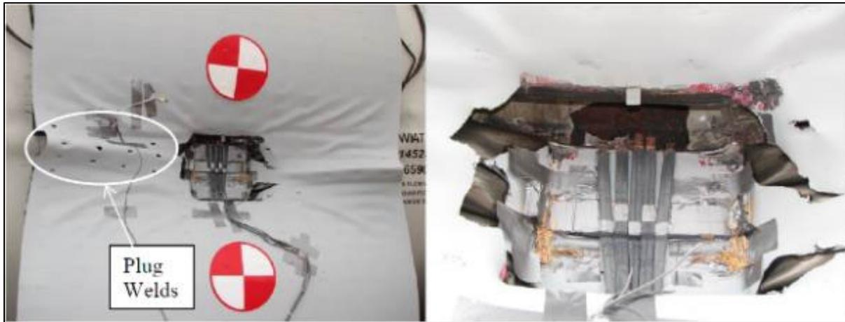
**Figure 33. Test 3 – Damage to Protective Panel**
