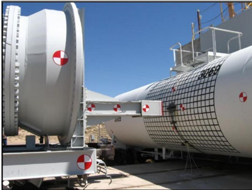
**Figure 16. Test 1 – Test Setup Showing Tank Car**
