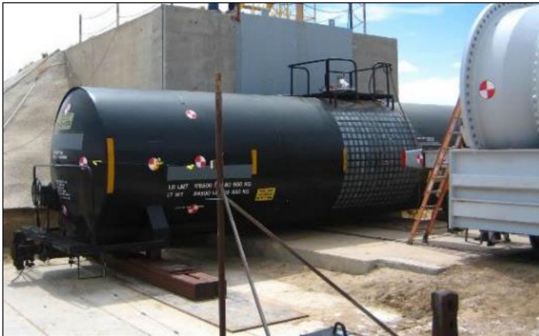
**Figure 55. Test 6 – Test Setup Showing DOT105 Tank Car and Impactor**
