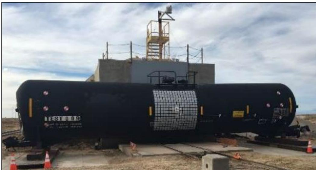
**Figure 64. Test 9 – Test Setup Showing DOT111 Tank Car**
