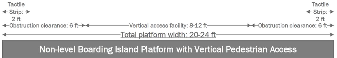
**Figure 6-11. Non-Level-Entry Boarding Island Platform with Vertical Pedestrian Access Minimum Width. Source: USDOT**
