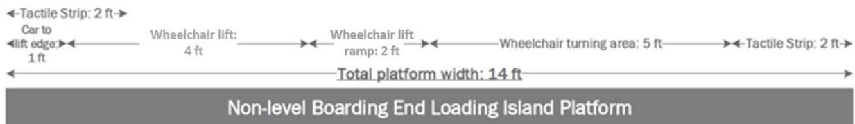
**Figure 6-9. Non-Level-Entry Boarding End-Loading Island Platform Minimum Width. Source: USDOT**
