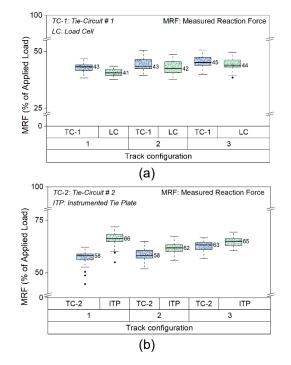
Figure 4: Comparison of TC Results with (a) LCs and (b) ITP
