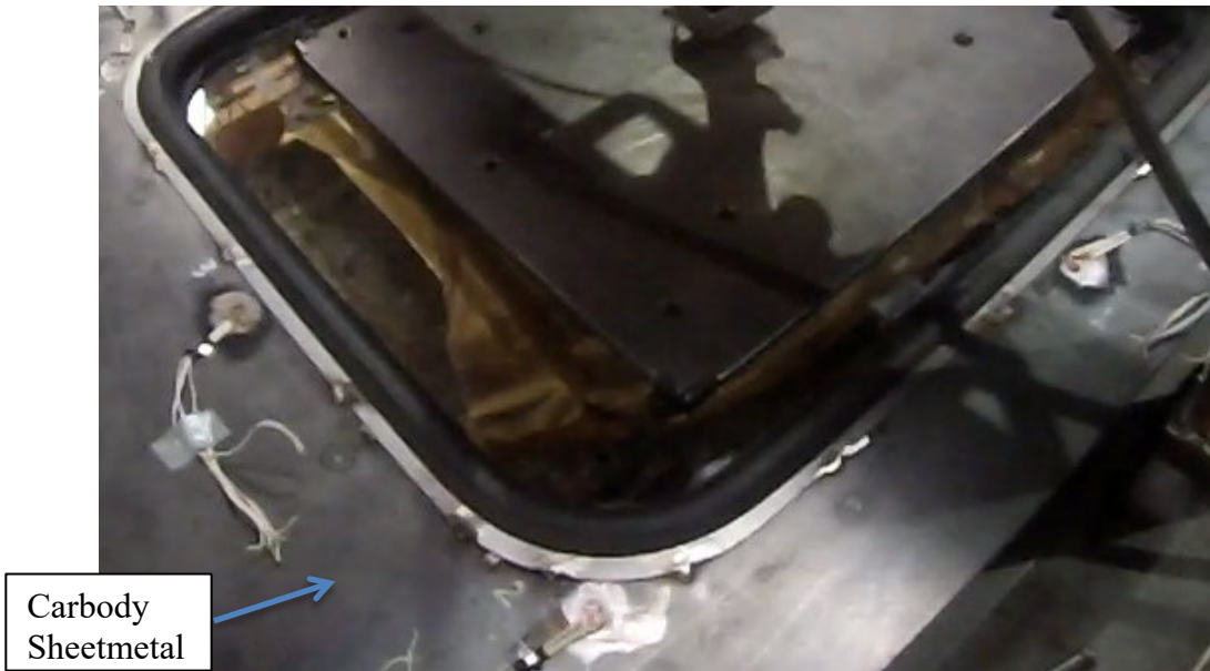
Figure 23. Close-up of shims added to specimen
