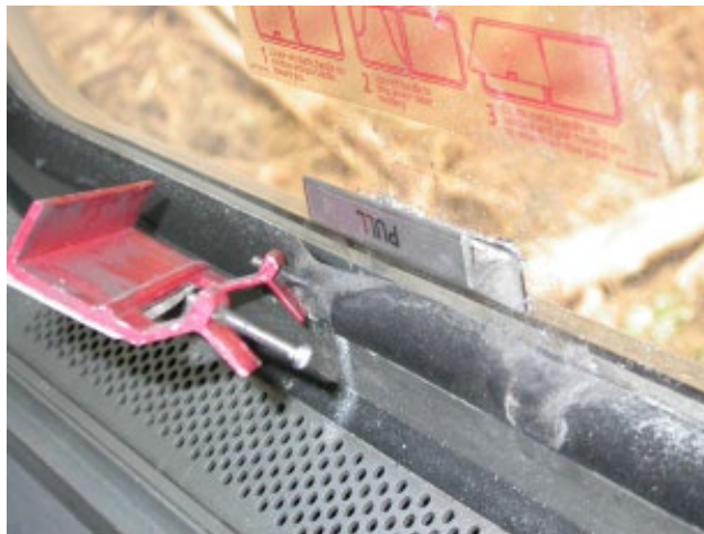
Figure 3. Example of malfunctioning emergency egress features from accident in Flora, MS
