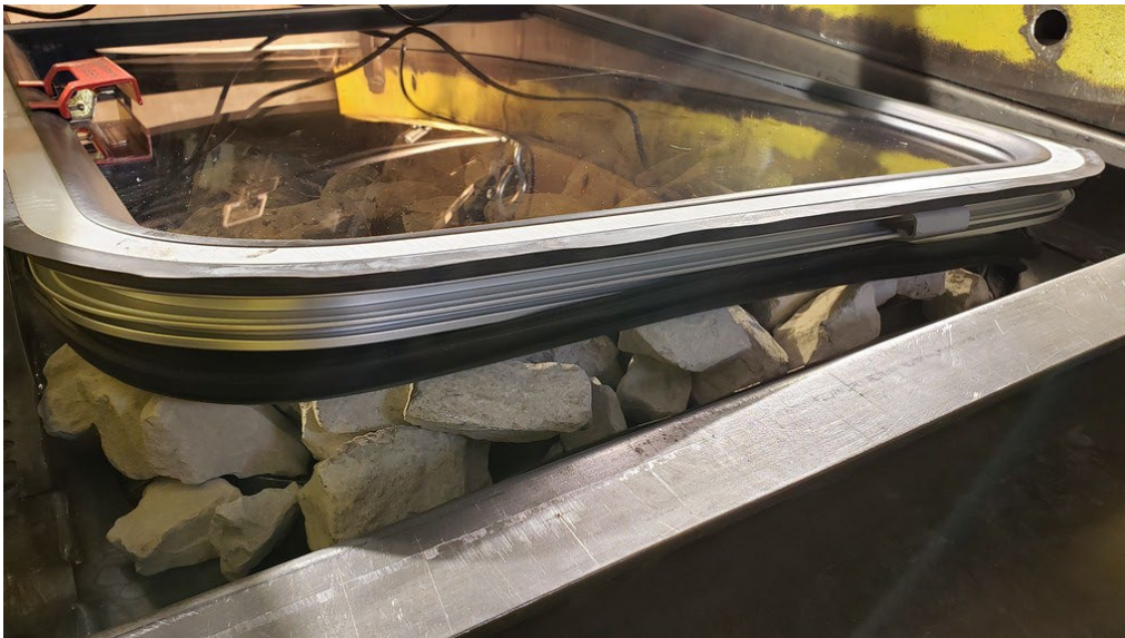
Figure 34. Drag test Specimen 10 – push-through failure at trailing edge
