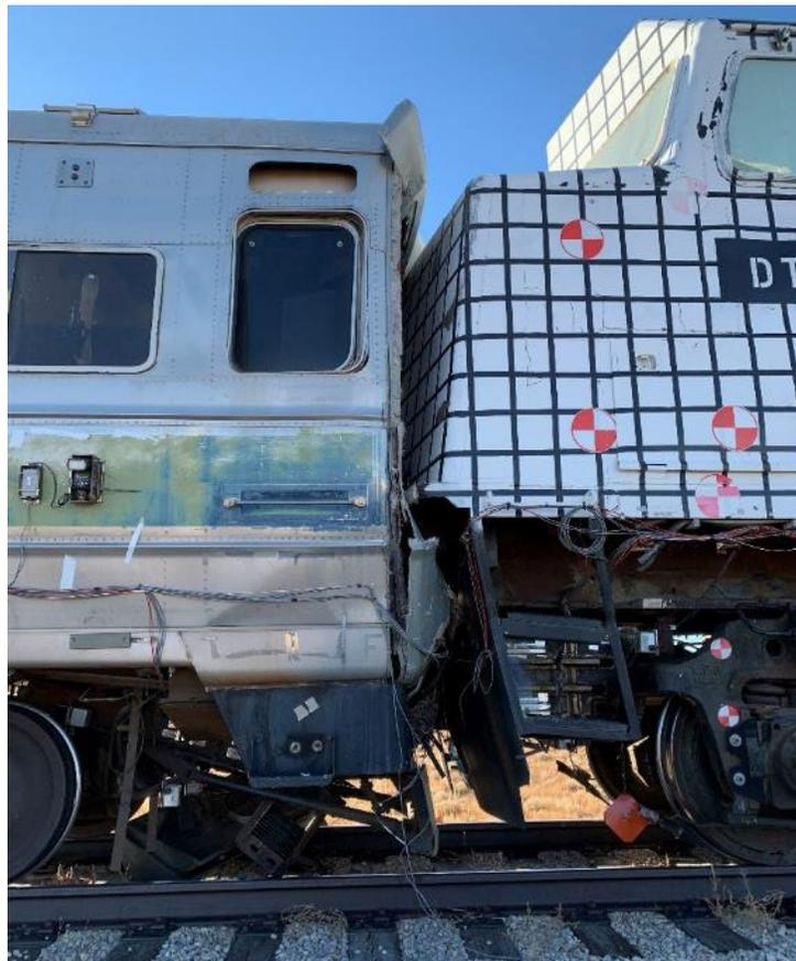
**Figure 54. CEM Locomotive and M1 Passenger Car Intertwined after Test**
