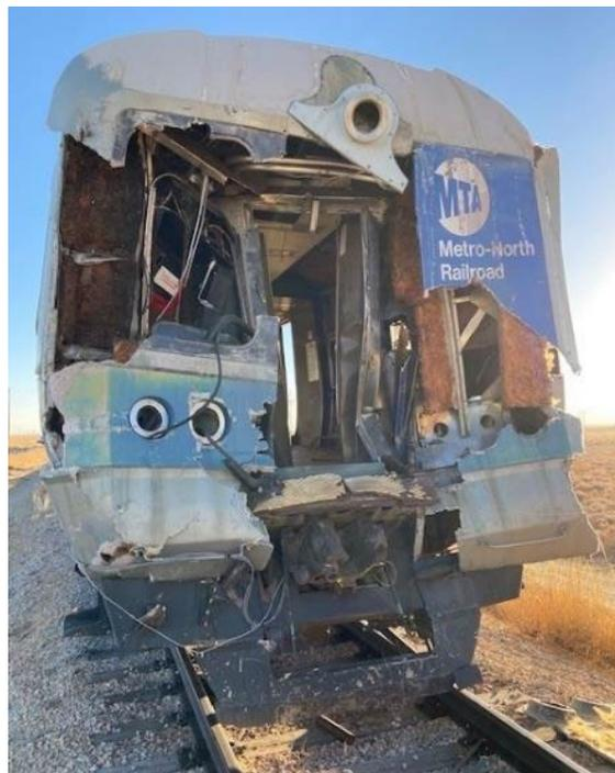
**Figure 57. M1 Passenger Car Impact End (Cab) Exterior**
