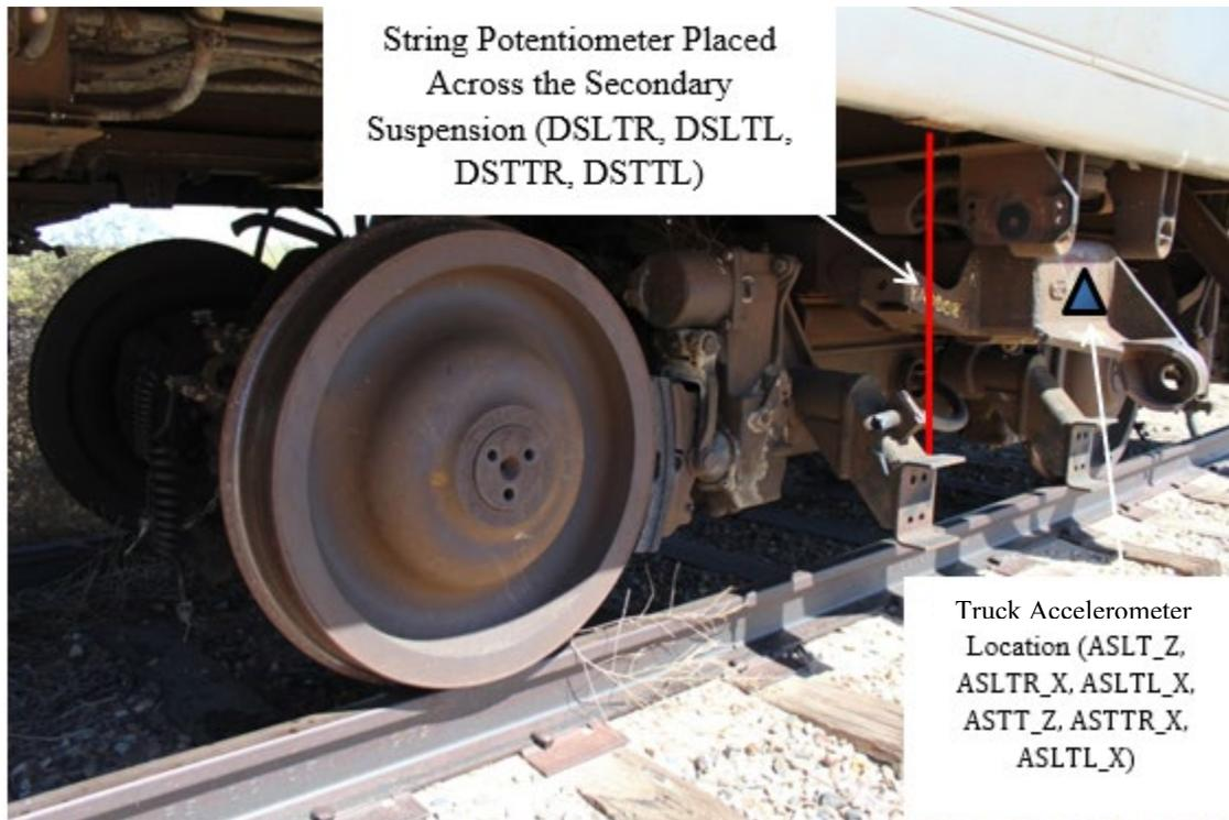
**Figure 17. M1 Passenger Car Truck Instrumentation**
