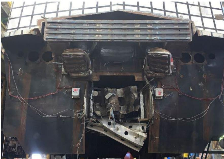
**Figure 49. Crushed Bottom Anti-climbers**
