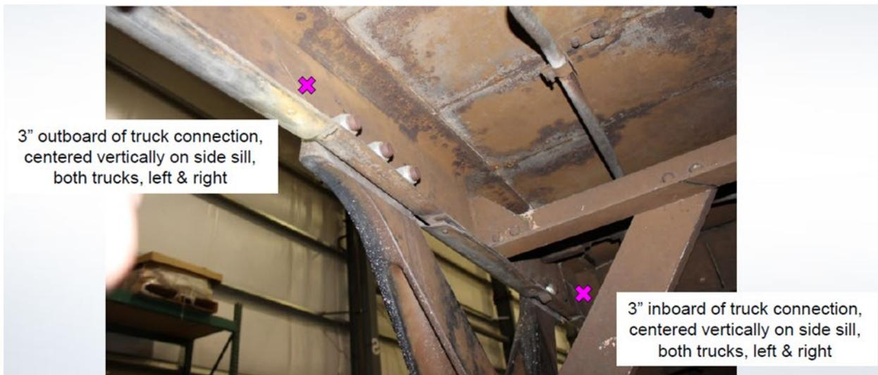
**Figure 23. Strain Gage Locations on the M1 Passenger Car Side Sill**
