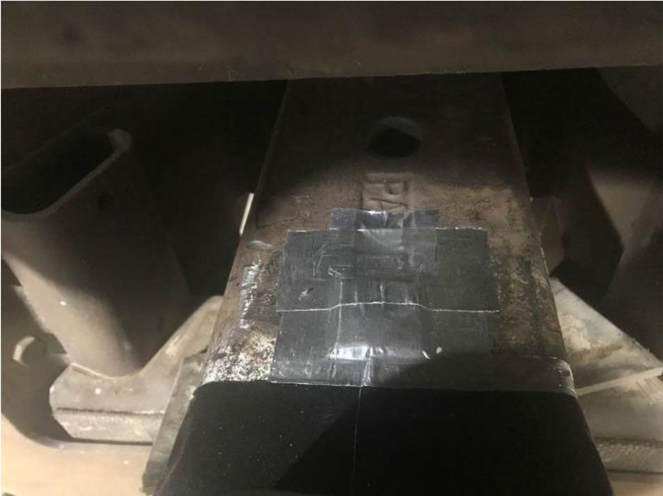
**Figure 25. Strain Gage Location on the M1 Passenger Car Rear Coupler**
