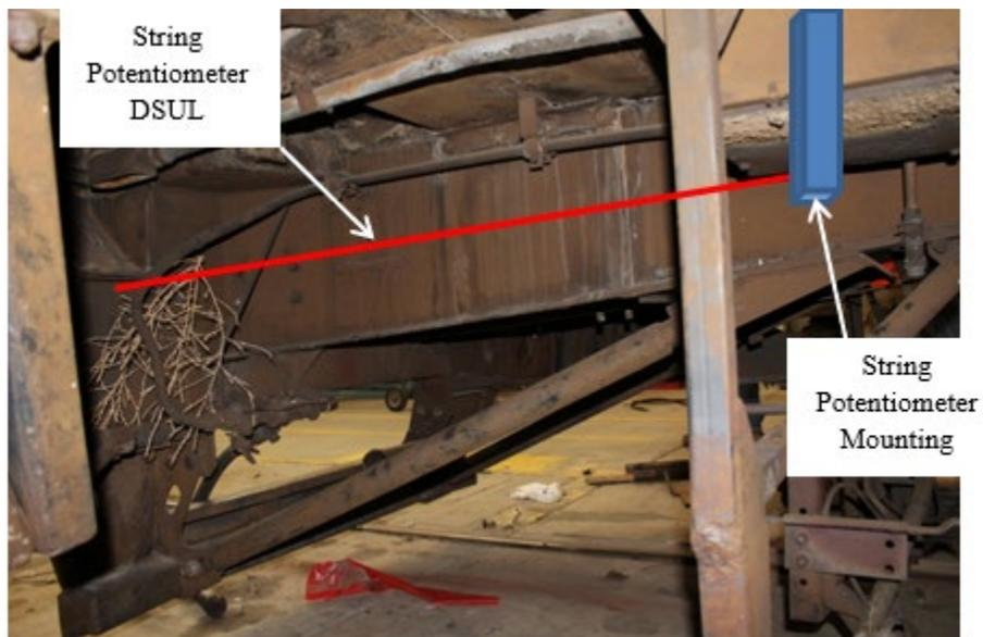
**Figure 19. M1 Passenger Car Left Side Underframe String Potentiometer**
