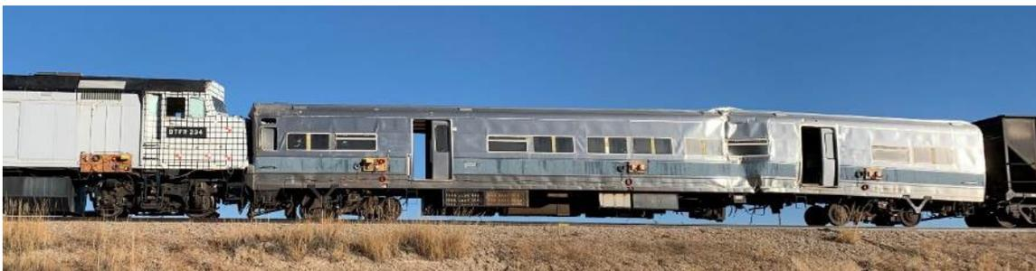
**Figure 55. Buckled M1 Passenger Car**
