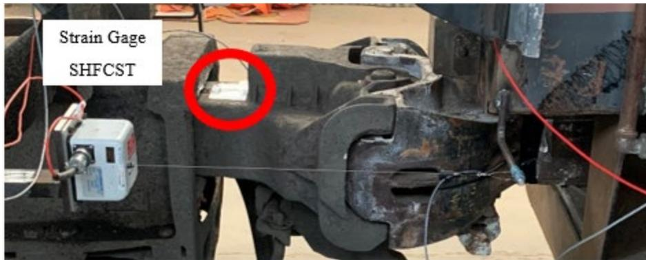
**Figure 27. Strain Gage Location on First Hopper Car Front Coupler**
