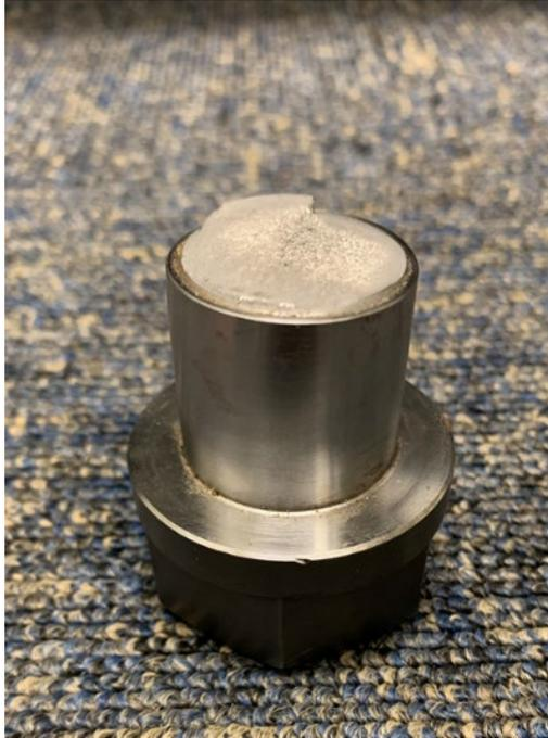
**Figure 52. Activated Shear Bolt after Test**
