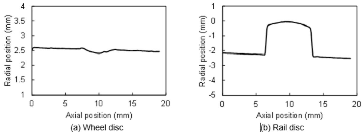
**Figure 18. Contact Surface Profiles of Test Discs
