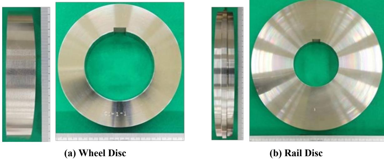
Figure 4. Photos of Wheel and Rail Test Discs
