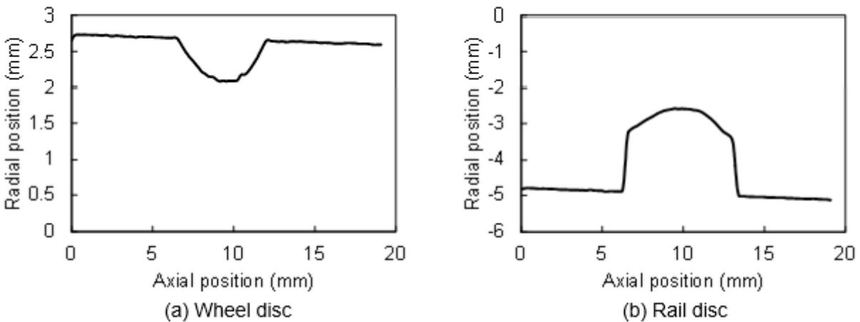
**Figure 12. Contact Surface Profiles of Test Discs
