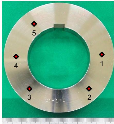
**Figure 1. Measurement Positions of Rockwell Hardness on Wheel Disc**
