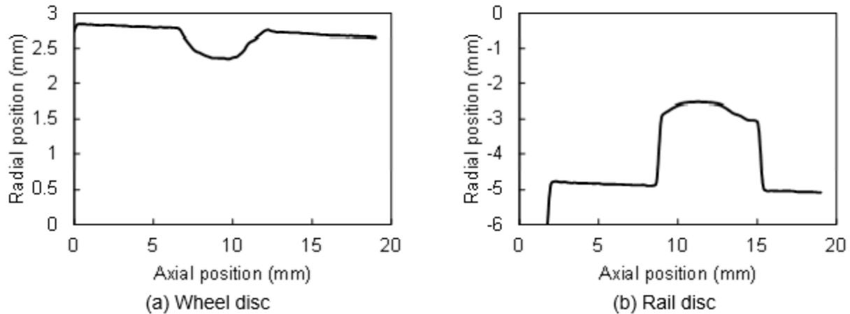
**Figure 9. Contact Surface Profiles of Test Discs
