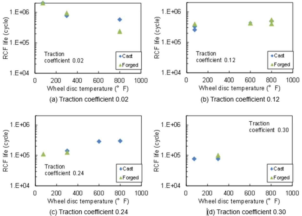
**Figure 20. RCF Life as a Function of Wheel Disc Temperature**
