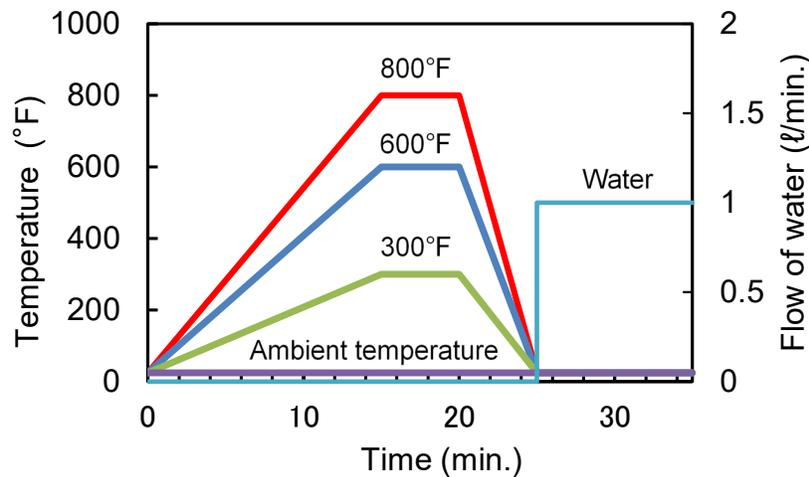
**Figure 6. Thermal Cycle of Wheel Disc and Variation of Water Flow**
