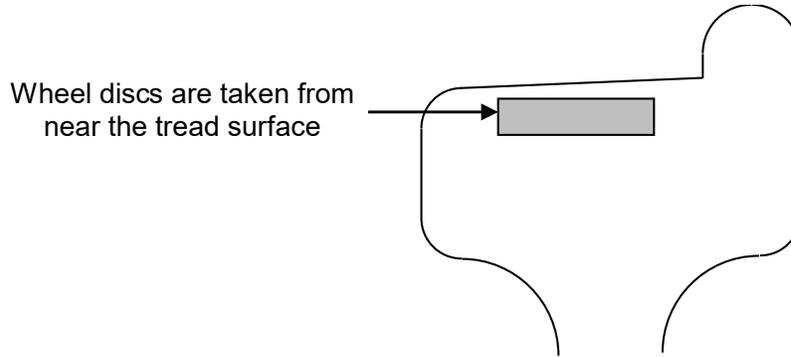
**Figure 2. Schematic of Wheel Disc Sampling Position**
