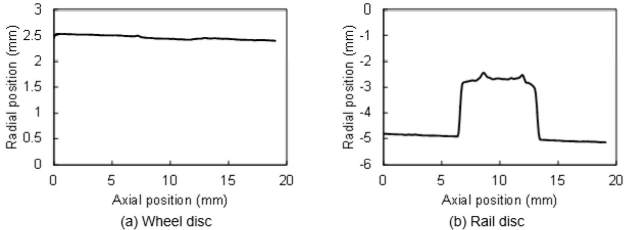
**Figure 15. Contact Surface Profiles of Test Discs
