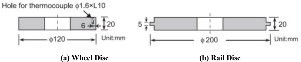
**Figure 3. Schematic of Wheel and Rail Test Discs**
