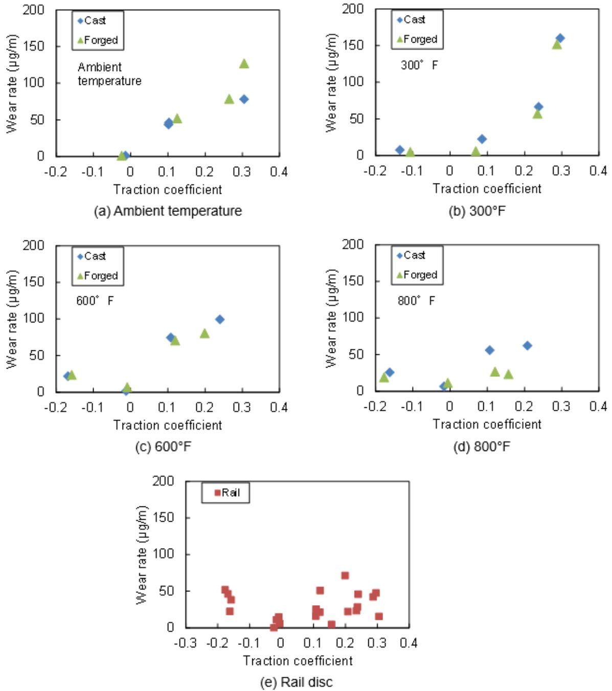
**Figure 21. Wear Rate as a Function of Traction Coefficient**
