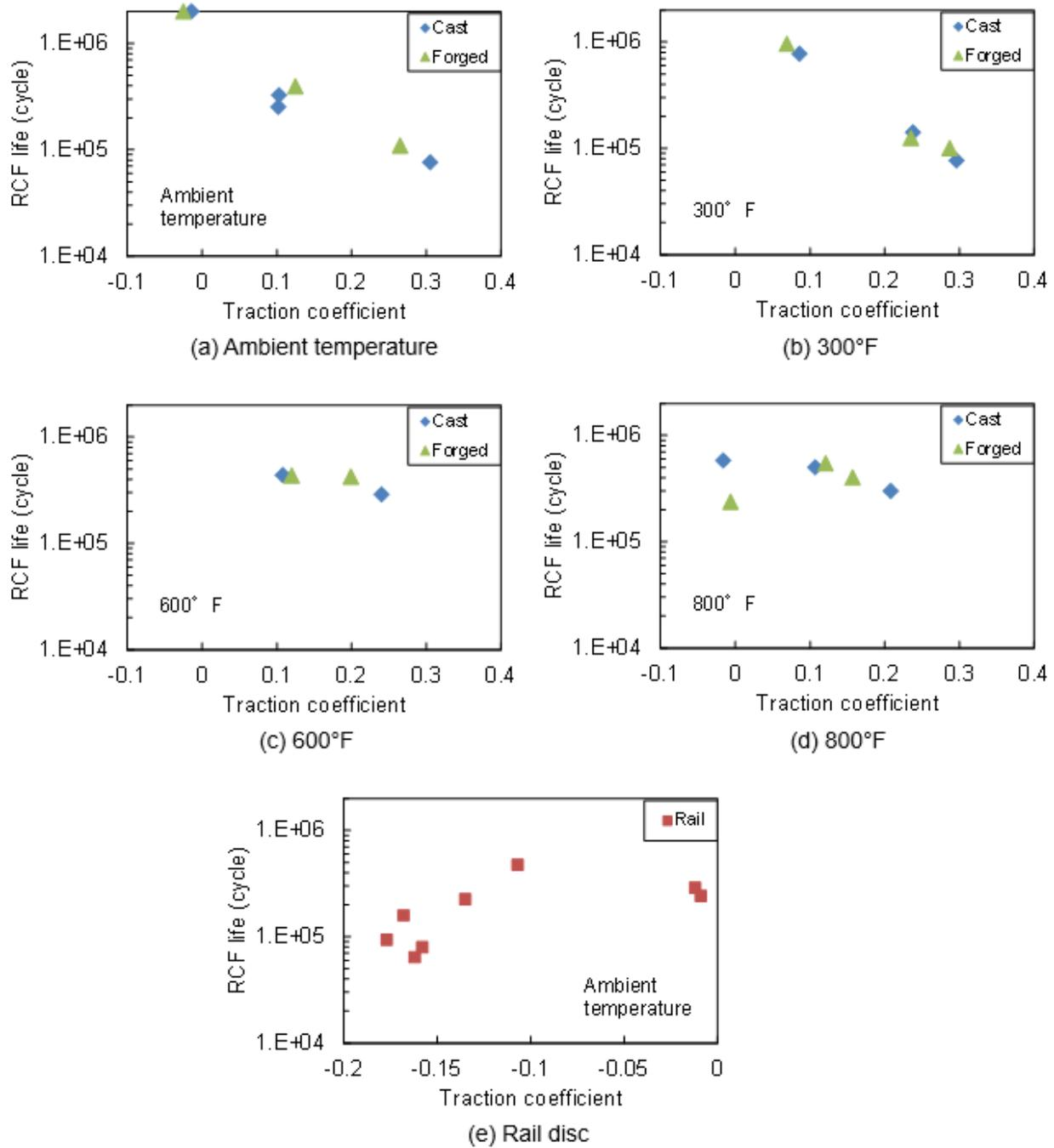
**Figure 19. RCF Life as a Function of Traction Coefficient**
