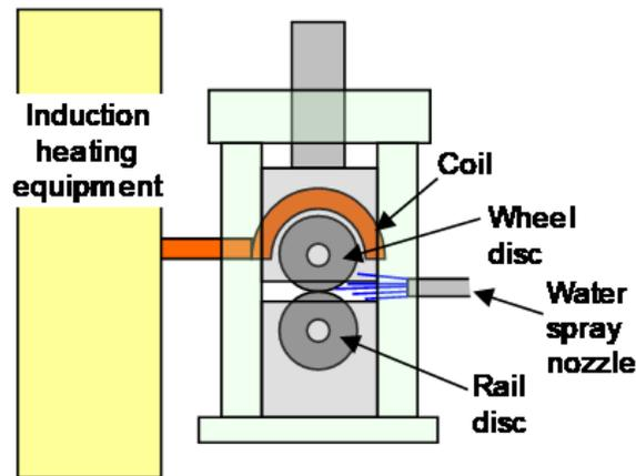
Figure 5. Schematic of the Twin Disc Testing Machine
