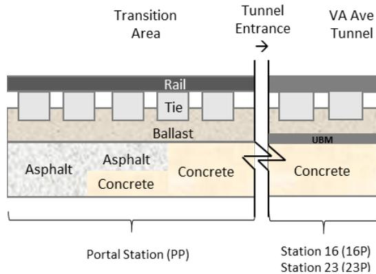
**Figure 1. Transition from asphalt to concrete at the Portal location**
