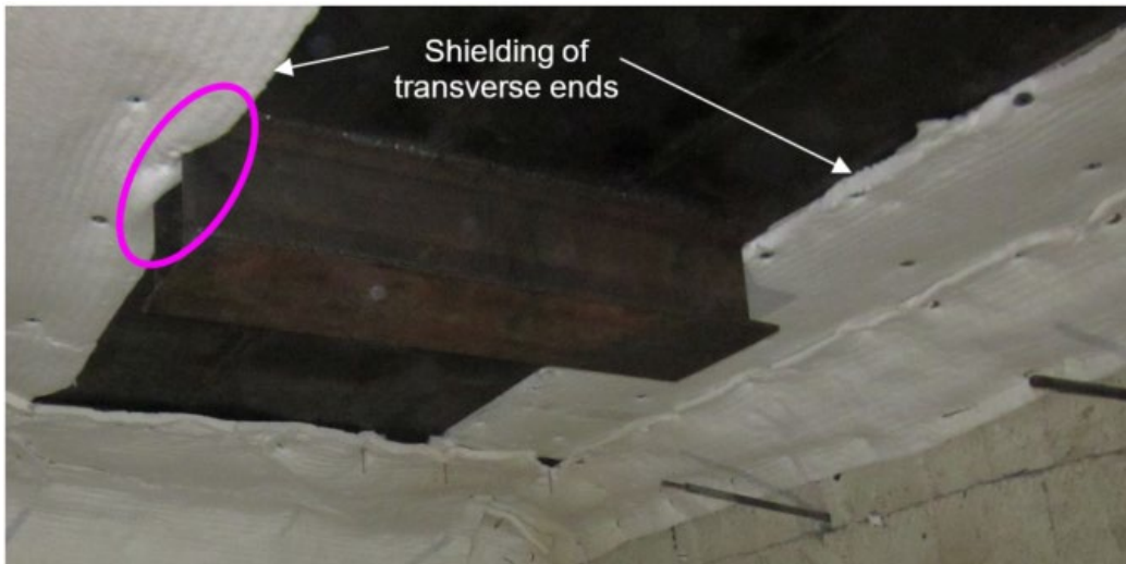
Figure 77. Exposed surface of Test Article 3b just prior to testing
