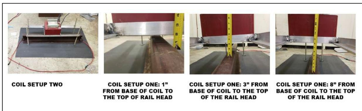
**Figure 32. Tx Coil Setup Two**
