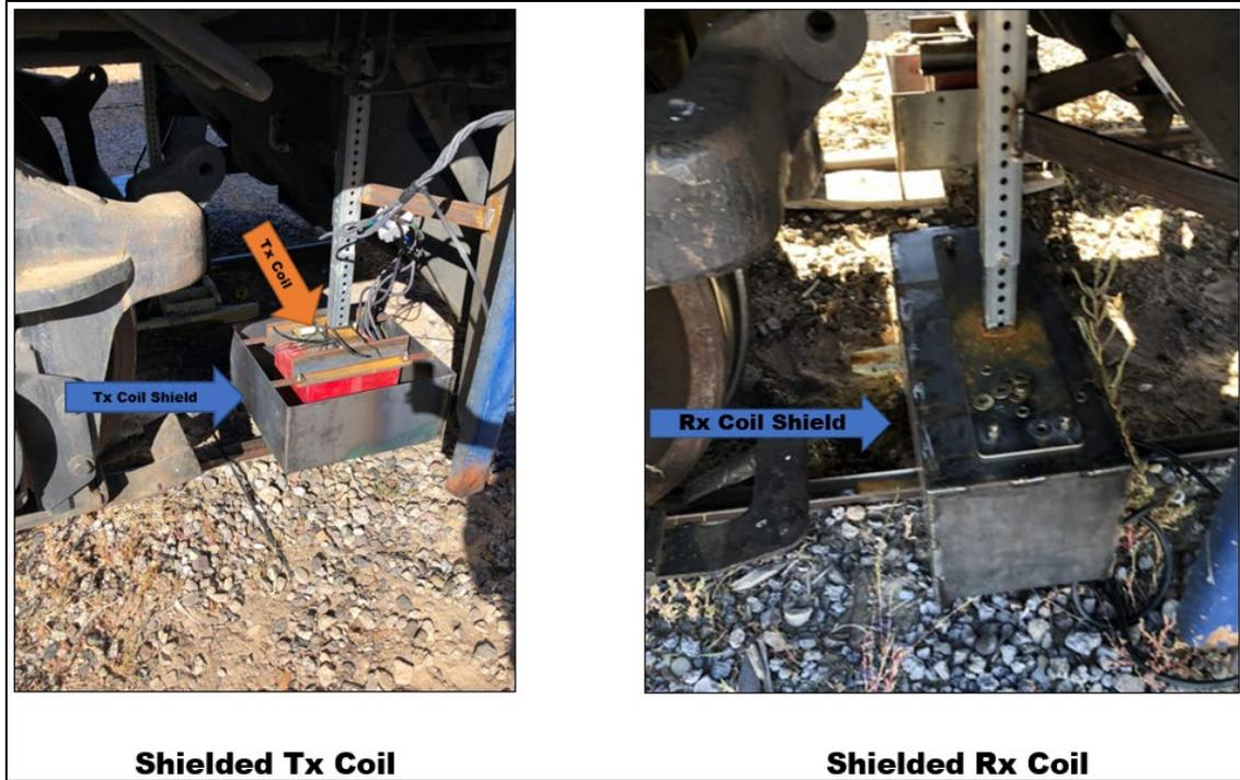
Figure 61. Images of Shielded Tx and Rx Coils
