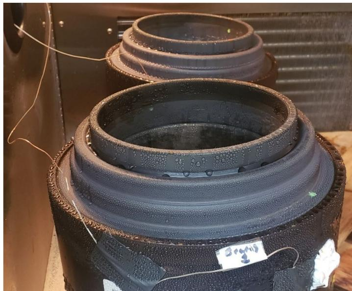
**Figure 4. Bearings in Environmental Chamber**
