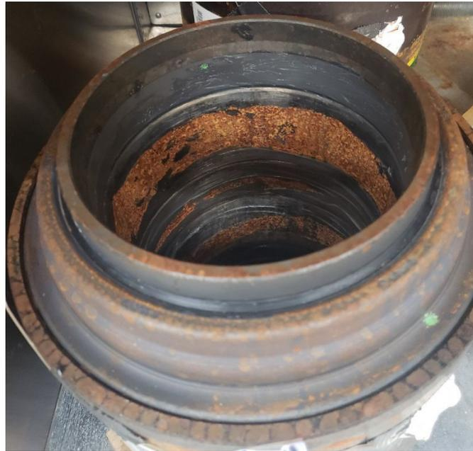
**Figure 5. Corrosion on Bearing Surfaces**
