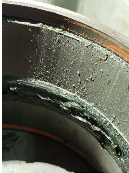
**Figure 1. Bearing Cup Running Surface with Water Ingress**
