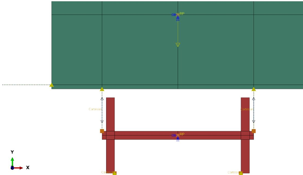
**Figure 34. Loads in 2D Rollover Model in Abaqus/Explicit**
