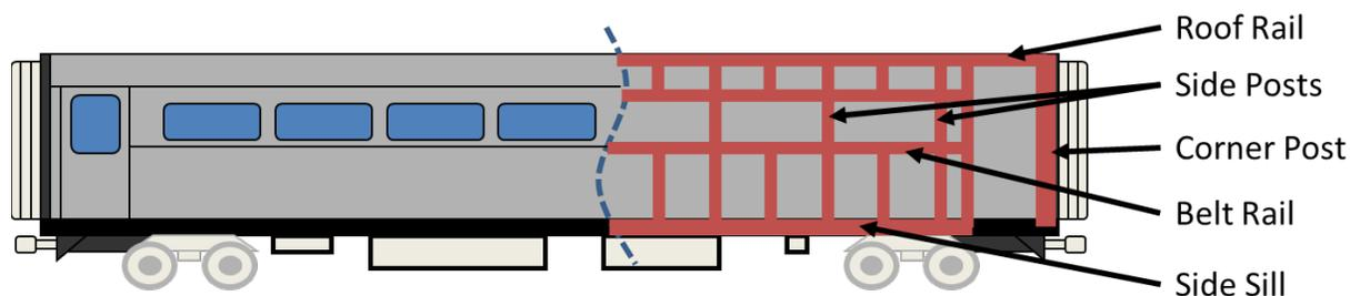
**Figure 2. Schematic of Structural Members in Sidewall of Single-level Passenger Car**
