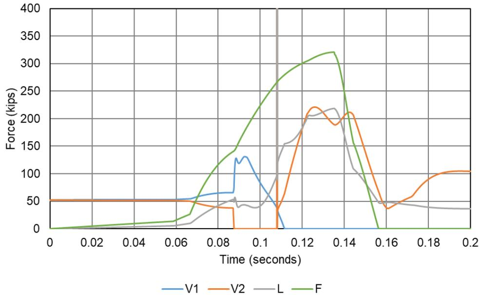
**Figure 38. Rail Reaction Forces and Impact Force versus Time at 5 mph**
