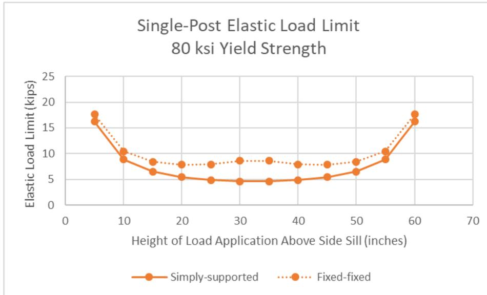
**Figure 28. Elastic Load Limit versus Height of Applied Load above Side Sill for Simply Supported and Fixed-fixed Sidewall Post (load on one post, 80 ksi yield)**
