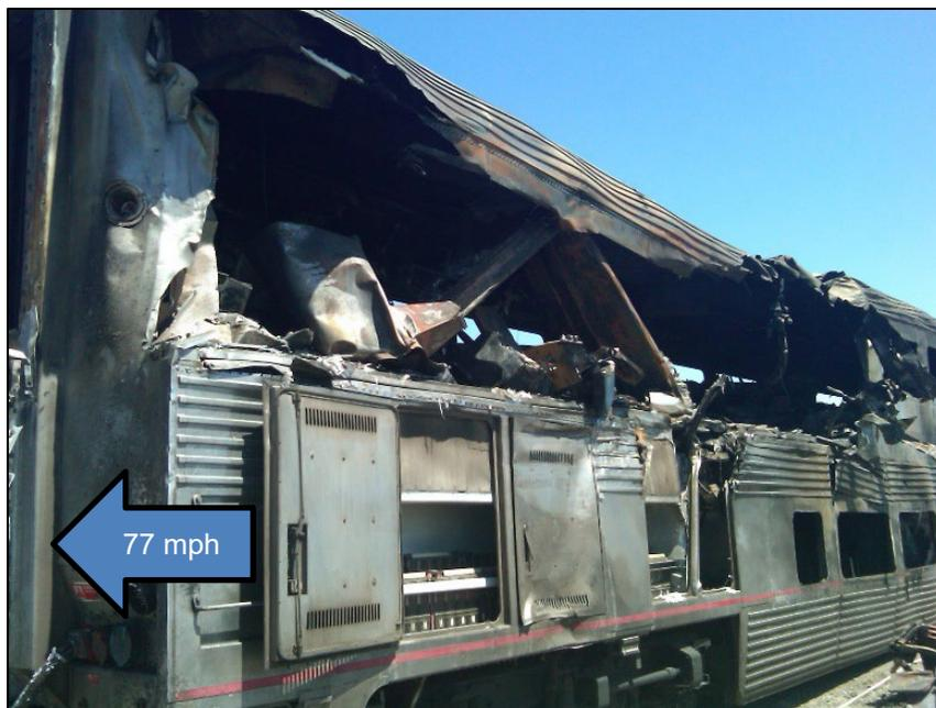
**Figure 10. Coach Car 34033 from Miriam, NV, Accident Showing Damage from Highway Trailer (FRA Photo)**
