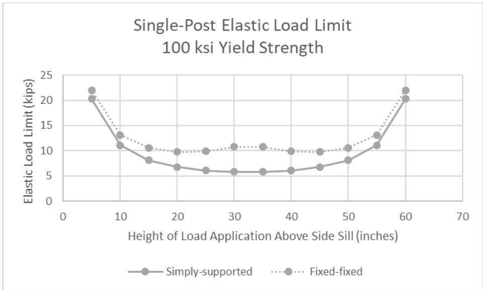
**Figure 30. Elastic Load Limit versus Height of Applied Load above Side Sill for Simply Supported and Fixed-fixed Sidewall Post (load on one post, 100 ksi yield)**
