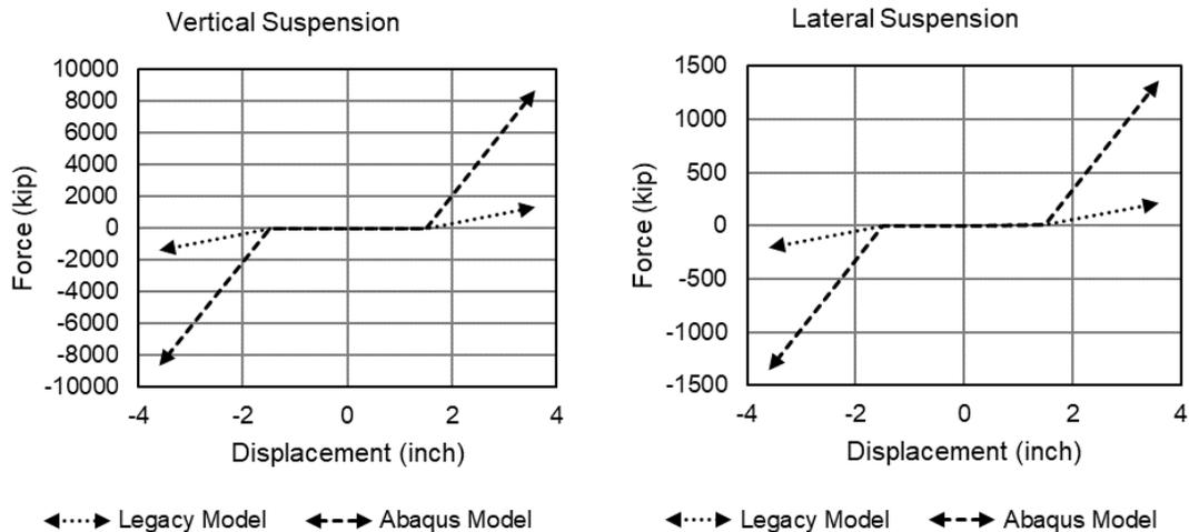
**Figure 36. Railcar Vertical and Lateral Suspension Behaviors**
