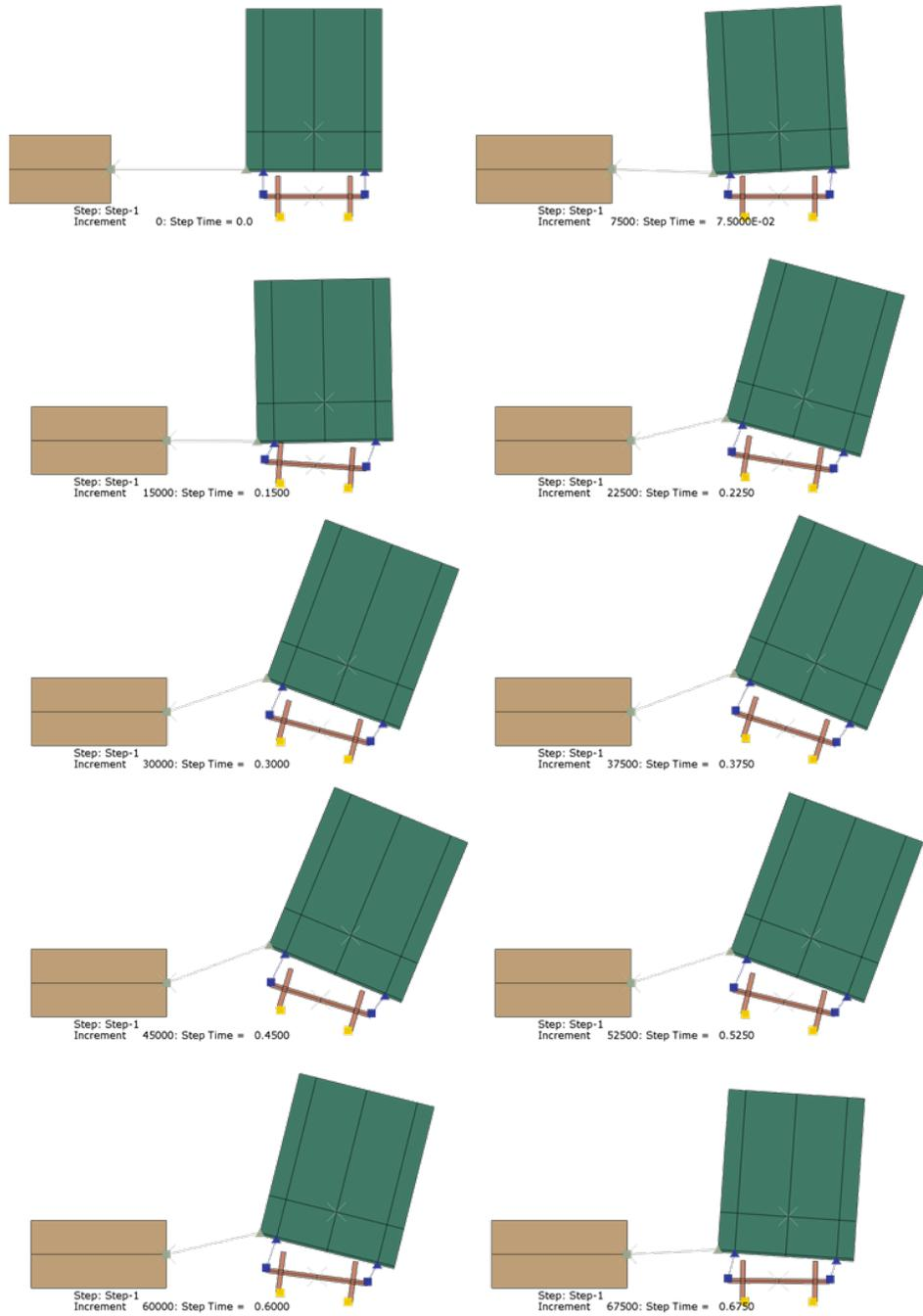
**Figure 37. Impact Sequence at 5 mph (5x displacement scale factor)**
