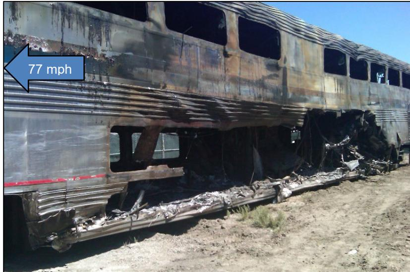
**Figure 9. Sleeper Car 39013 from Miriam, NV, Accident Showing Damage from Highway Tractor Unit (FRA Photo)**
