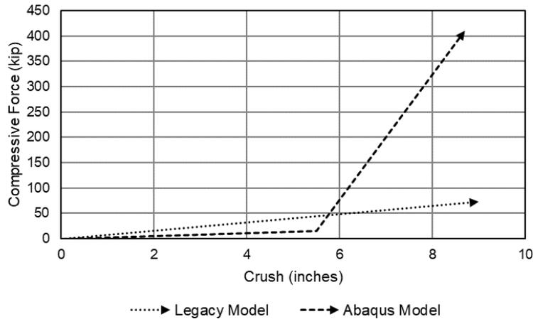
**Figure 35. Highway Vehicle Compressive Force versus Crush Behavior**
