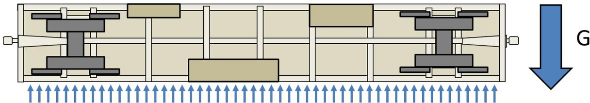
Figure 4. Schematic of Rollover Load Case, Carbody-on-Side
