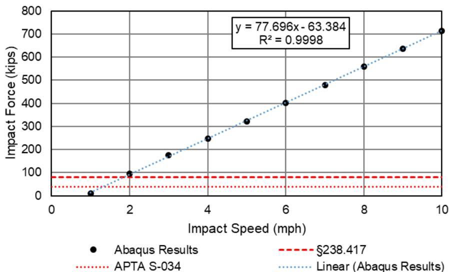
**Figure 39. Impact Force (F) versus Speed**
