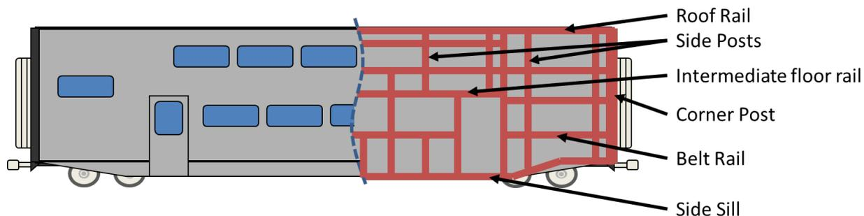
**Figure 3. Schematic of Structural Members in Side Wall of Multi-level Passenger Car**
