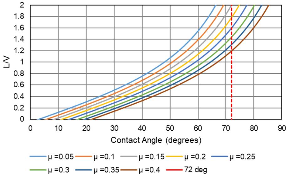
Figure 42. Nadal Formula for Various Coefficients of Friction
