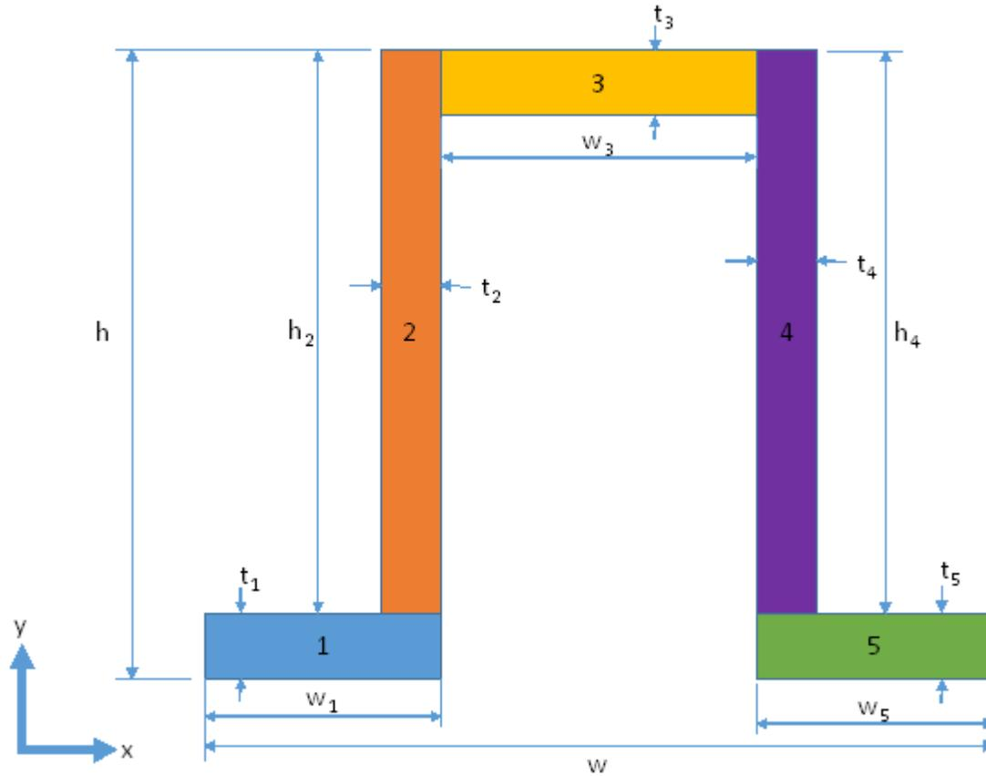
Figure B1. Generalized Sidewall Post Cross-section
