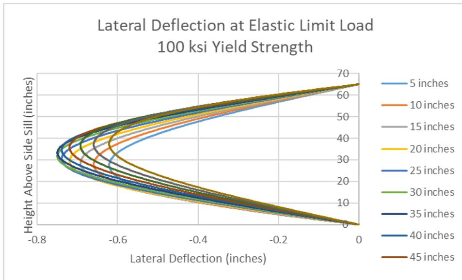
**Figure 22. Lateral Deflection at Elastic Load Limit for Varied Load Heights (single post, simply supported at ends, 100 ksi yield strength)**
