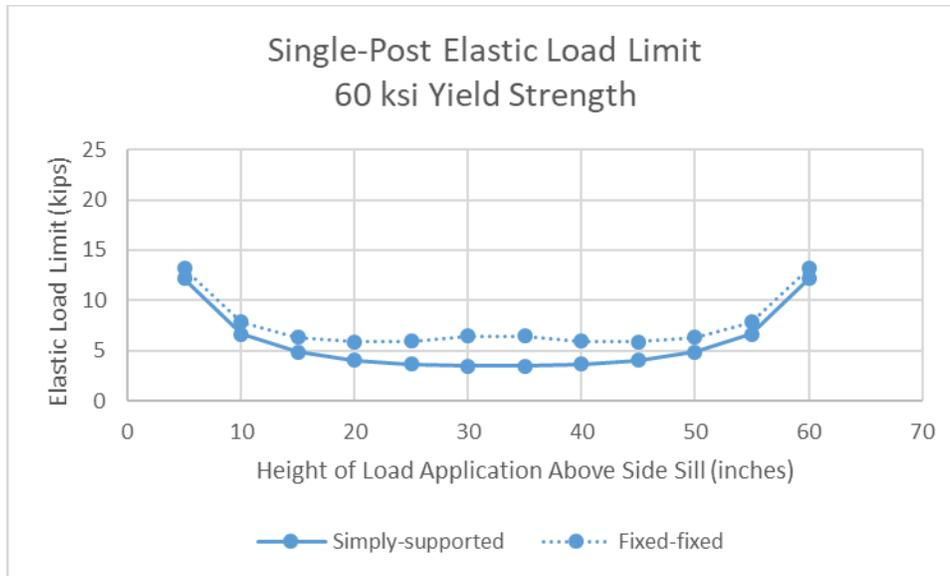
**Figure 26. Elastic Load Limit versus Height of Applied Load above Side Sill for Simply Supported and Fixed-fixed Sidewall Post (load on one post, 60 ksi yield)**
