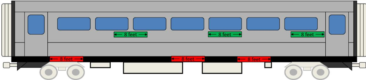
**Figure 5. Schematic of 8-ft Side Sill and Belt Rail Loads, Showing Multiple Loading Positions**
