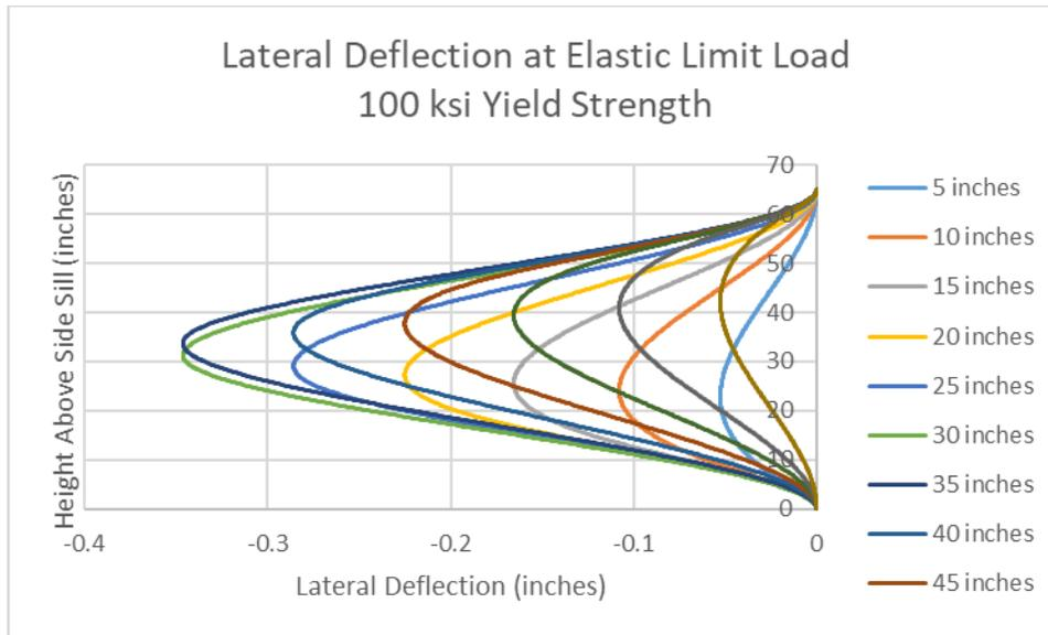
**Figure 25. Lateral Deflection at Elastic Load Limit for Varied Load Heights
