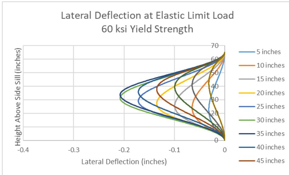
**Figure 23. Lateral Deflection at Elastic Load Limit for Varied Load Heights (single post, fixed at ends, 60 ksi yield strength)**
