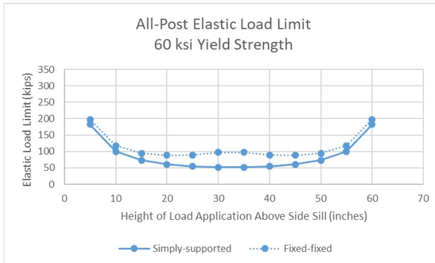
**Figure 27. Elastic Load Limit versus Height of Applied Load above Side Sill for Simply Supported and Fixed-fixed Sidewall Post (load shared across all posts, 60 ksi yield)**
