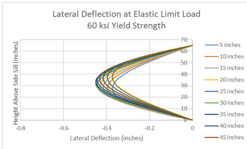
**Figure 20. Lateral Deflection at Elastic Load Limit for Varied Load Heights (single post, simply supported at ends, 60 ksi yield strength)**
