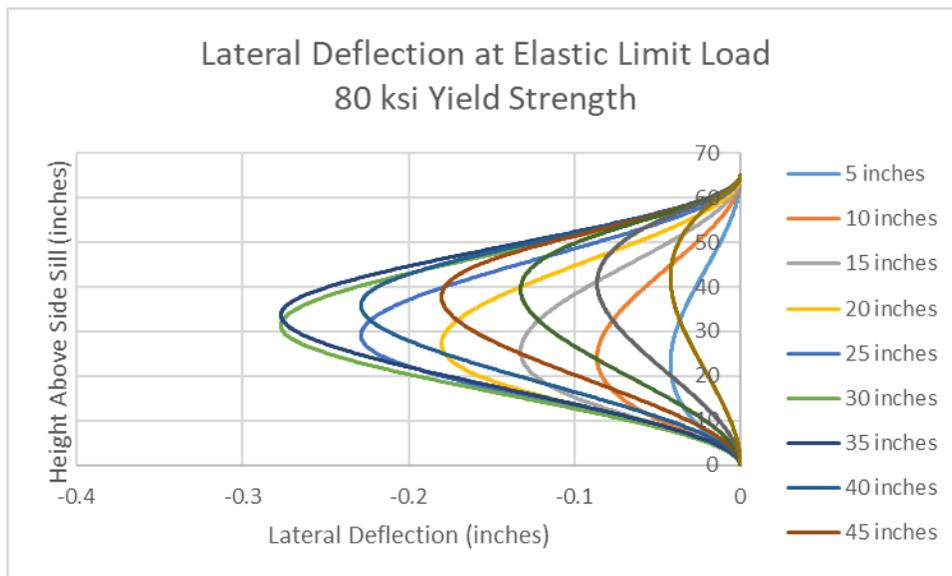
**Figure 24. Lateral Deflection at Elastic Load Limit for Varied Load Heights (single post, fixed at ends, 80 ksi yield strength)**
