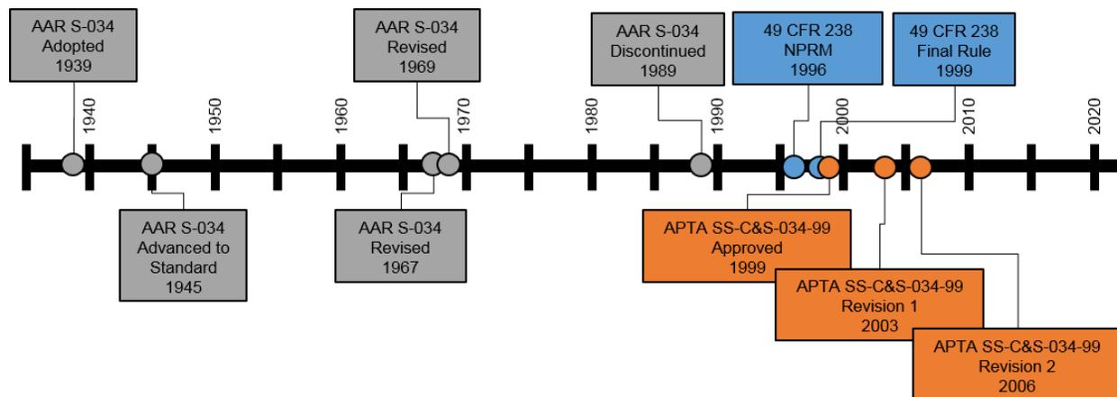
**Figure 1. Timeline of Standards and Regulations Applicable to U.S. Cars that Include Side Structure Criteria**
