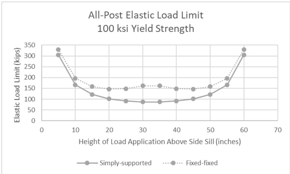
**Figure 31. Elastic Load Limit versus Height of Applied Load above Side Sill for Simply Supported and Fixed-fixed Sidewall Post (load shared across all posts, 100 ksi yield)**
