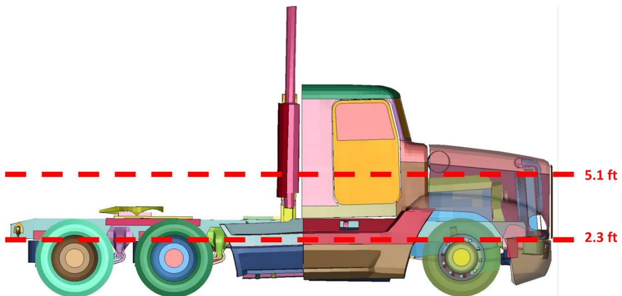
**Figure 16. Annotated Semi-tractor Model with 194-inch Wheelbase [29]**
