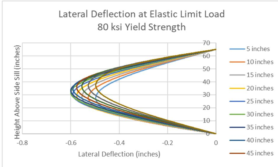
**Figure 21. Lateral Deflection at Elastic Load Limit for Varied Load Heights (single post, simply supported at ends, 80 ksi yield strength)**
