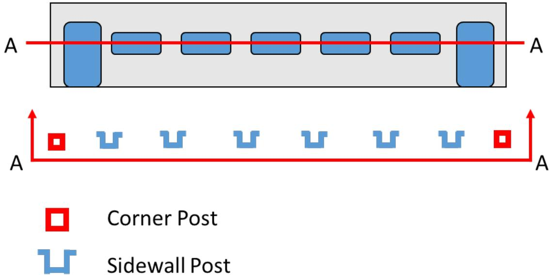
**Figure 18. Generalized Conventional Passenger Railcar Sidewall Post Arrangement**
