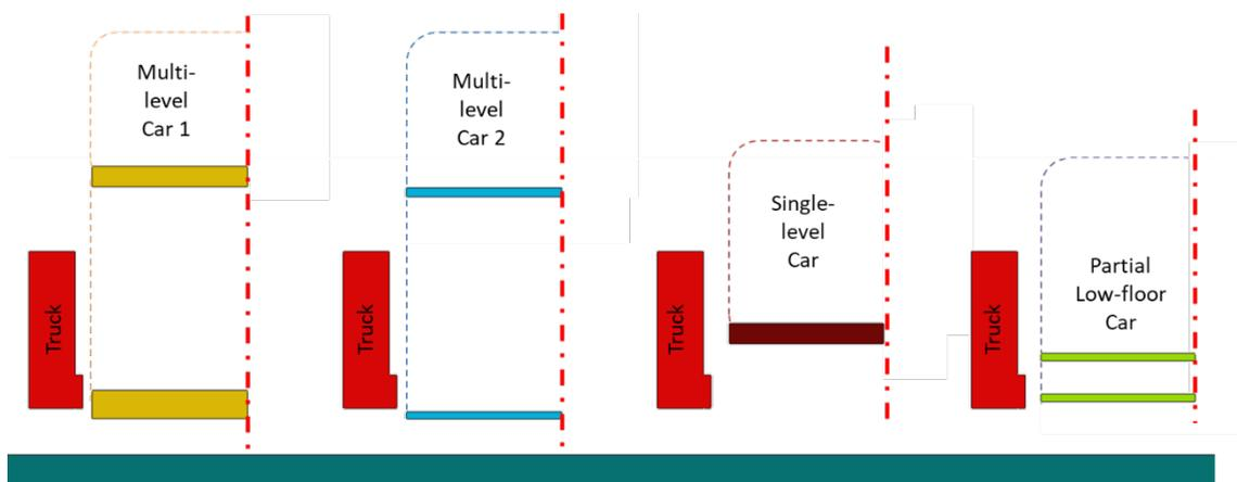
**Figure 15. Approximate Floor Heights and Heavy-duty Truck Front-End Height**
