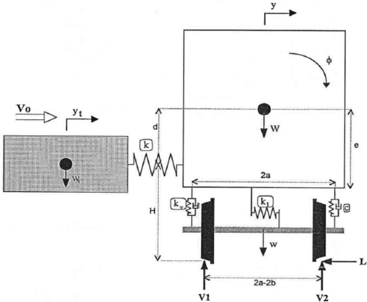
**Figure 32. Highway Vehicle Side Impact Model**
