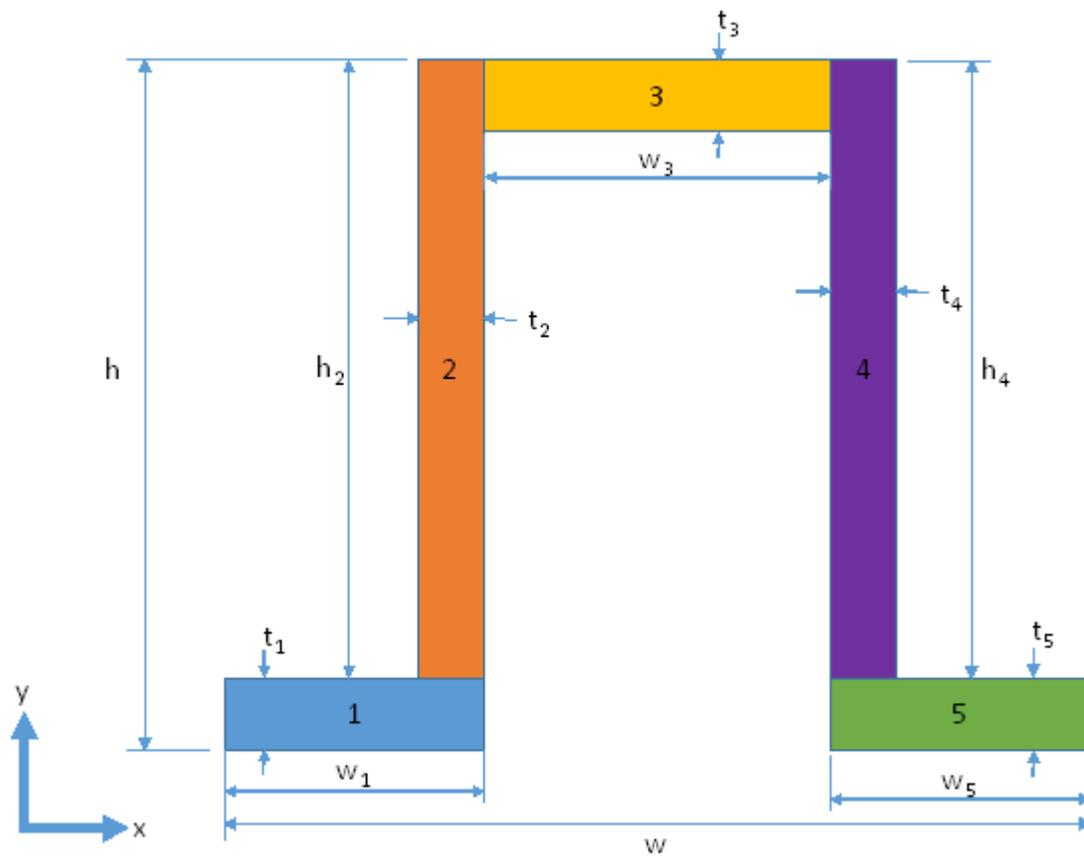
**Figure 19. Beam Profile for Sidewall Posts Used in Calculations**
