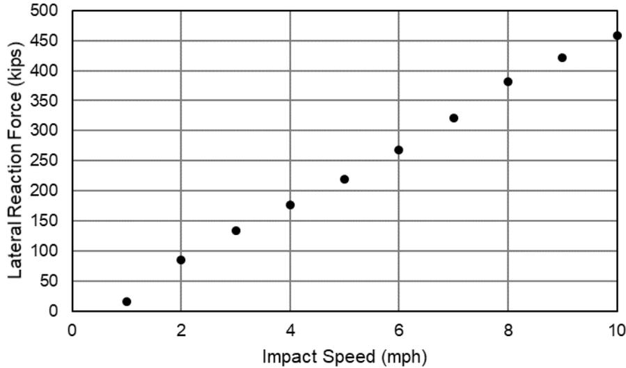
**Figure 40. Lateral Reaction Force (L) versus Speed**
