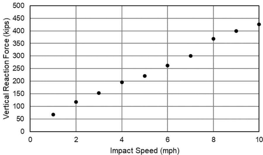
**Figure 41. Vertical Reaction Force (V<sub>2</sub>) versus Speed**
