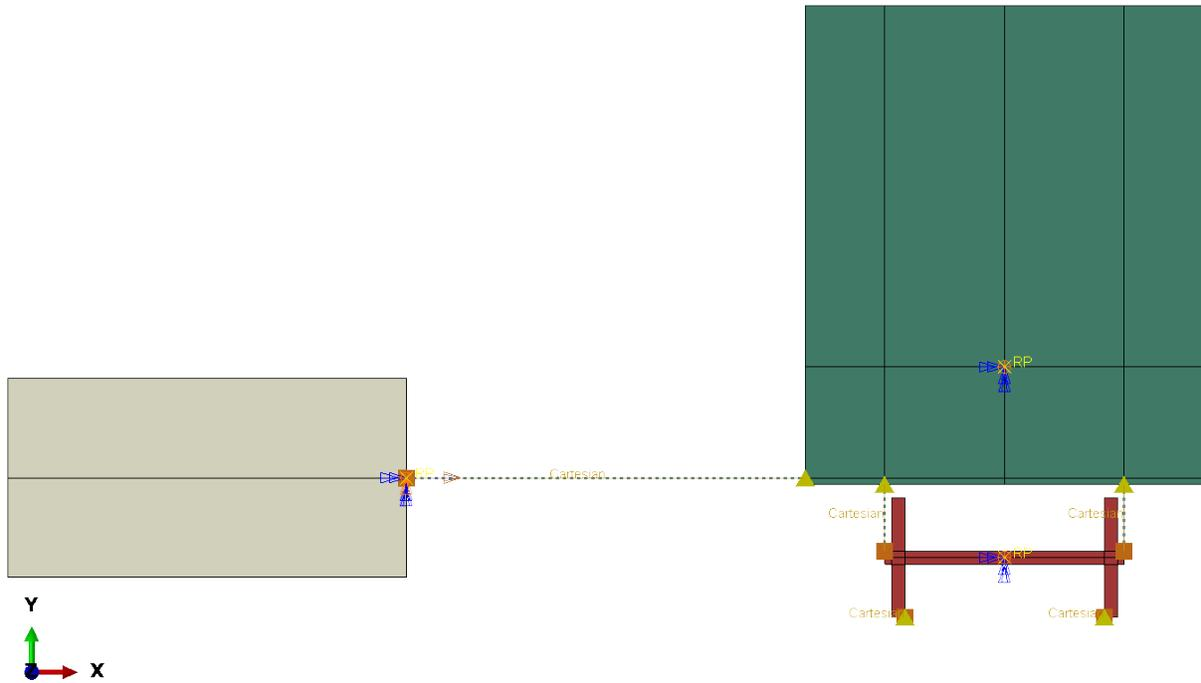
**Figure 33. Simplified 2D Rollover Model in Abaqus/Explicit**
