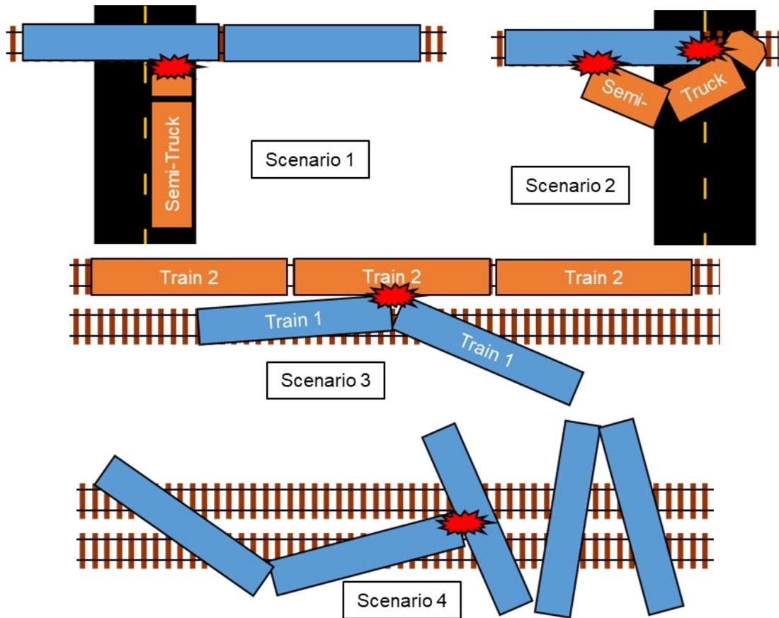
**Figure 14. Side-Impact Scenarios Involving (1) Side Impact from Heavy-duty Truck, (2) Struck Heavy-duty Truck Swinging Around to Impact Side of Passenger Car, (3) Sideswipe (raking) from Other Train, (4) Passenger Car Derailment and Pile-Up**
