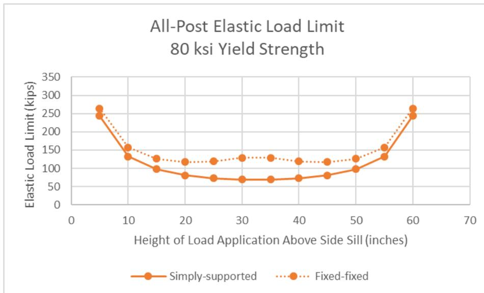
**Figure 29. Elastic Load Limit versus Height of Applied Load above Side Sill for Simply Supported and Fixed-fixed Sidewall Post (load shared across all posts, 80 ksi yield)**
