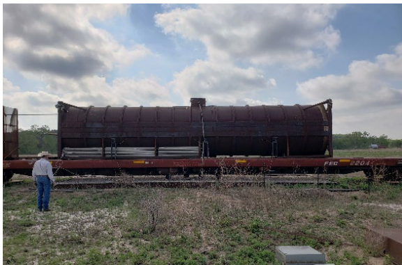
Figure 1. UN-T75 Tank Prior to Fire Test
