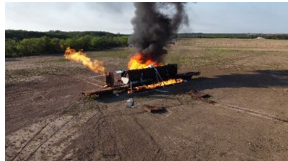
Figure 2. Fire Test in Progress (PRV Venting)
