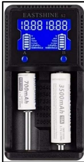
**Figure 32. EASTSHINE cylinder charger**
