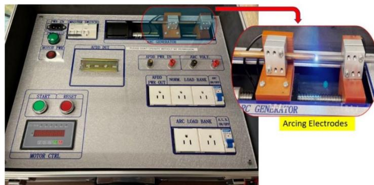
Figure 13. Arc generator with arcing electrodes
