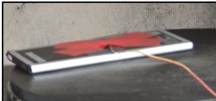
**Figure 33. Pre-heating prism (LCO) placement**
