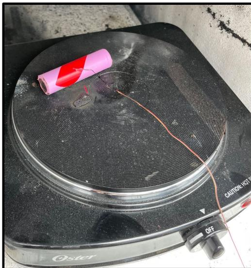
**Figure 34. Standard 18650 cell placement**
