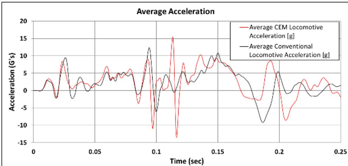
**Figure 44. Longitudinal Average Acceleration**
