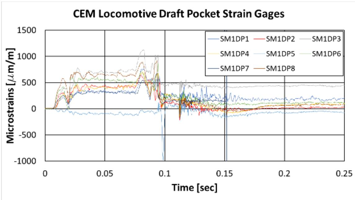
Figure 50. CEM Locomotive Draft Pocket Strain Results
