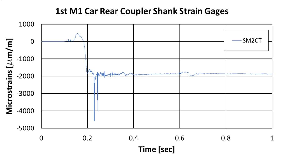
**Figure 58. First M1 Passenger Car Rear Coupler Shank Strain Results**
