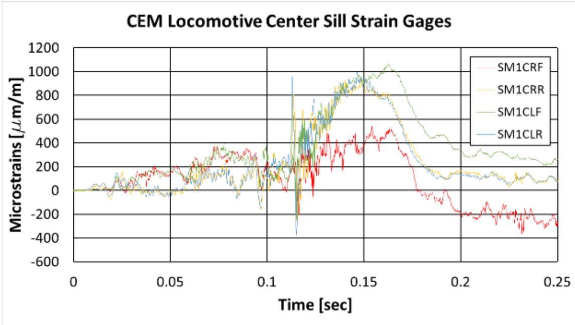
Figure 52. CEM Locomotive Center Sill Strain Results
