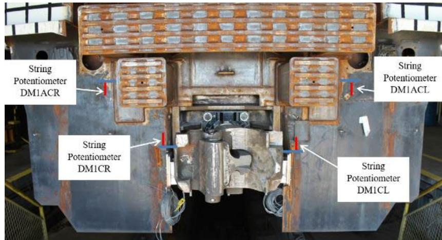
**Figure 8. CEM Locomotive Coupler and Anti-Climber String Potentiometers**
