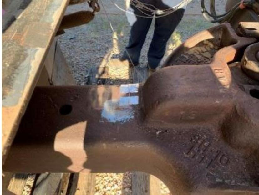
**Figure 25. Strain Gage Location on the First M1 Passenger Car Lead Coupler**
