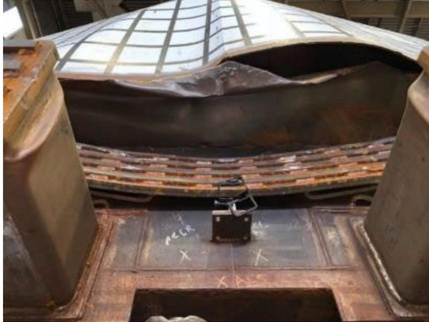
**Figure 101. CEM Locomotive – Deformed Nose**
