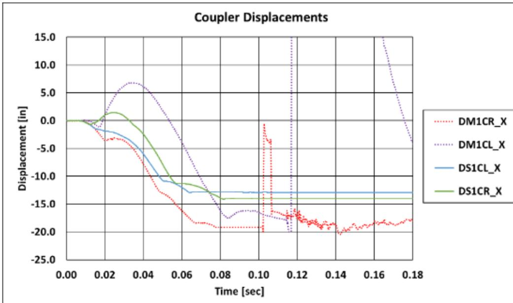
**Figure 45. Impacting Coupler Displacements**
