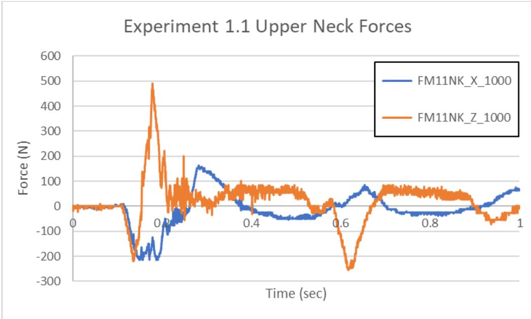
**Figure 86. Occupant Protection Experiment 1.1 Upper Neck Force Data**
