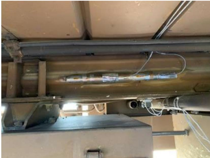
**Figure 24. Strain Gage Locations on the First M1 Passenger Car Center Sill**
