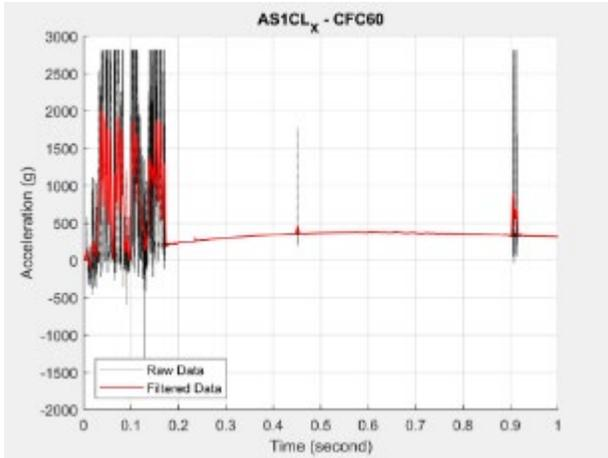
Figure B25. AS1CL\_X Accelerometer Data
