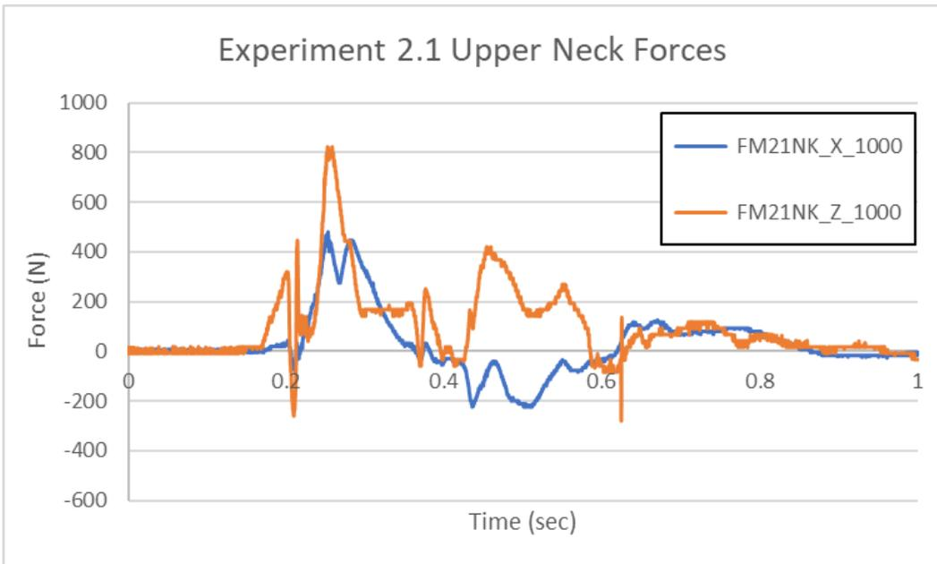
**Figure 87. Occupant Protection Experiment 2.1 Upper Neck Force Data**
