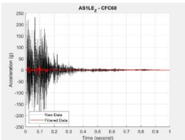
Figure B29. AS1LE\_Z Accelerometer Data
