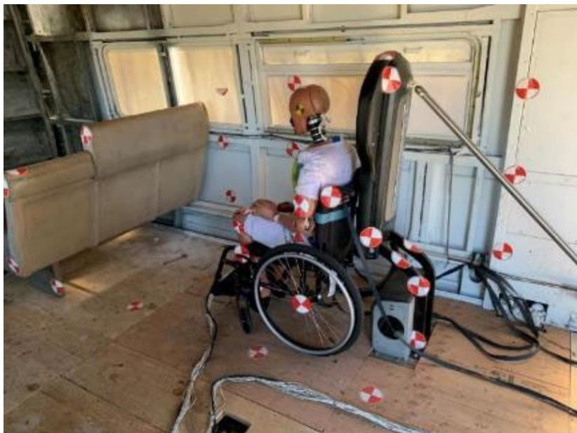
**Figure 118. Post Impact Unrestrained Quantum Backboard**
