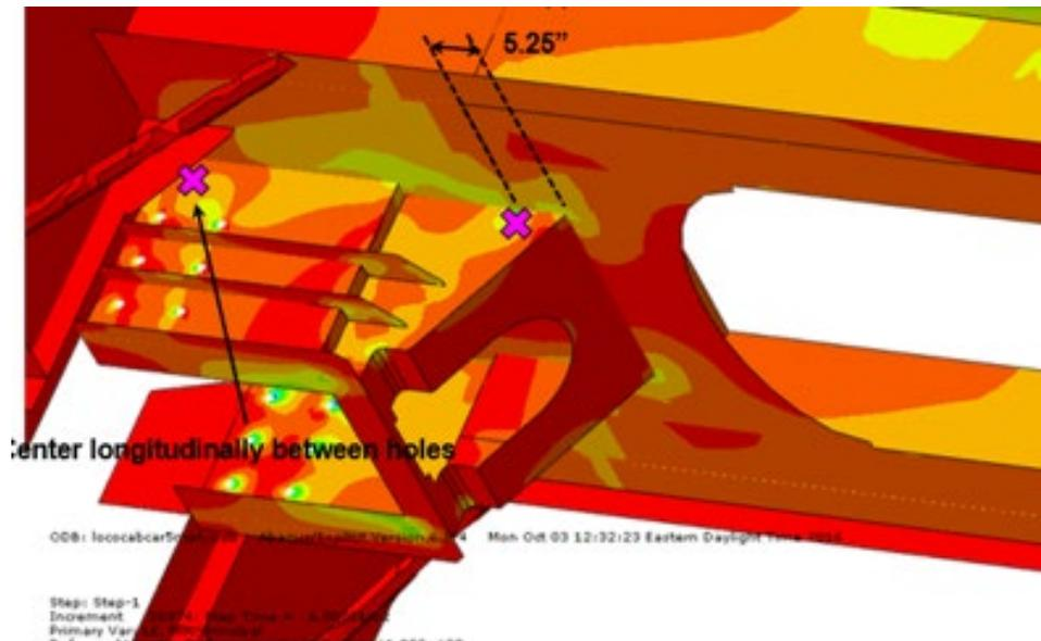
**Figure 16. Strain Gage Locations on CEM Locomotive Draft Pocket**
