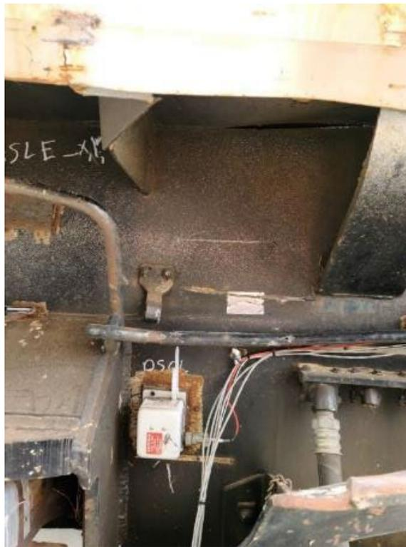
**Figure 111. Buckled Floor Structure and Deformed Front Plate, Left Side**
