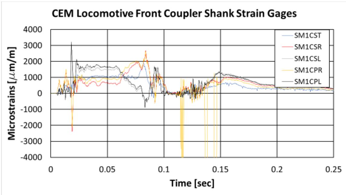
Figure 48. CEM Locomotive Front Coupler Shank Strain Results
