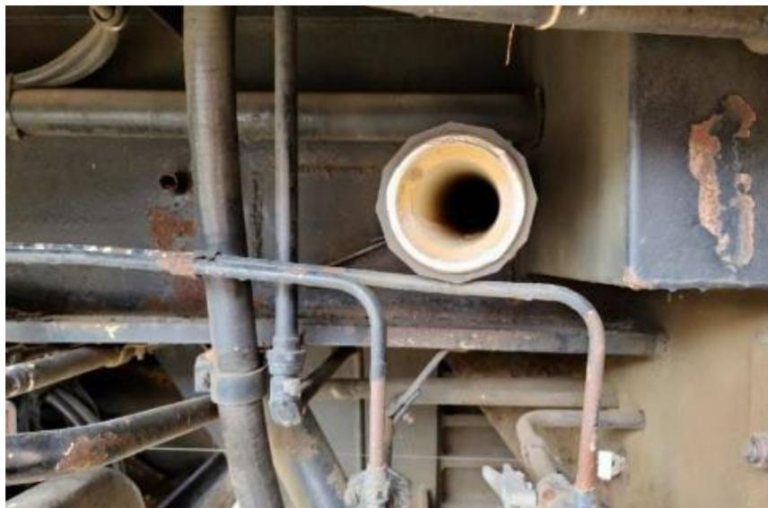
**Figure 112. Downward Curve in Conventional Locomotive Center Sill Flange**
