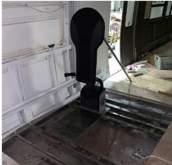
**Figure 36. Quantum Backboard Restraint Device**
