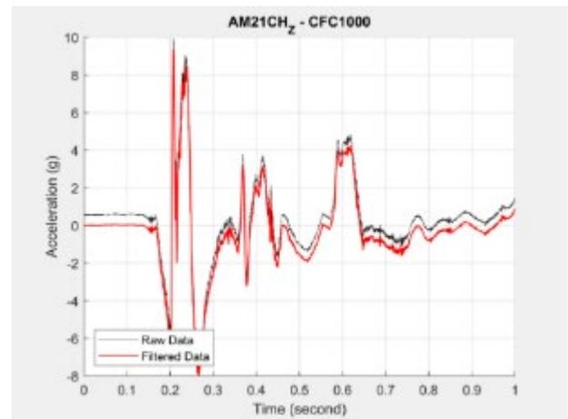
**Figure B106. AM21CH\_Z-CFC1000 Accelerometer Data**
