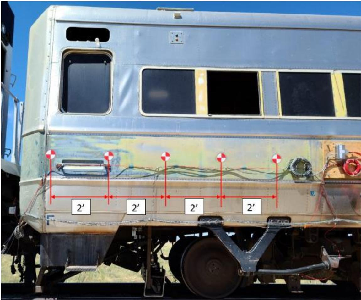
**Figure A3. Target Spacing for 8332 M1 Car**
