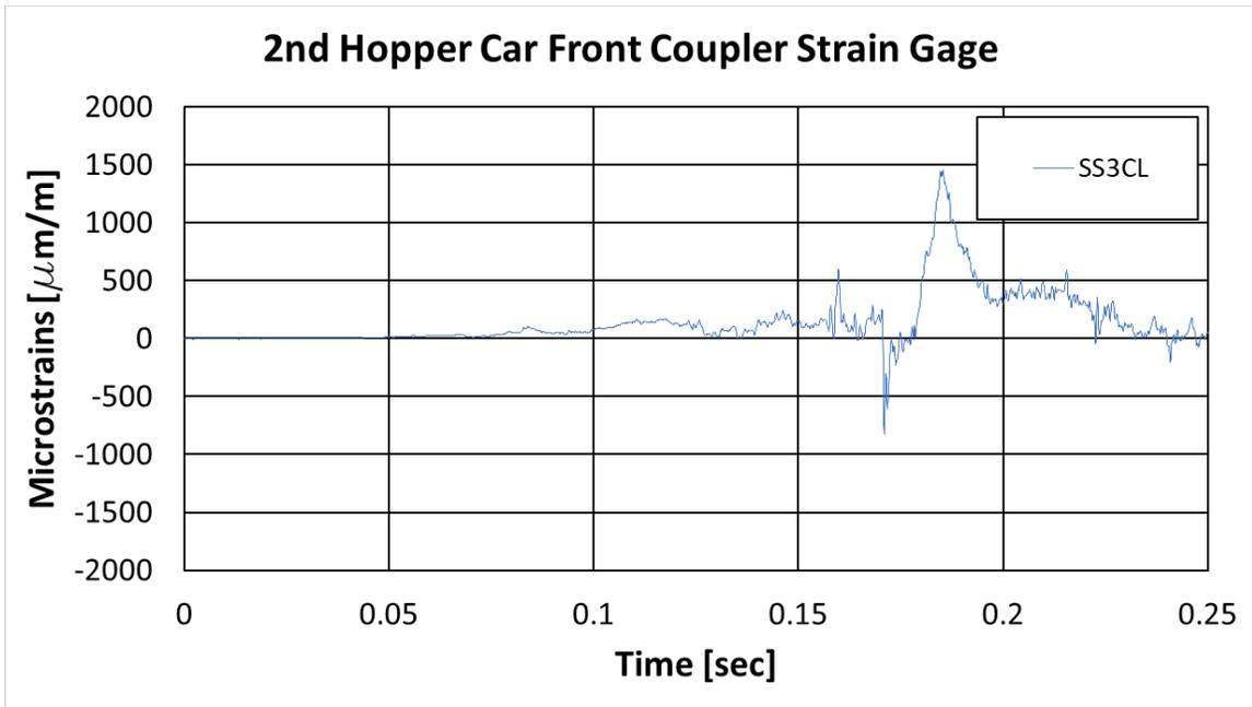
**Figure 66. 2nd Hopper Car Front Coupler Shank Strain Results**
