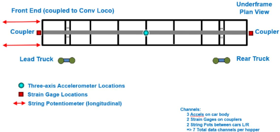
**Figure 34. First Hopper Car Instrumentation**
