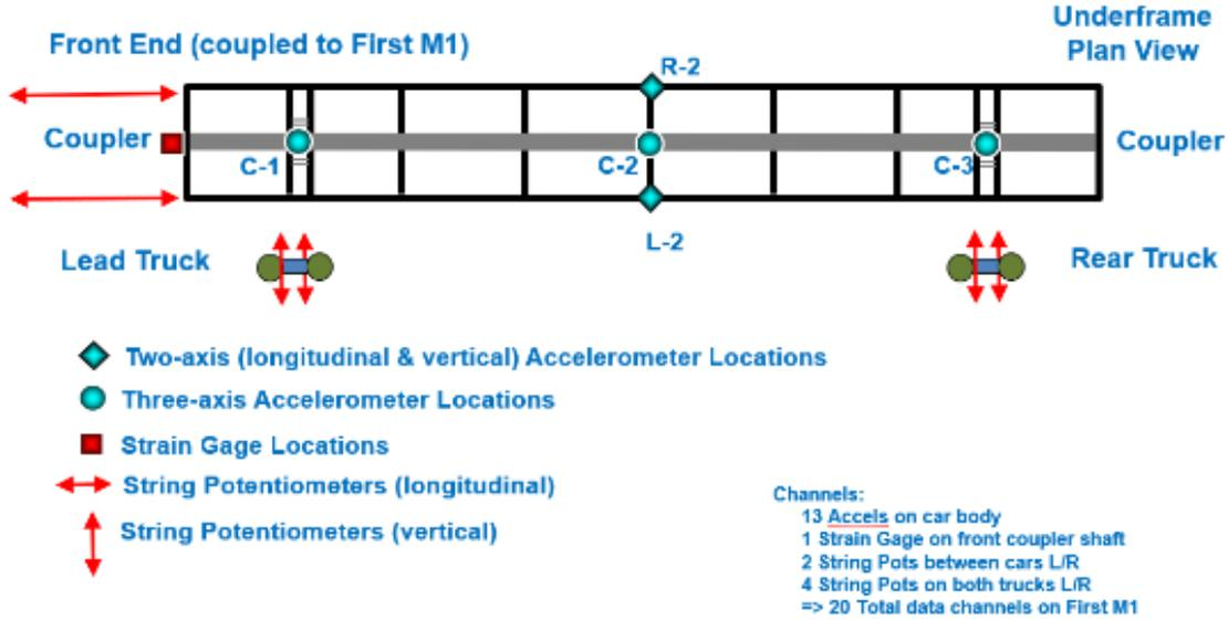
Figure 26. Second M1 Car Instrumentation
