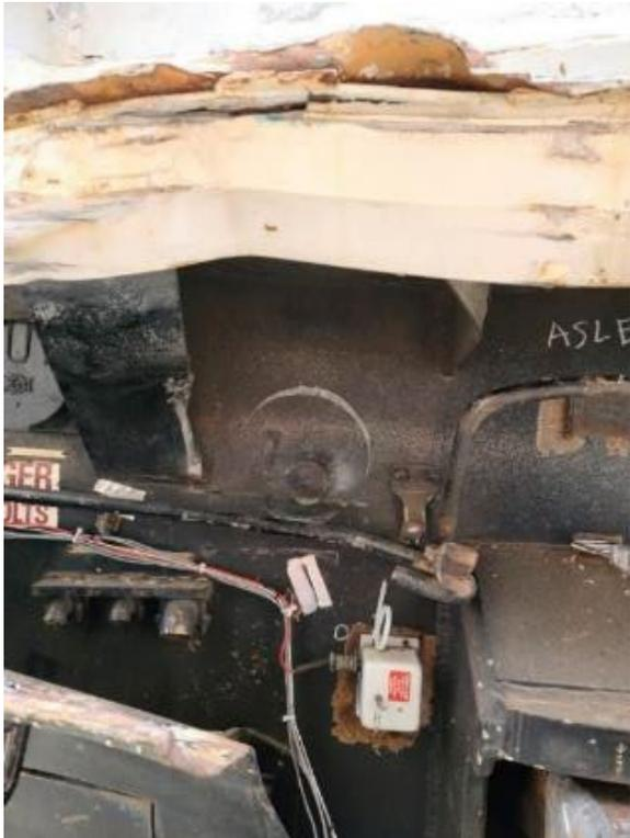
**Figure 110. Buckled Floor Structure and Deformed Front Plate, Right Side**
