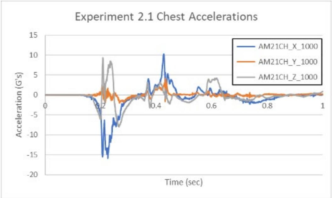
**Figure 76. Occupant Protection Experiment 2.1 Chest Acceleration Data**
