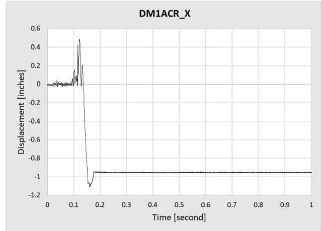
**Figure B56. DM1ACR\_X Displacement Data**
