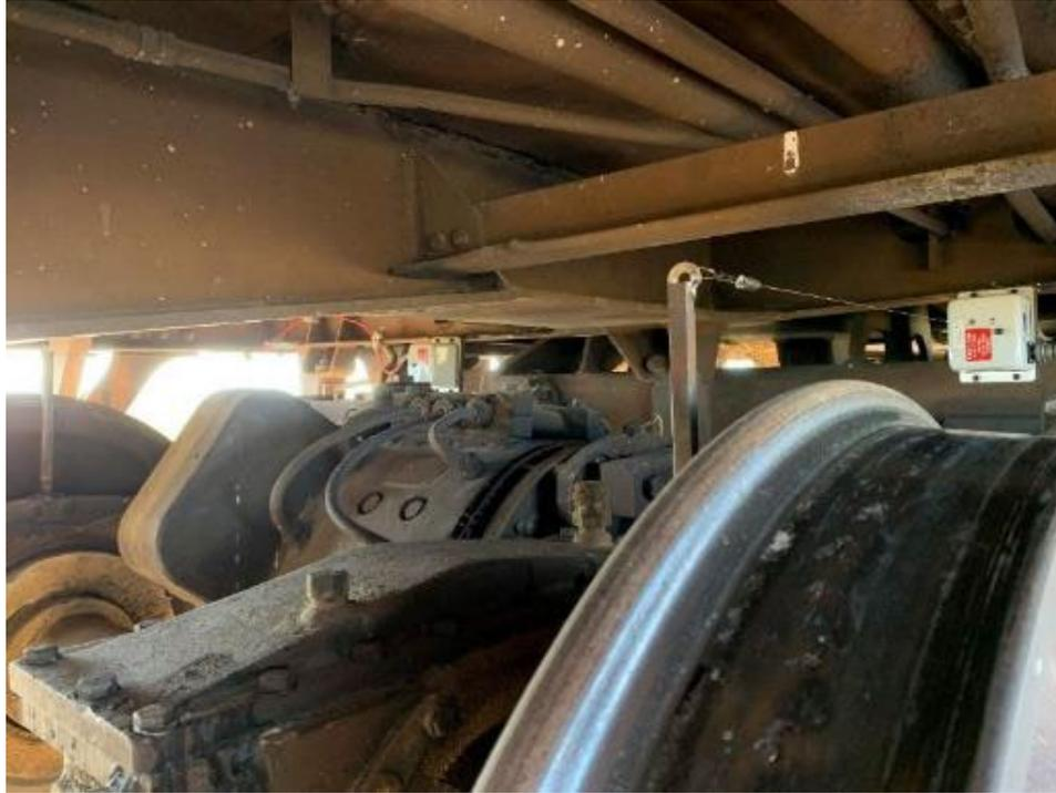
**Figure 22. First M1 Passenger Car Lead Truck to Bolster String Potentiometers**
