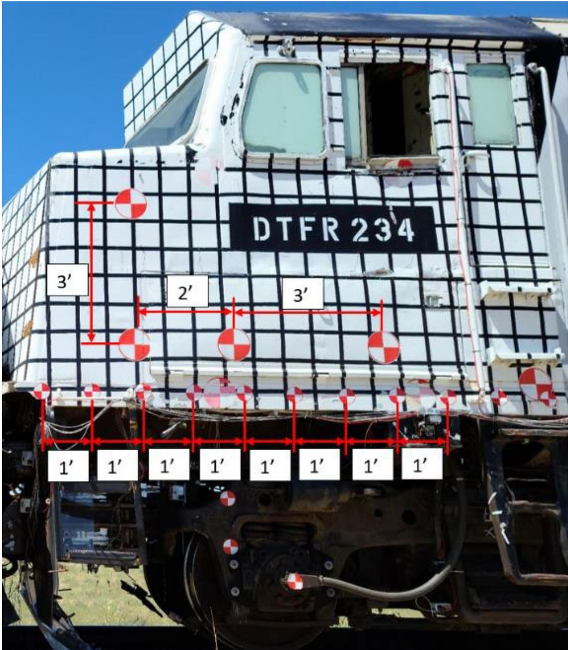
Figure A1. Target Spacing for CEM Locomotive
