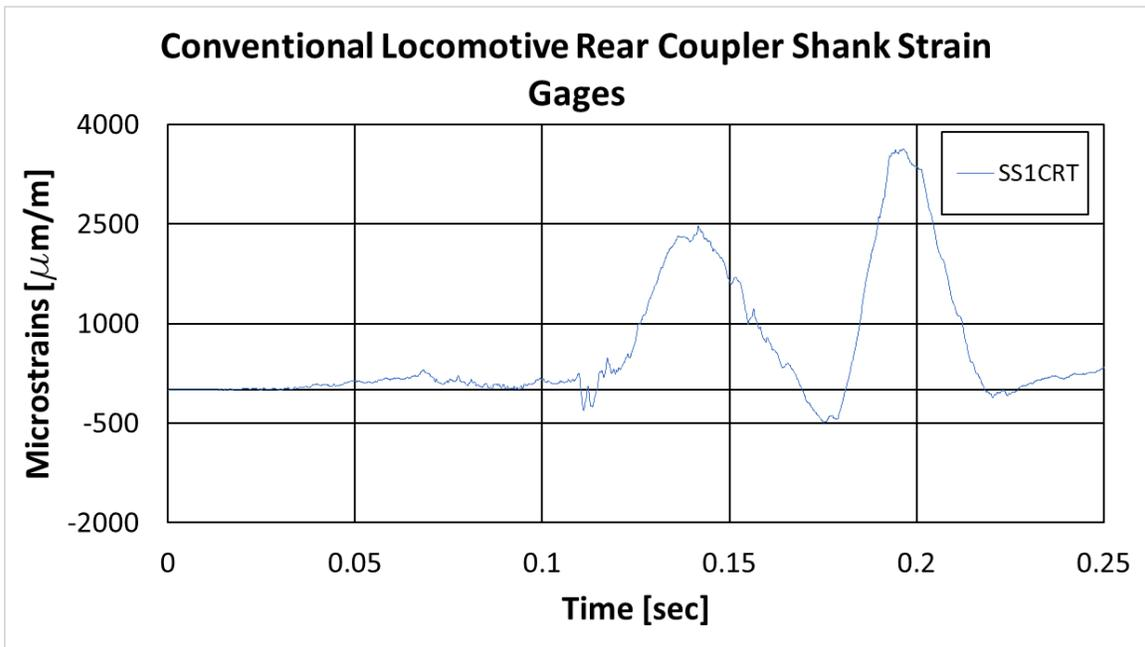
**Figure 63. Conventional Locomotive Rear Coupler Shank Strain Results**
