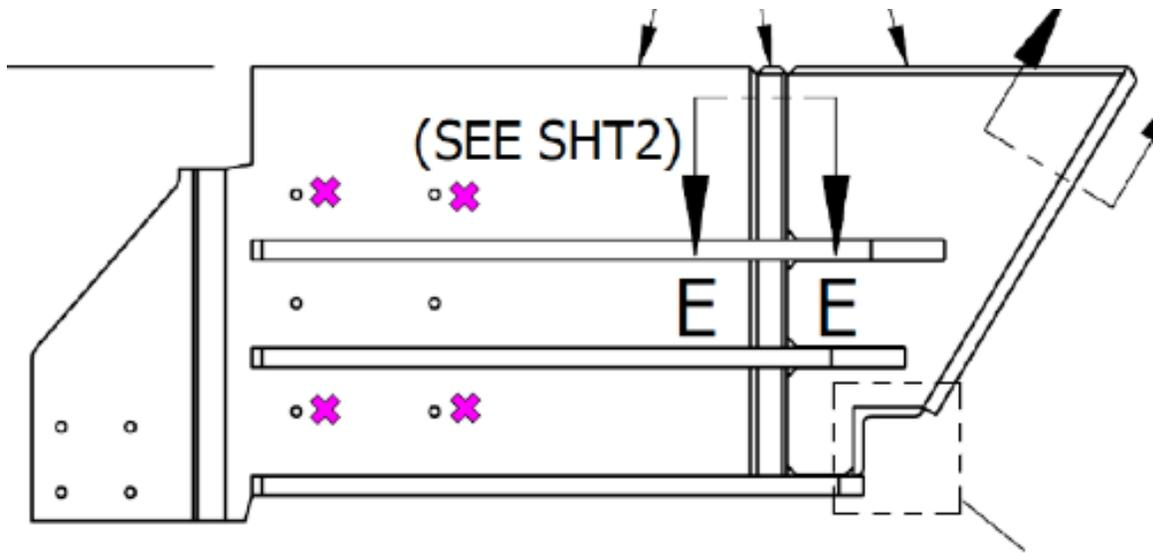
**Figure 15. Strain Gage Locations on CEM Locomotive Draft Pocket**
