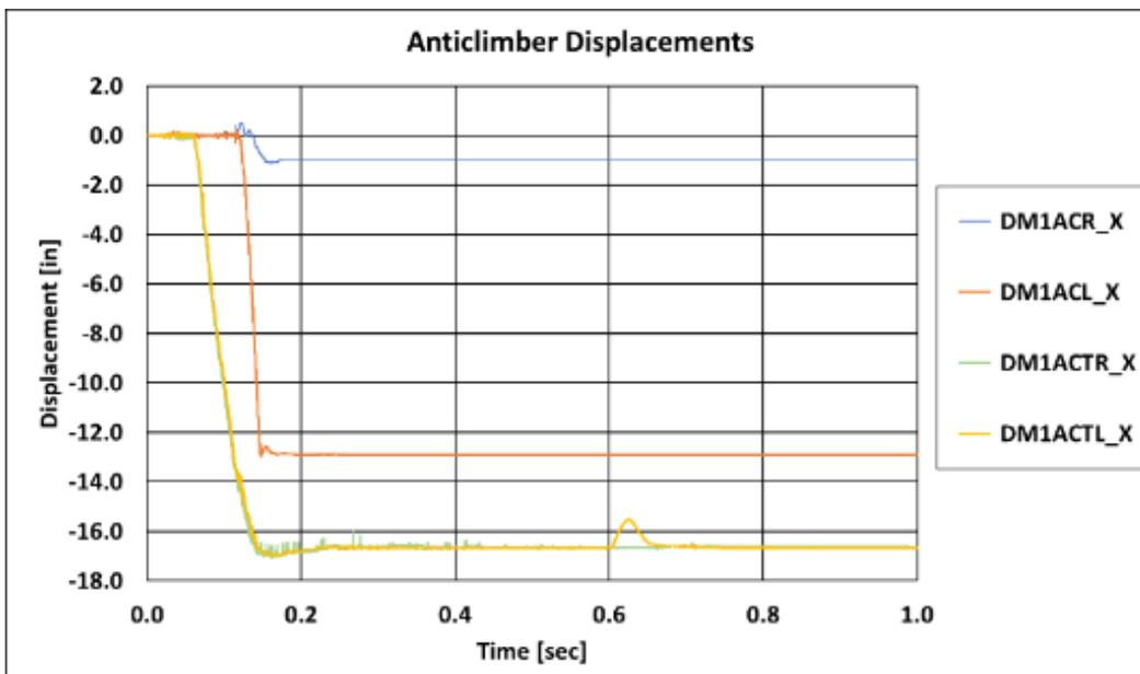
**Figure 46. Anti-climber Displacements**
