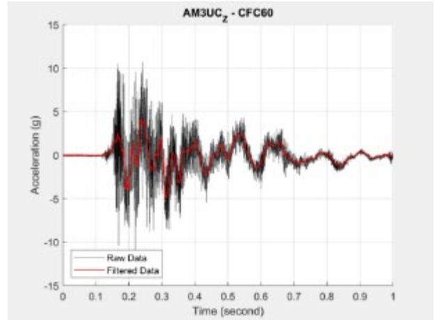
Figure B20. AM3UC\_Z Accelerometer Data
