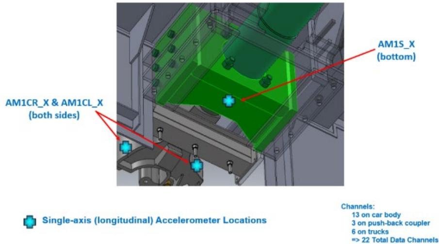
**Figure 5. Locations of Accelerometers on CEM Locomotive Sliding Lug and Pushback Coupler**
