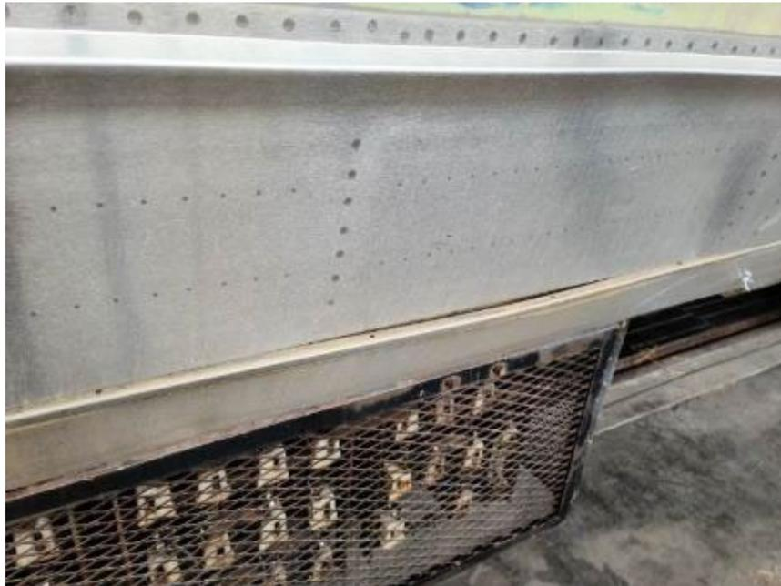
**Figure 115. Side Sill Deformation on the Right Side of 8332**
