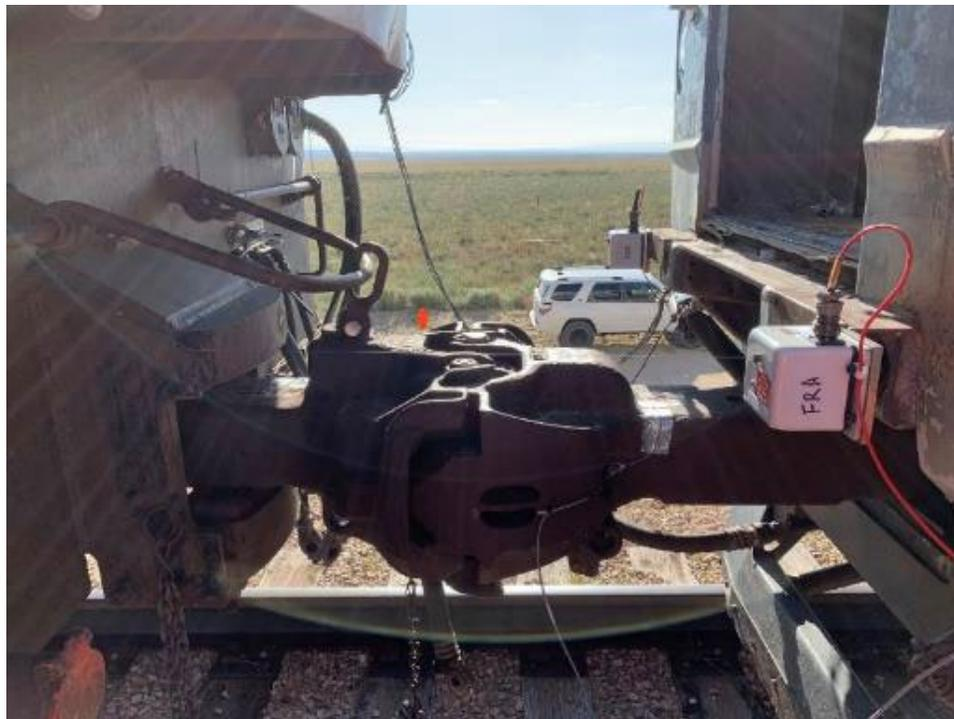
**Figure 21. First M1 Passenger Car Front Coupler String Potentiometers**
