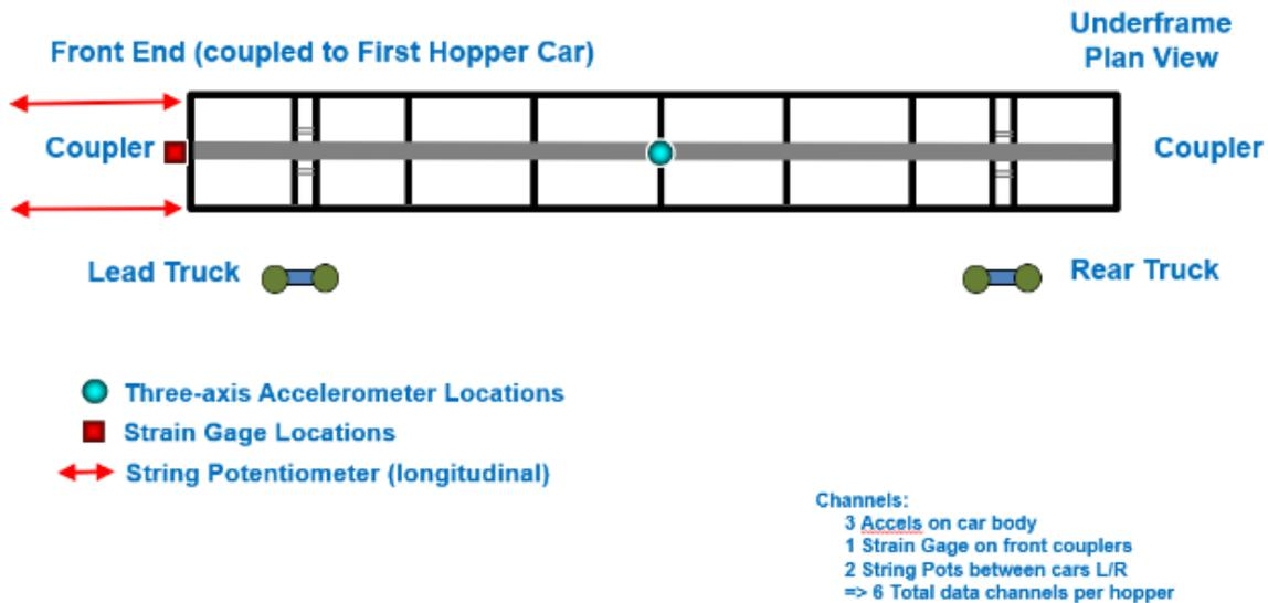
**Figure 35. Second Hopper Car Instrumentation**
