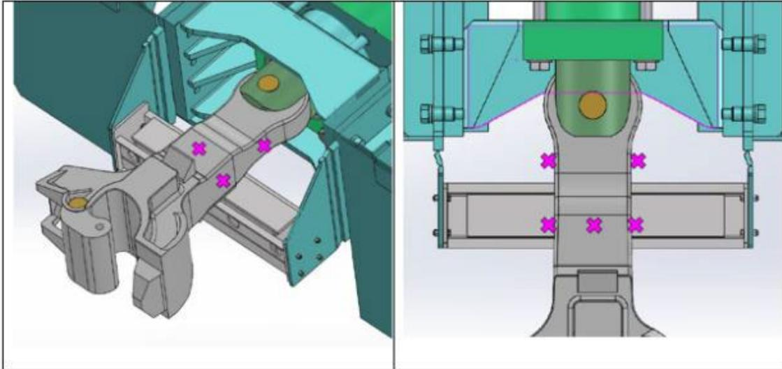
**Figure 13. Strain Gage Locations on CEM Locomotive Coupler Shank**
