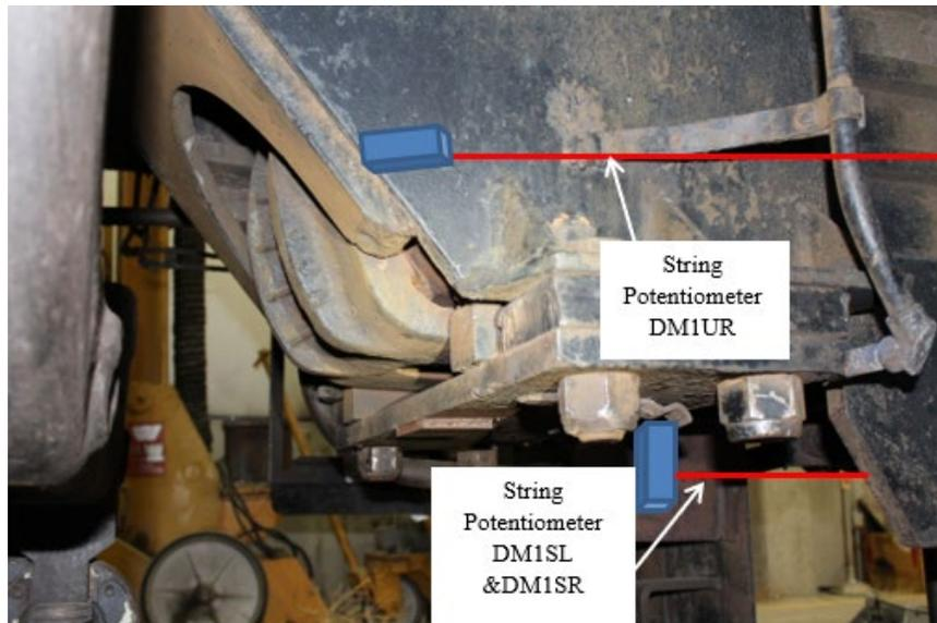
**Figure 11. Right Side CEM Locomotive String Potentiometers**
