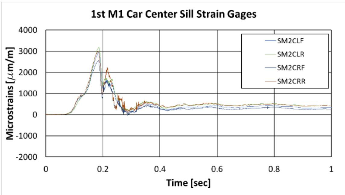
Figure 57. First M1 Passenger Car Center Sill Strain Results
