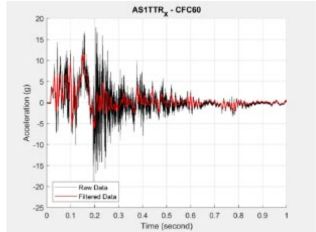
**Figure B38. AS1TTR\_X Accelerometer Data**
