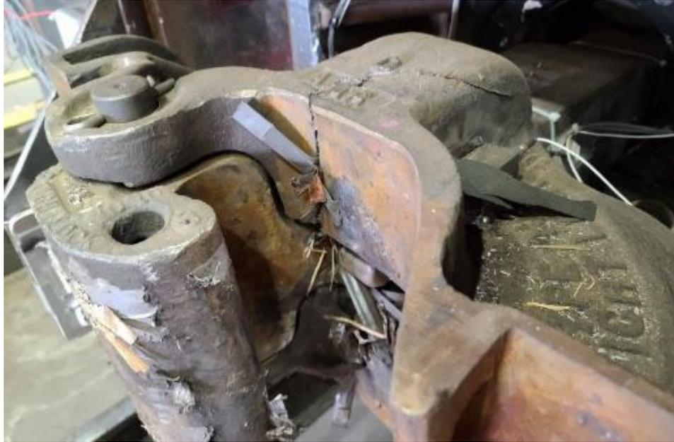
**Figure 99. Crack Along the Front and Top of the PBC Coupler Head**
