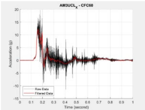
Figure B21. AM3UCL\_X Accelerometer Data<sup>1</sup>
