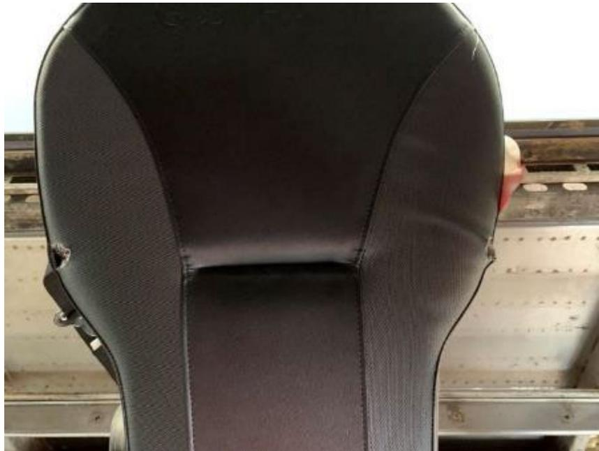
**Figure 120. Holes in the Left and Right Side of the Full Quantum System Backboard**
