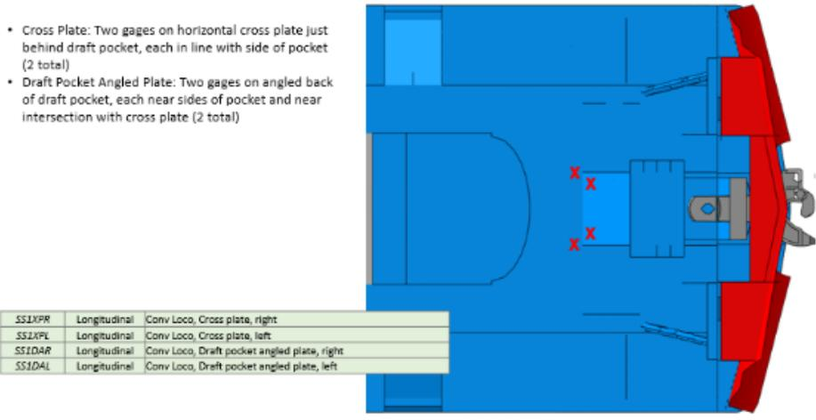
**Figure 32. Strain Gages on the Cross-plate and the Draft Gear Pocket Back Plate**
