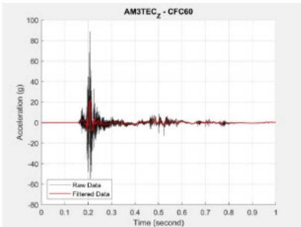
Figure B17. AM3TEC\_Z Accelerometer Data
