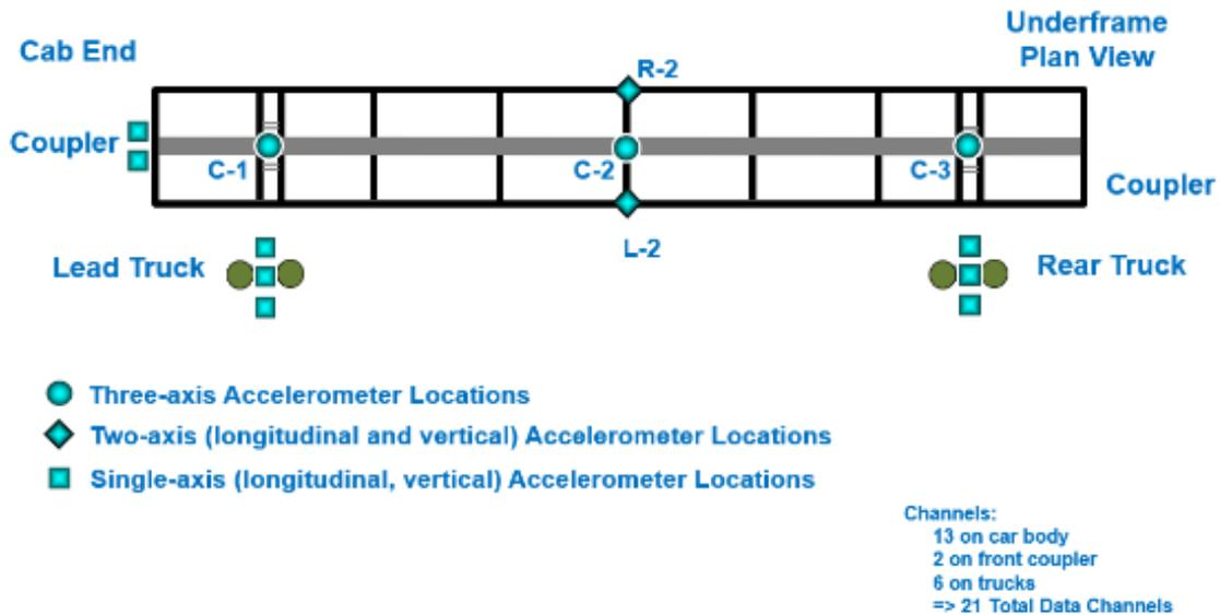
**Figure 30. Accelerometer Locations on Conventional F40 Locomotive**
