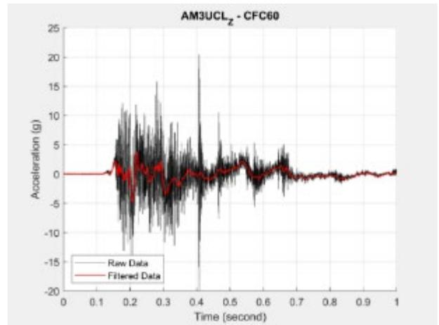
Figure B22. AM3UCL\_Z Accelerometer Data
