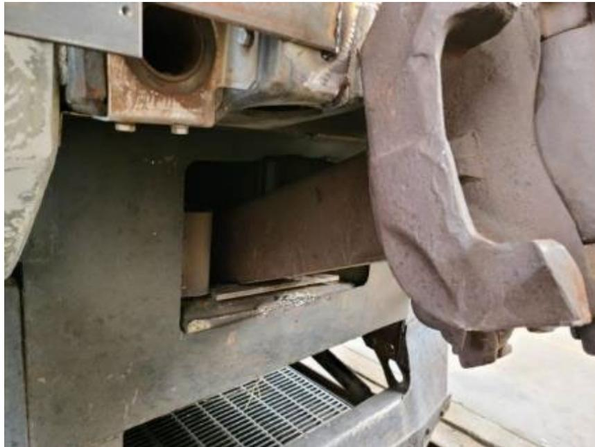
**Figure 114. Shank from Front Coupler on 8332 at Upward Angle**
