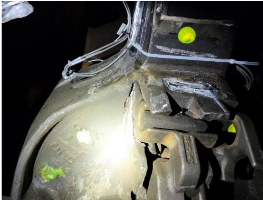
**Figure 98. Crack Along the Bottom of the PBC Coupler Head**
