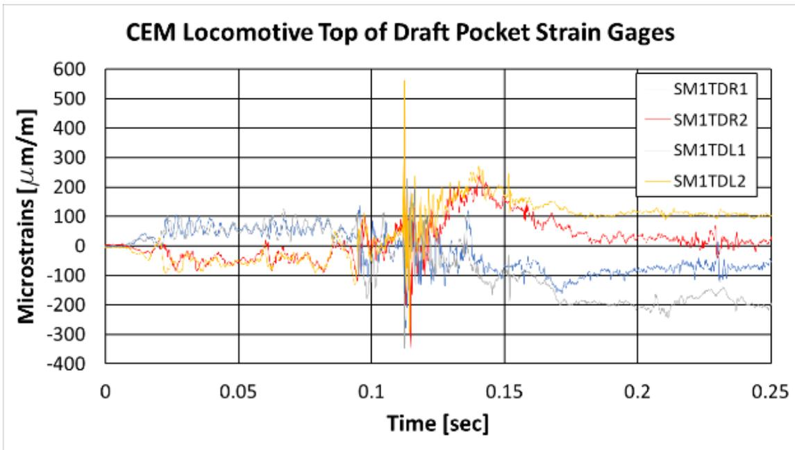
Figure 51. CEM Locomotive Top of Draft Pocket Strain Results
