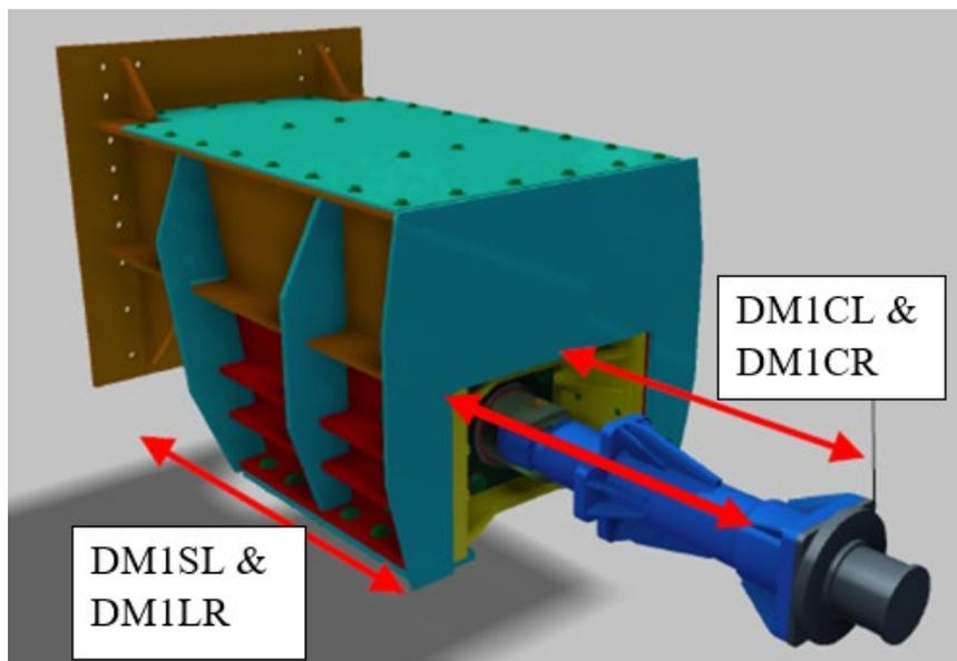
**Figure 12. CEM Locomotive Coupler and Sliding Lug String Potentiometers**
