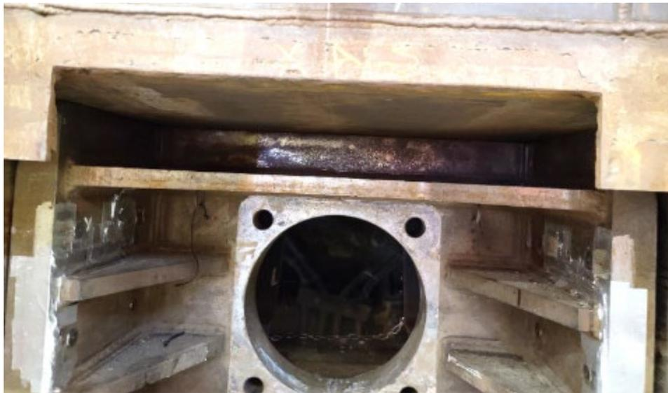
**Figure 108. Contact between the Top of the Sliding Lug and the Top of the Draft Pocket**
