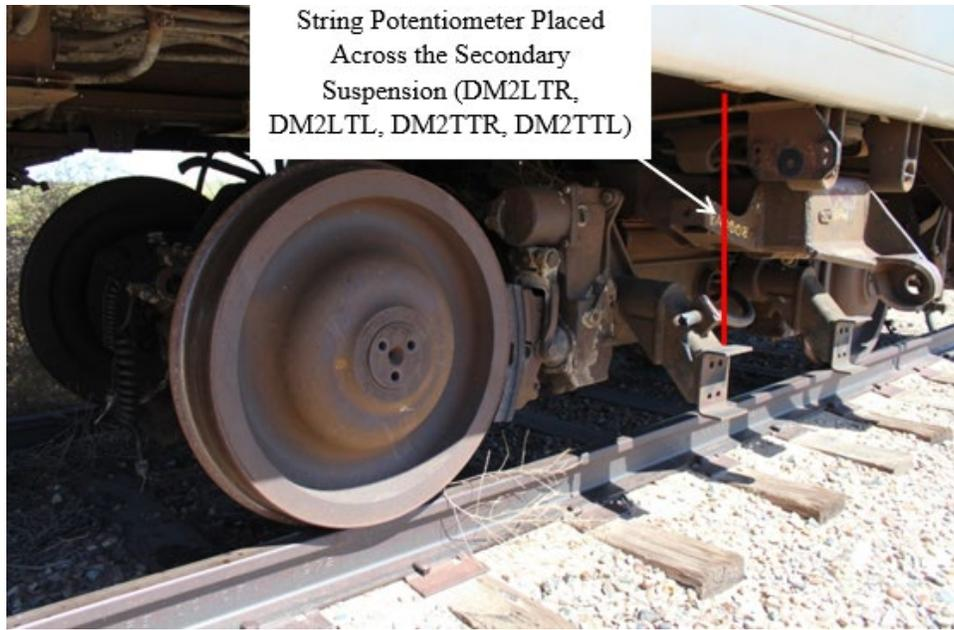
**Figure 20. First M1 Passenger Car Truck Secondary Suspension String Potentiometers**
