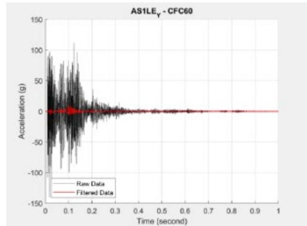
Figure B28. AS1LE\_Y Accelerometer Data
