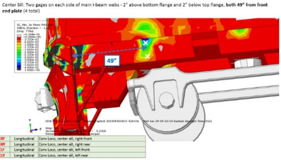
**Figure 33. Strain Gage Locations on the Center Sill**
