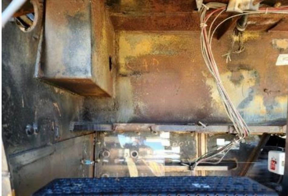
**Figure 107. Curved Center Sill in Front End of CEM Locomotive**
