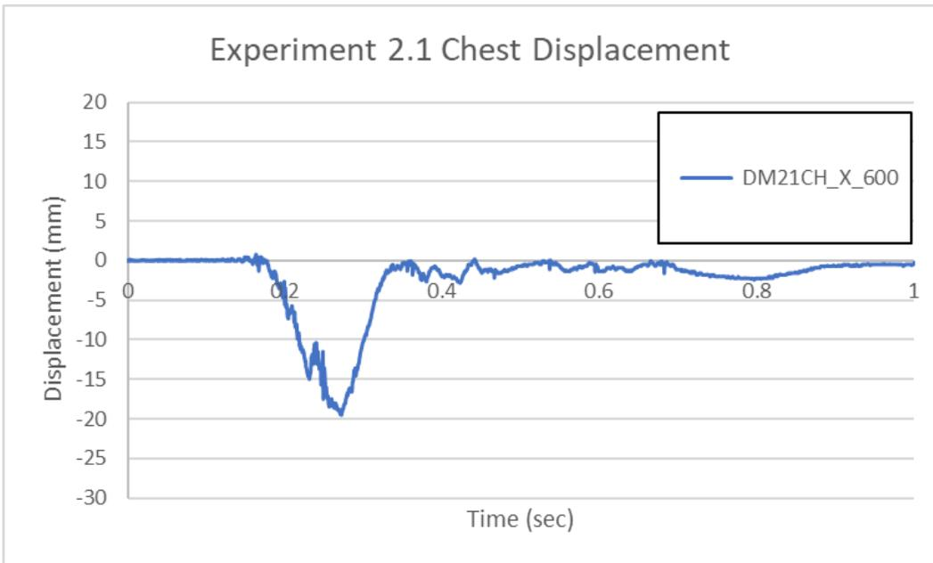
**Figure 93. Occupant Protection Experiment 2.1 Chest Displacement Data**
