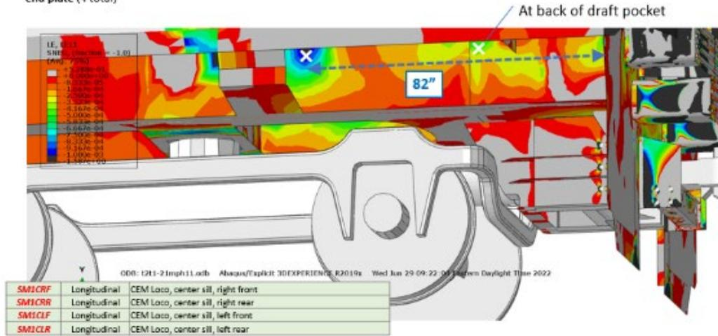
**Figure 17. Strain Gage Locations on CEM Locomotive Center Sill**
