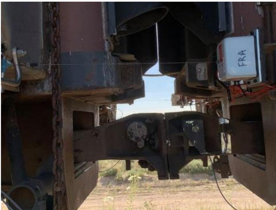
**Figure 28. Second M1 Passenger Car Coupler String Potentiometers**
