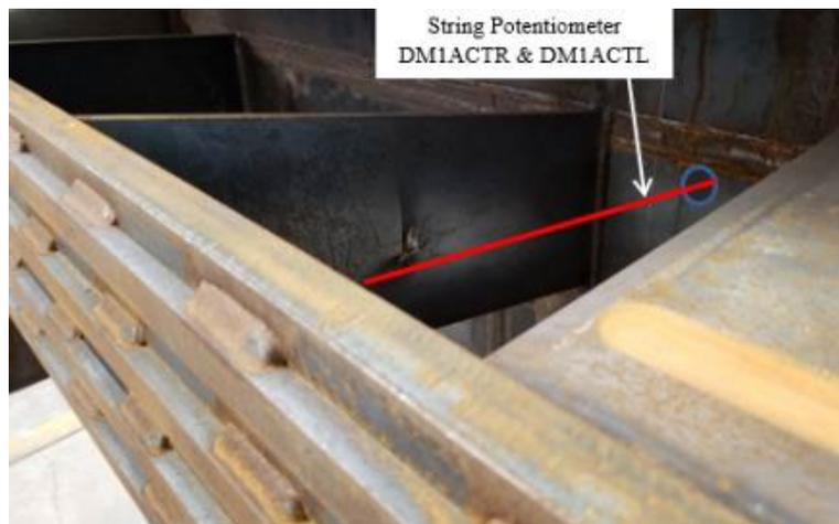
**Figure 9. CEM Locomotive Top Anti-climber String Potentiometers**
