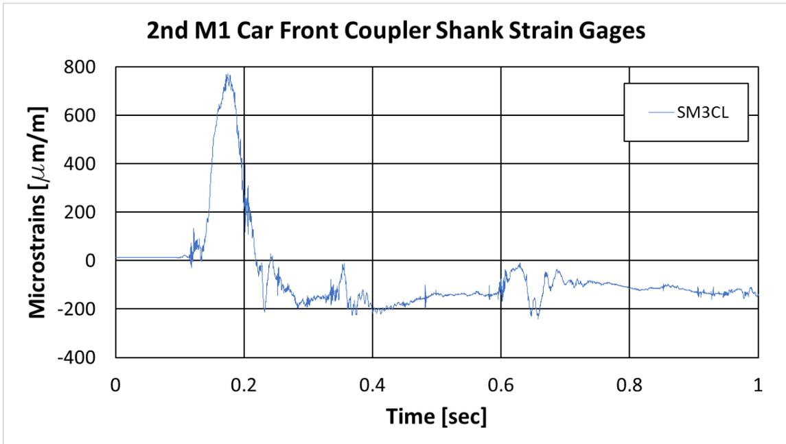
**Figure 59. 2nd M1 Passenger Car Front Coupler Shank Strain Results**
