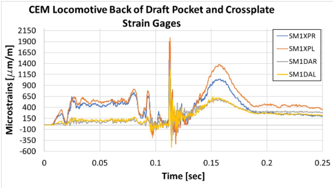
Figure 53. CEM Locomotive Back of Draft Pocket and Cross Plate Strain Results
