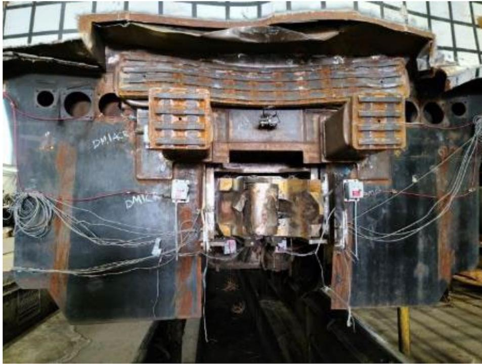
**Figure 95. Crushed Upper DAC and Partially Crushed Lower DAC Tubes**
