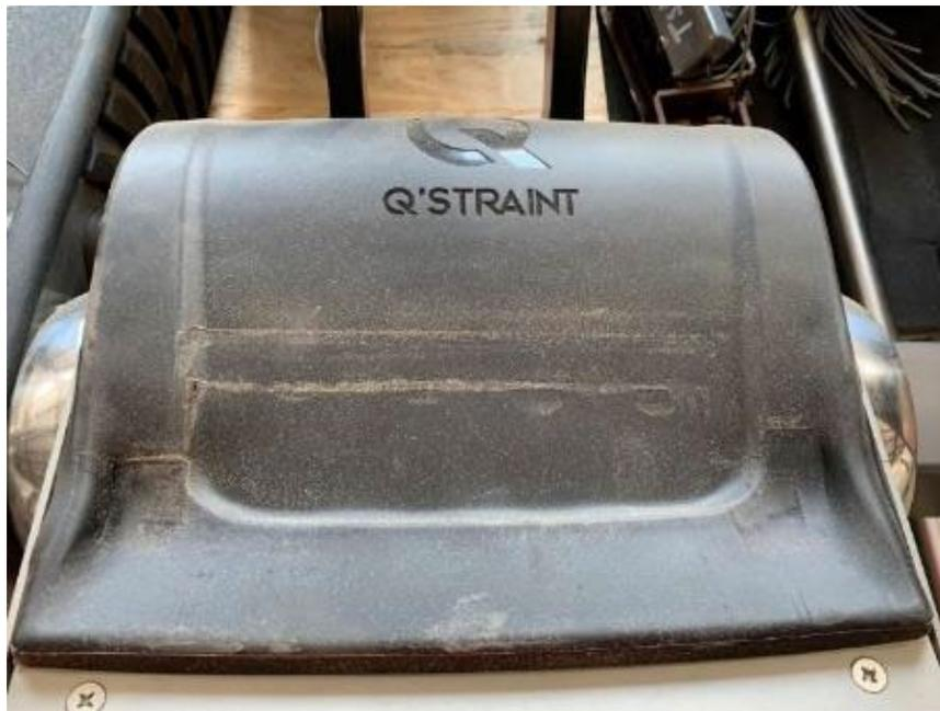
**Figure 122. Damaged Cover Plate on the Quantum Chassis**
