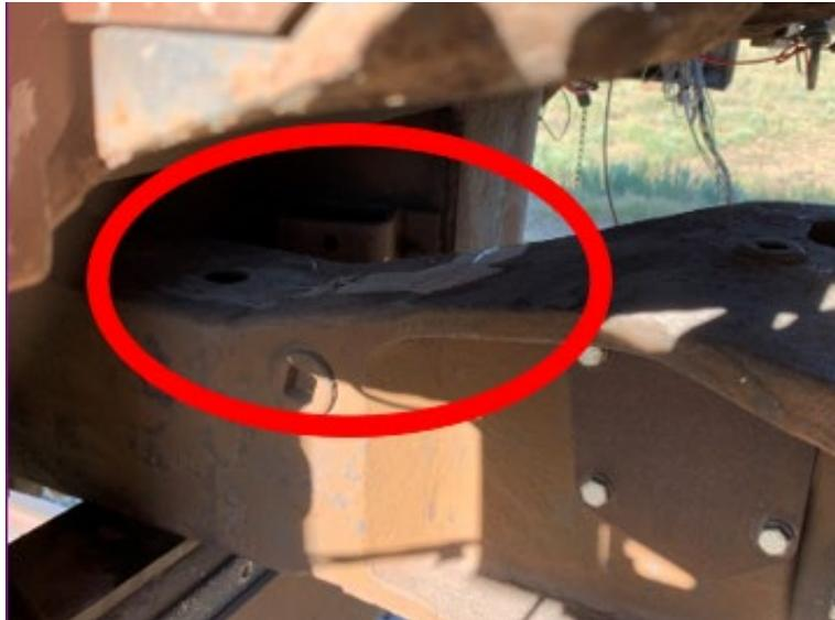
**Figure 29. Strain Gage Location on the Second M1 Passenger Car Lead Coupler**
