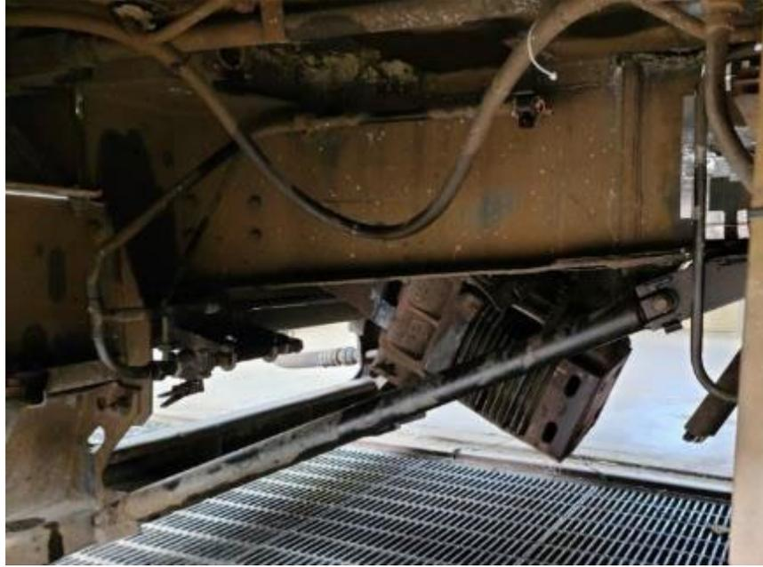
**Figure 113. Yoke from the Front Coupler on Car 8332**
