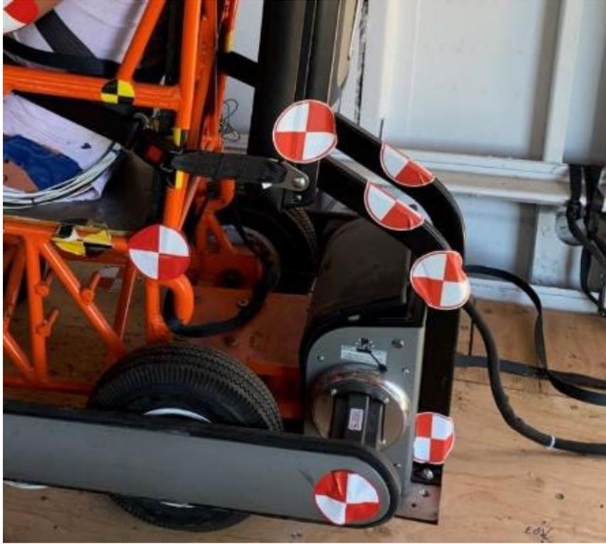
**Figure 121. Plate at Base of Surrogate Wheelchair in Contact with Quantum Chassis**
