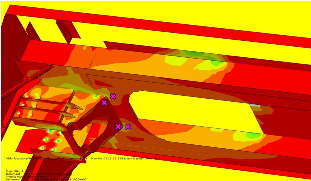
**Figure 18. Strain Gage Locations on Cross-Plate and Draft Gear Pocket Back Plate**
