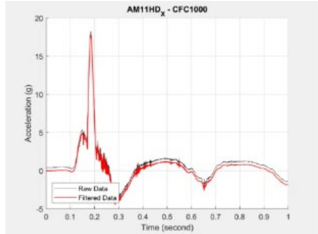
**Figure B110. AM11HD\_X Accelerometer Data**
