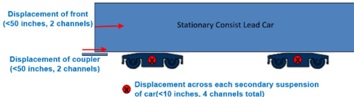
**Figure 31. Conventional F40 Locomotive String Potentiometer Locations**
