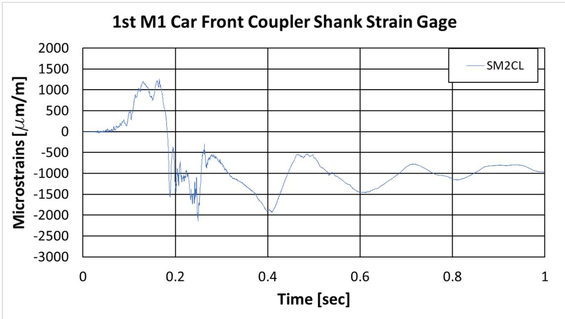
**Figure 55. First M1 Passenger Car Front Coupler Shank Strain Results**
