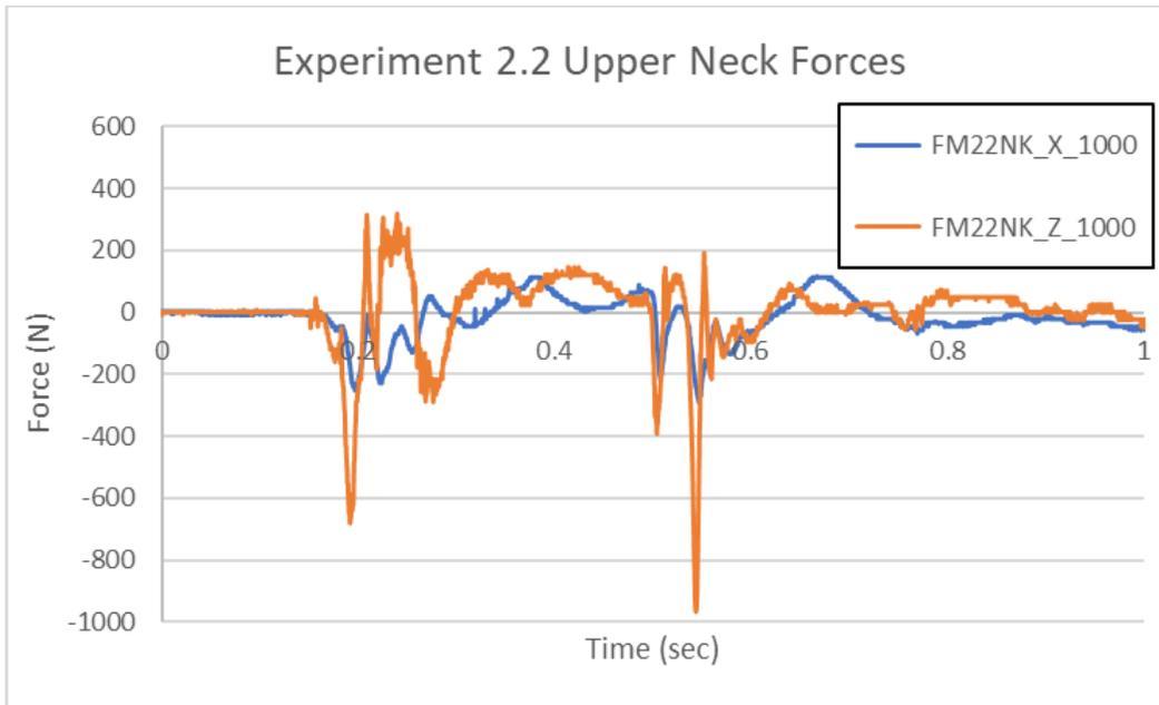
**Figure 88. Occupant Protection Experiment 2.2 Upper Neck Force Data**
