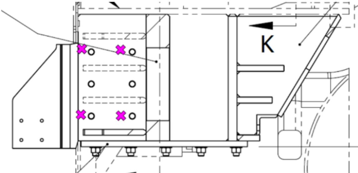
**Figure 14. Strain Gage Locations on CEM Locomotive Sliding Lug**
