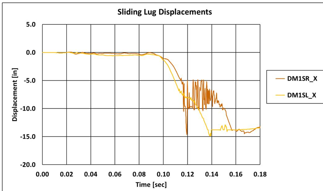
**Figure 47. Sliding Lug Displacements**
