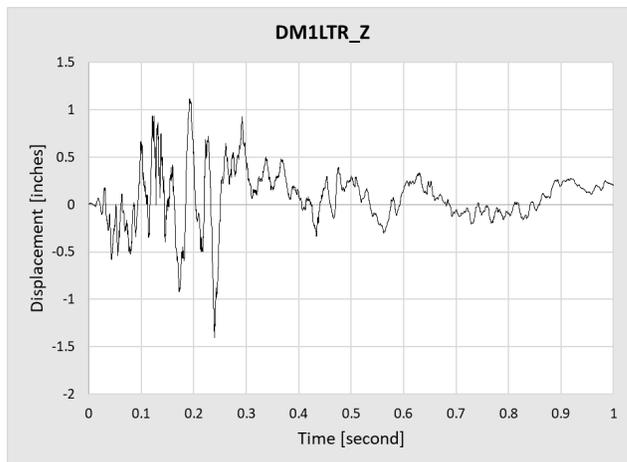
**Figure B54. DM1LTR\_Z Displacement Data**
