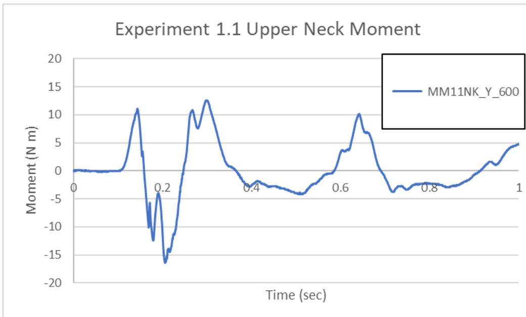
**Figure 89. Occupant Protection Experiment 1.1 Upper Neck Moment Data**
