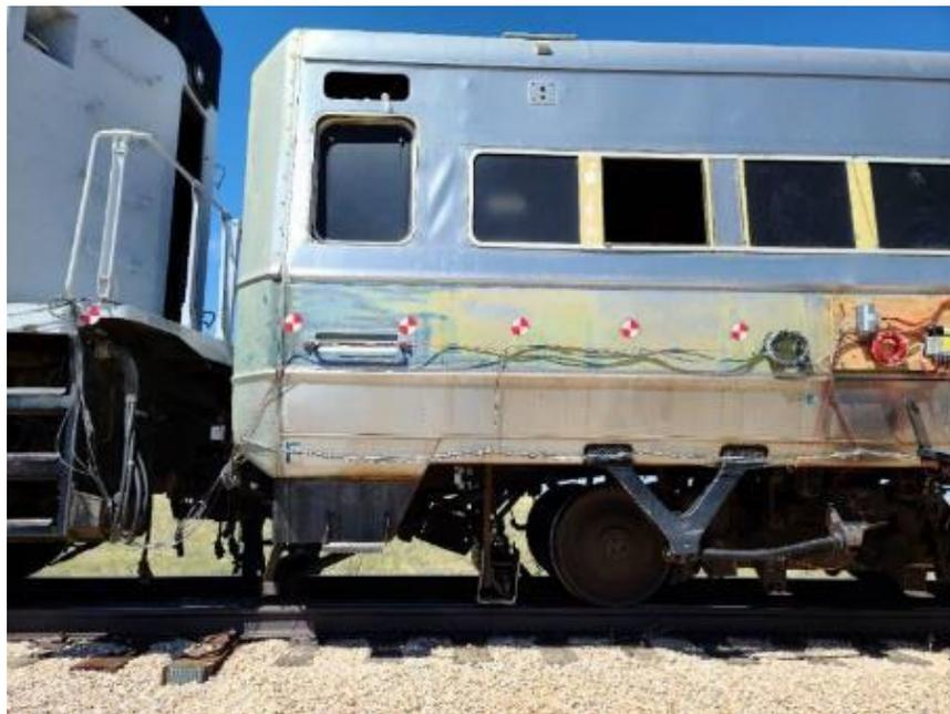
**Figure 116. Bent Traction rod at Cab End of 8332**
