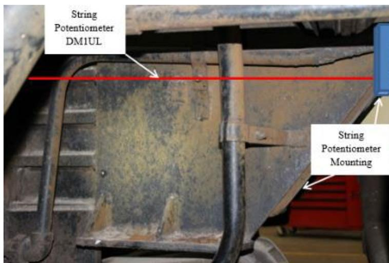
**Figure 10. CEM Locomotive Underframe String Potentiometers**
