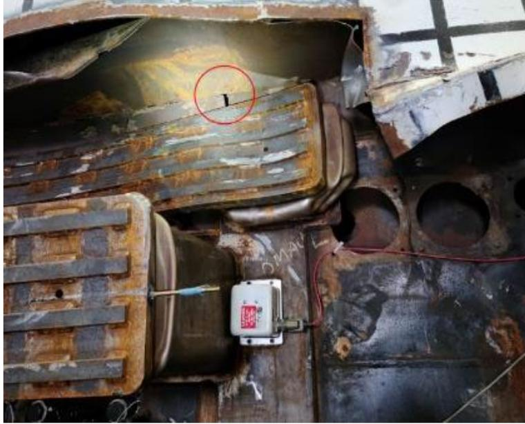
**Figure 103. Left Side of the Cracked Front Plate (Highlight in Red)**
