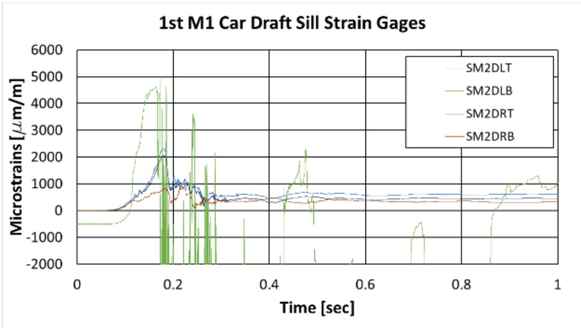
Figure 56. First M1 Passenger Car Draft Sill Strain Results
