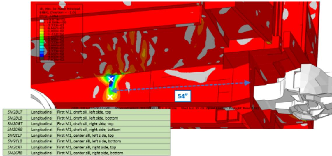
**Figure 23. Strain Gage Locations on the First M1 Passenger Car Draft Sill**
