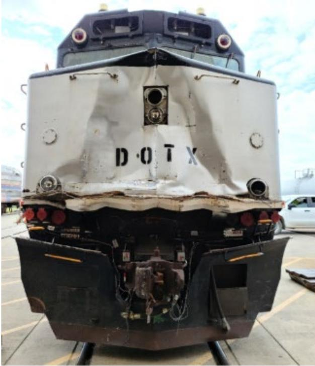
**Figure 109. Damaged Front of the Conventional Locomotive**
