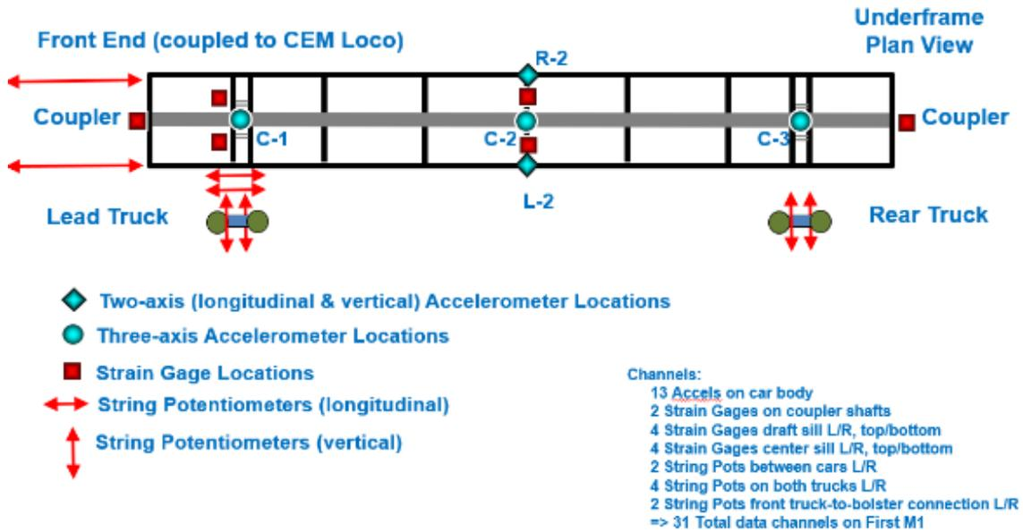
Figure 19. First M1 Passenger Car Instrumentation
