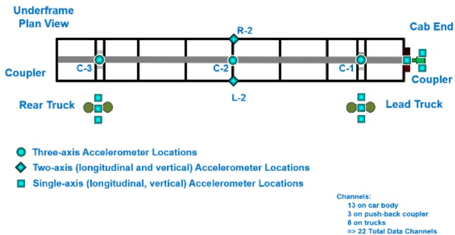
**Figure 4. Top View of Accelerometer Locations on CEM Locomotive**
