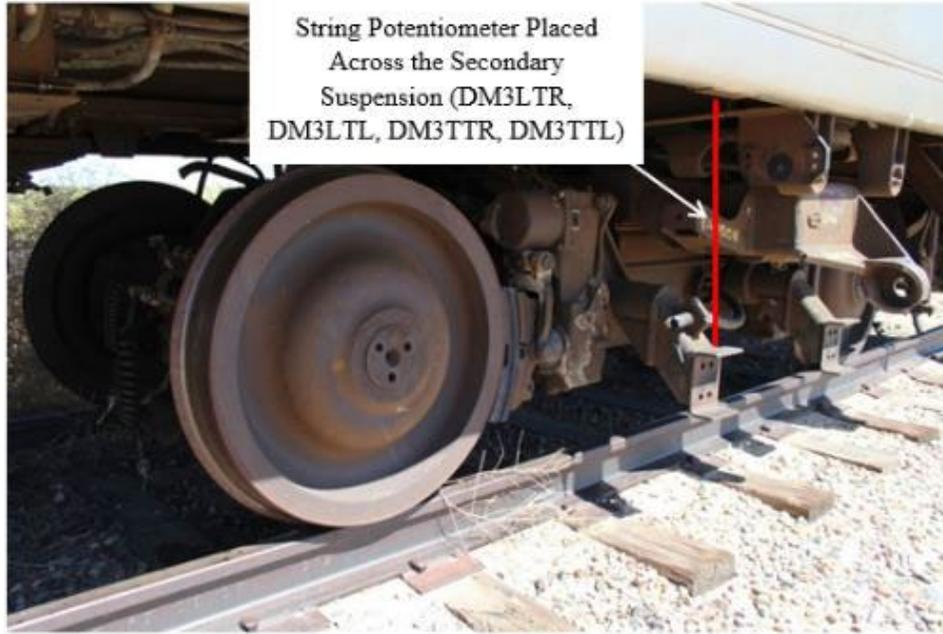
**Figure 27. Second M1 Passenger Car Truck Secondary Suspension String Potentiometer**
