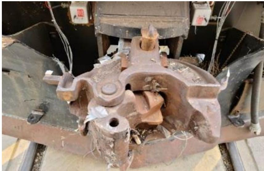
**Figure 100. Conventional Locomotive Coupler Head – After Impact**
