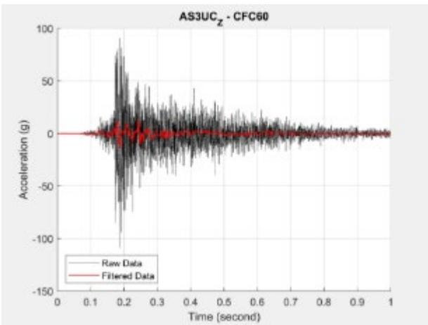
**Figure B51. AS3UC\_Z Accelerometer Data**
