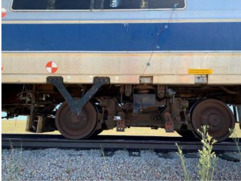
**Figure 117. Broken Traction Rod Mountings on Cab End of 8221**
