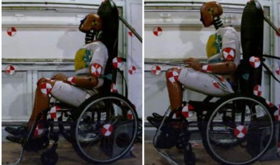
**Figure 69. Occupant Protection Experiment 1.1 Impact Movement**
