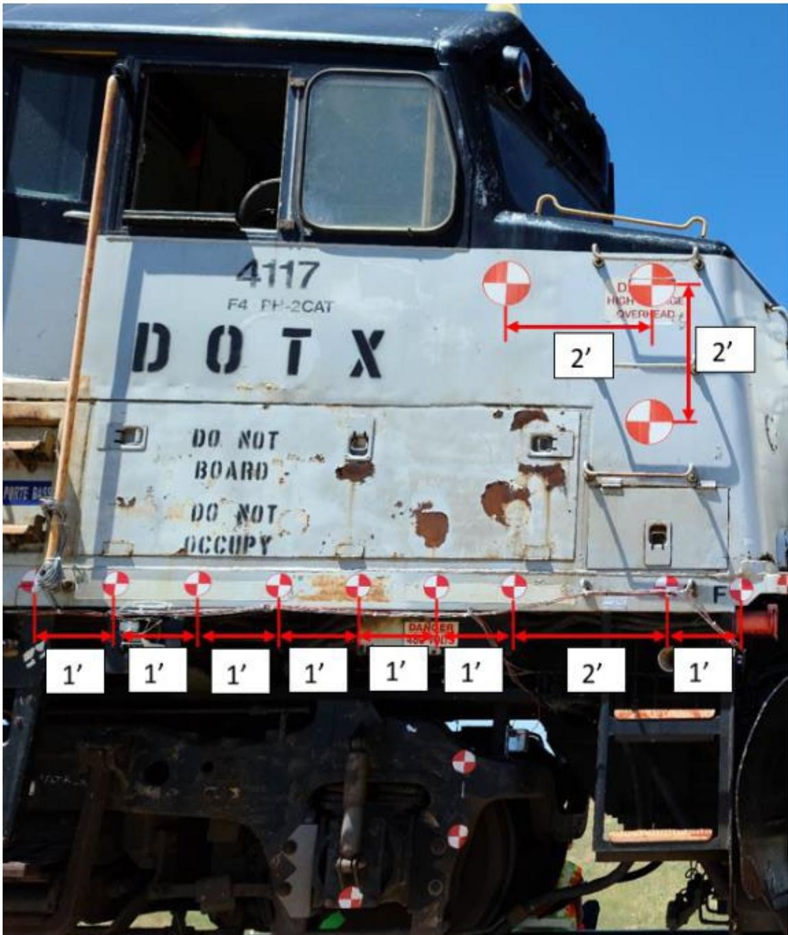
Figure A2. Target Spacing for Conventional Locomotive
