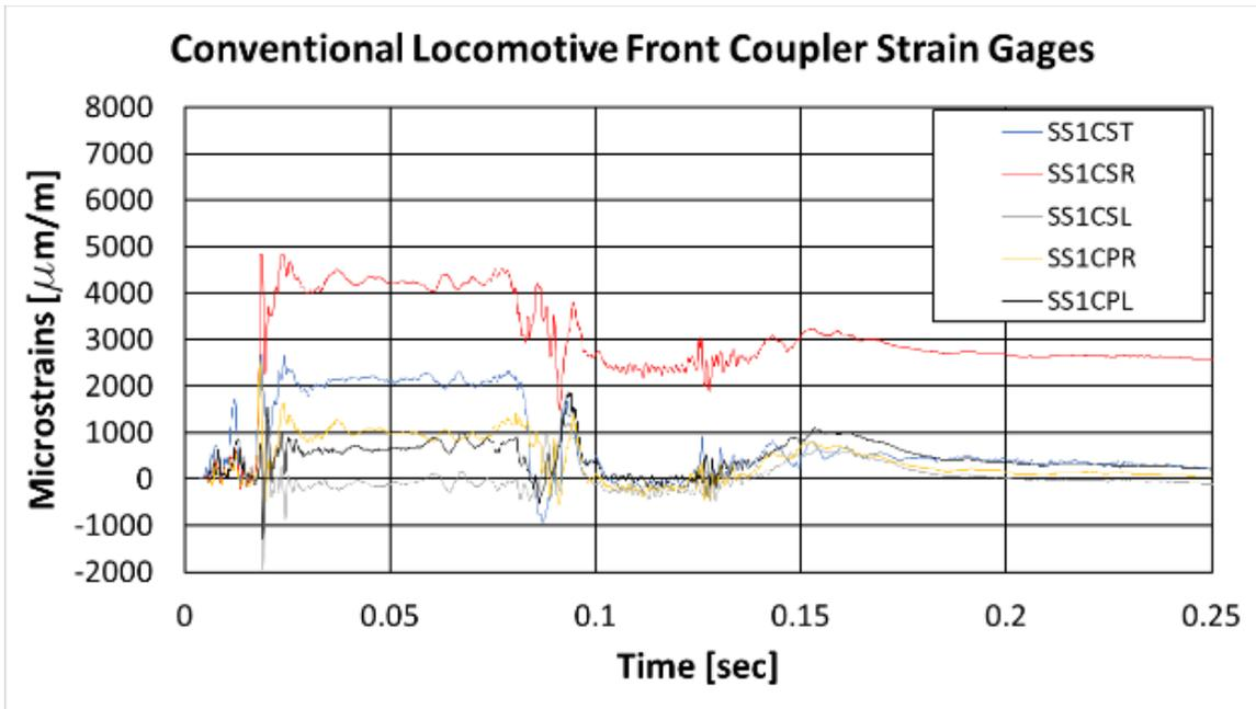
**Figure 60. Conventional Locomotive Front Coupler Shank Strain Results**
