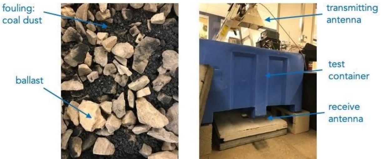
**Figure 3. Ballast with coal dust fouling (left). Test container with antennas above and below to measure signal attenuation (right).**
