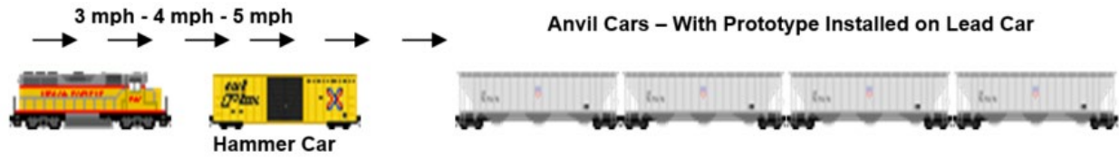
Figure 2. Impact Test Train Setup
