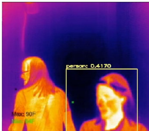
Figure 5. Thermal camera data processed using Darknet architecture
