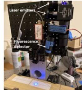
Optical sensing system in Field testing
