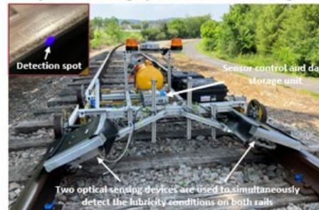
Rail-cart-mounted grease detection system
