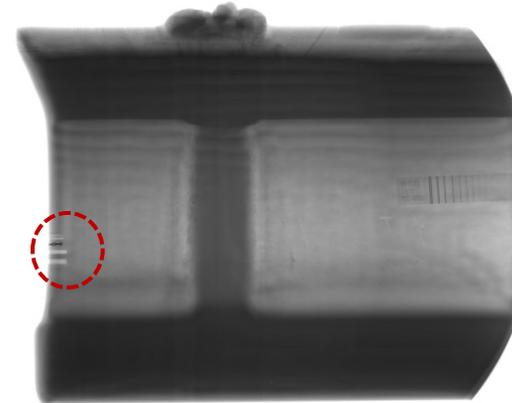
Processed radiograph a flash-butt with a zoomed-in view (left) highlighting the machined holes to represent flaws with diameters of 0.5 mm (tungsten impurity), 1 mm, 1.5 mm, 2 mm, 2.5 mm, and 3 mm (top to bottom)
