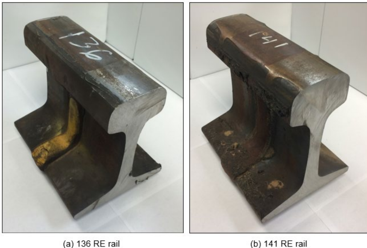
Figure 58. Photographs of thermite welded rails.
