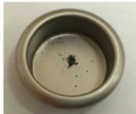
(b) Fragments of oxide layer
