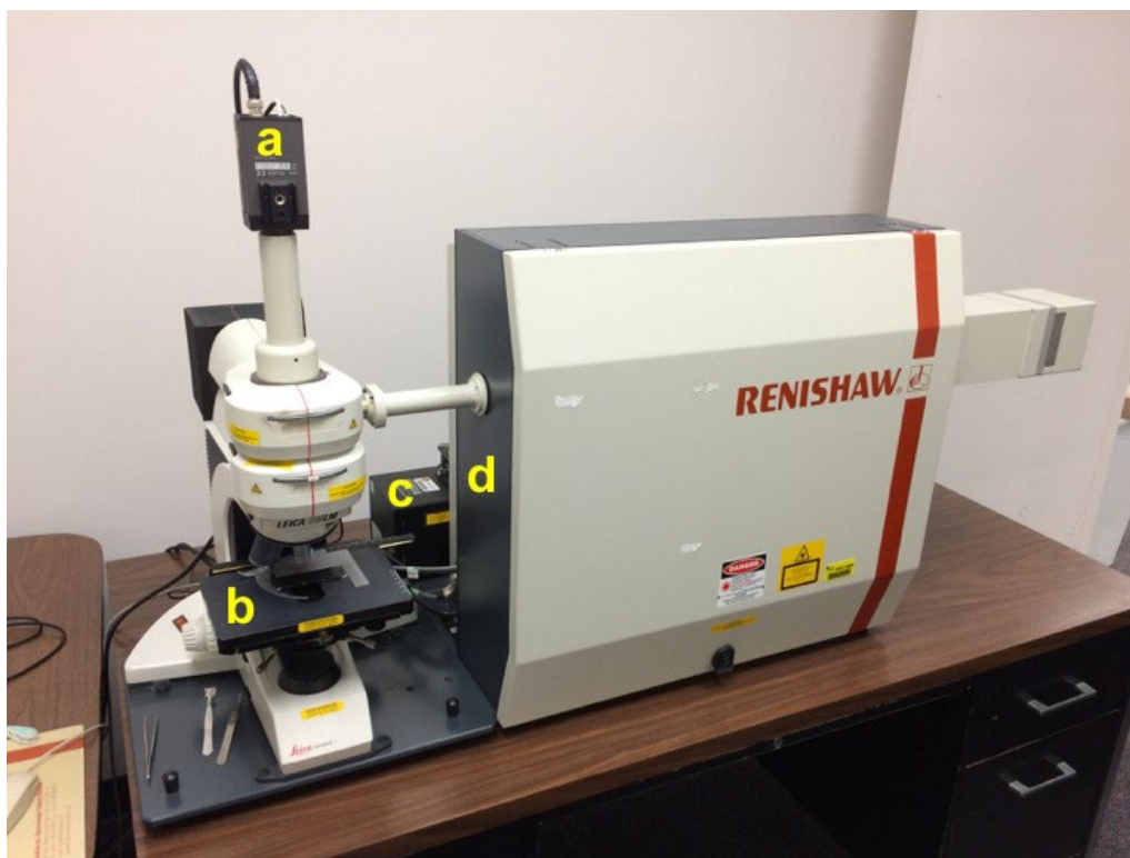
Figure 8. Bench-Top Raman Spectroscopy System at UCF (a) CCD Camera; (b) Microscope; (c) 514 nm Laser (Green Laser); (d) Raman Spectrometer
