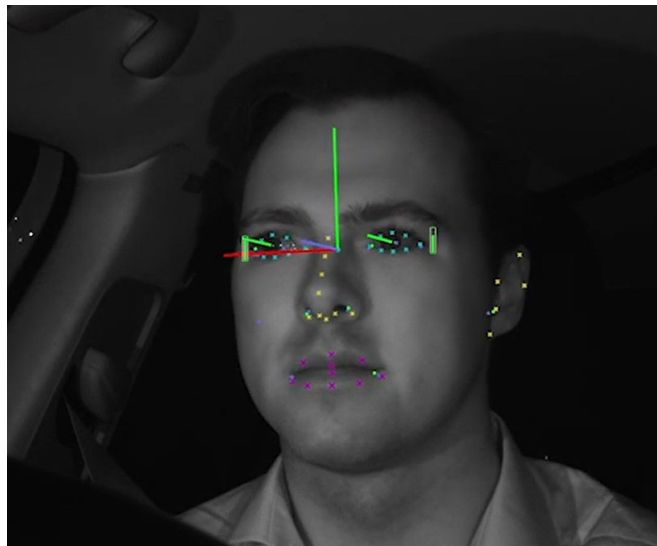
Figure 4. Facial features and tracking measures used by the SmartEye system
