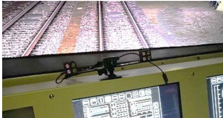
Figure 3. SmartEye DSM system set up in the CTIL simulator
