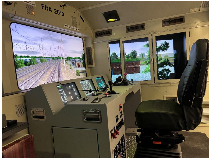
Figure 1. Interior of CTIL Simulator, modified Siemens ACS 64 console
