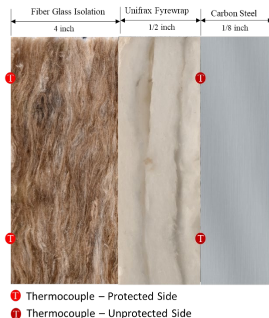
Figure 11. Thermal protection system thermocouple locations
