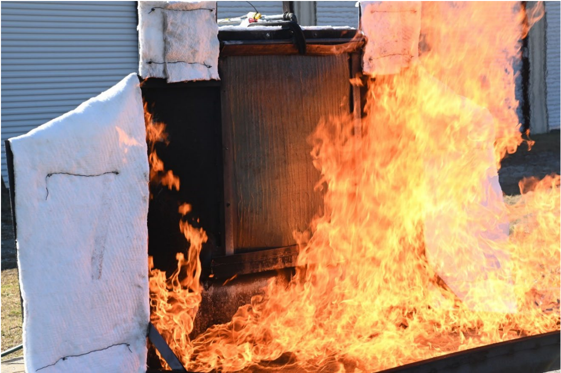
Pool fire test – cooling water
