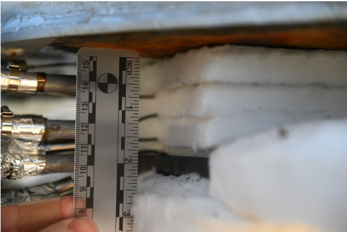
Insulation layer detail in thermal conductivity test
