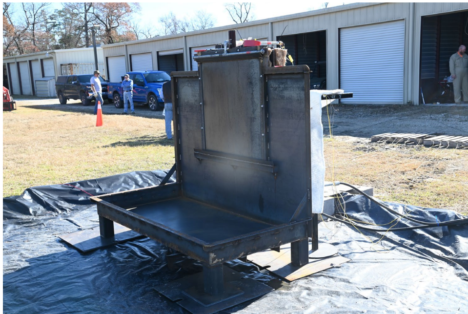
Pool fire test apparatus – front
