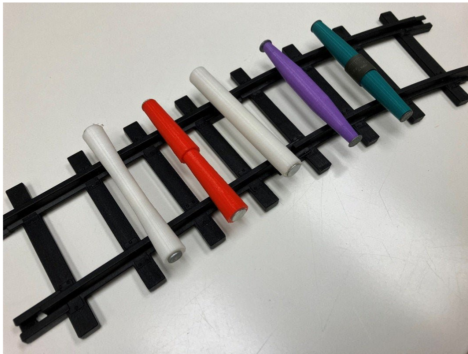
Figure 7. 3D Printed Wheelset Models for Wheel-Rail Dynamics Activity
